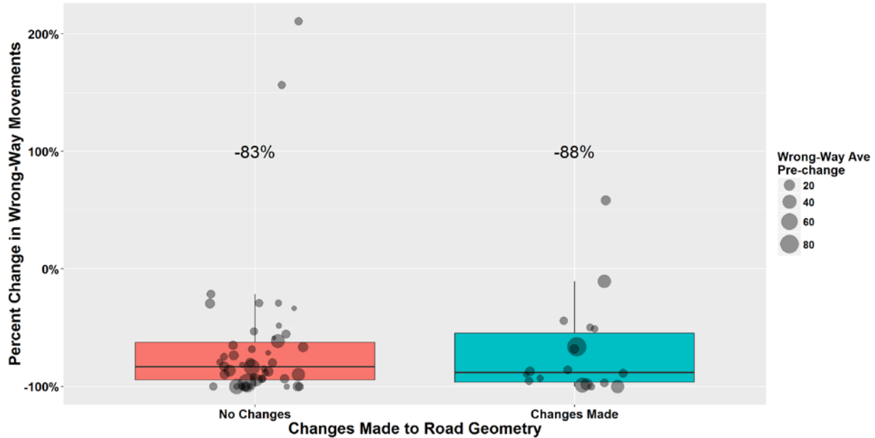
Figure 21. Percent change in wrong-way movements by whether or not geometric design changes were implemented at a ramp. Geometric changes were the least common type of change made, likely because this is likely the most expensive types of change made.
