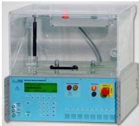
Figure 3.6. MIG0606 Surge Generator with TC-MIG24ED Cabinet
