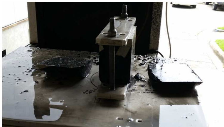
Figure 4 —Trimmed Specimen (Side view, specimen still in clamps, specimen sides have been cut away on each side)
