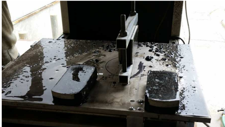
Figure 6 —Trimmed Specimen (Side view, specimen still in clamps, specimen top and bottom have been cut away on each side)
