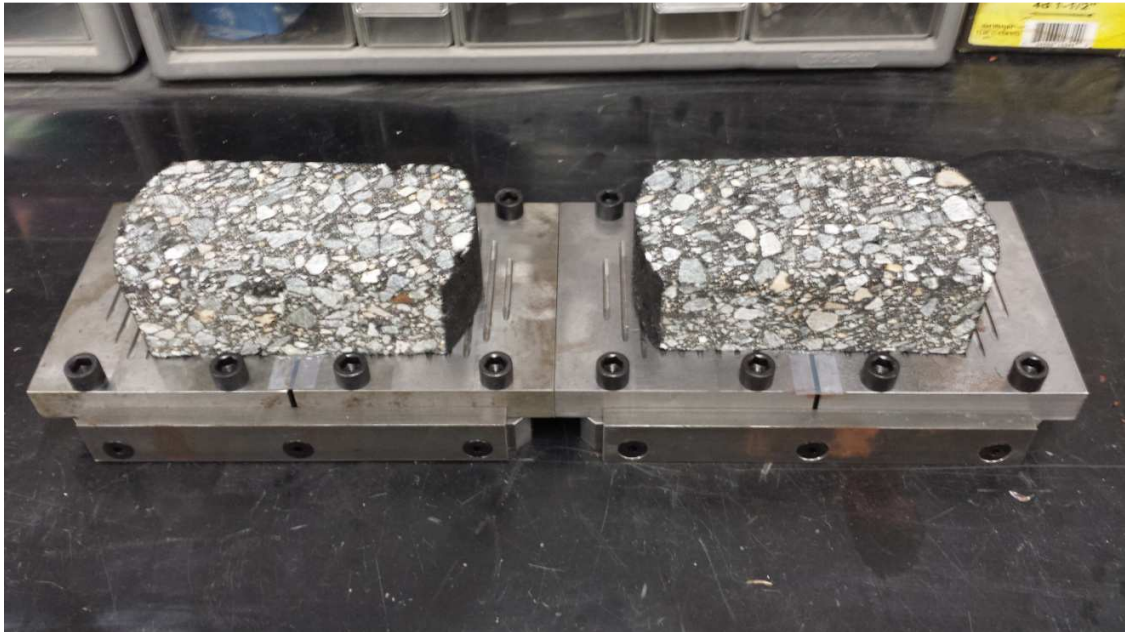
Figure 3.6. Samples on the Specimen Plates and the Setup Plate after Curing of Epoxy
