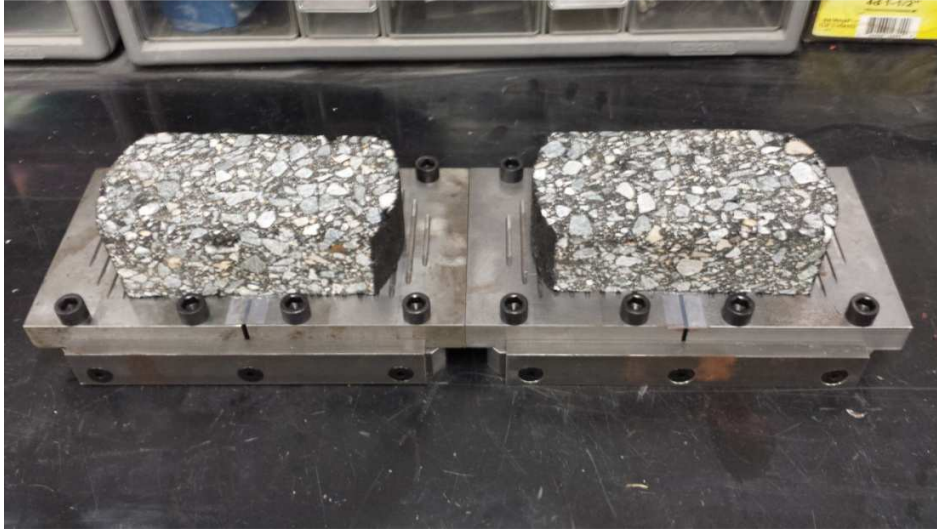
a) View from the side: The mounting jigs are visible under the base plates, and the clear adhesive tape is visible over the gap between the base plates.
