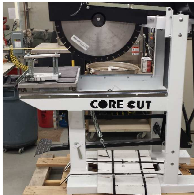
Figure 3.4. Diamond Product® CC800M Single Blade Saw with Specimen Cutting Jig
