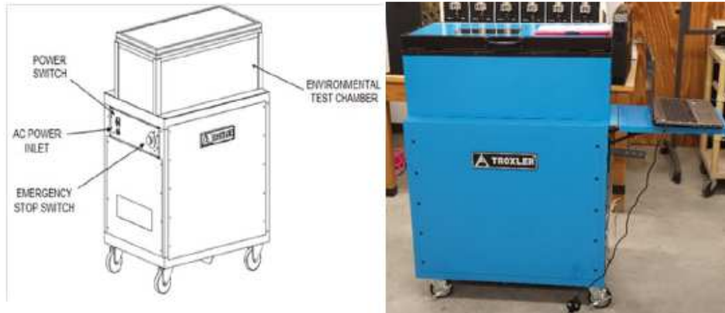
Figure 3.7. Troxler Model 5950 Overlay Tester
