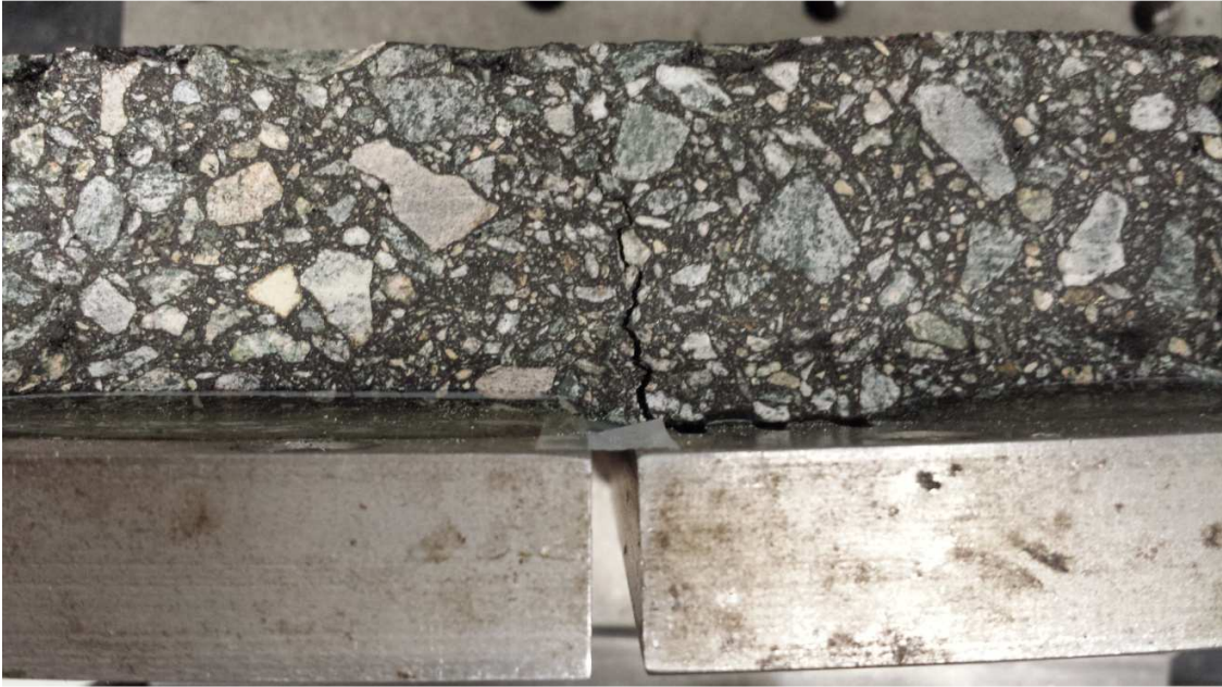
Figure 4.2. Representative Specimen after Cracking
