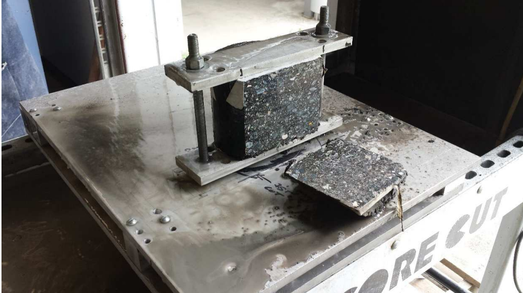
Figure B-9. First Side Cutting
