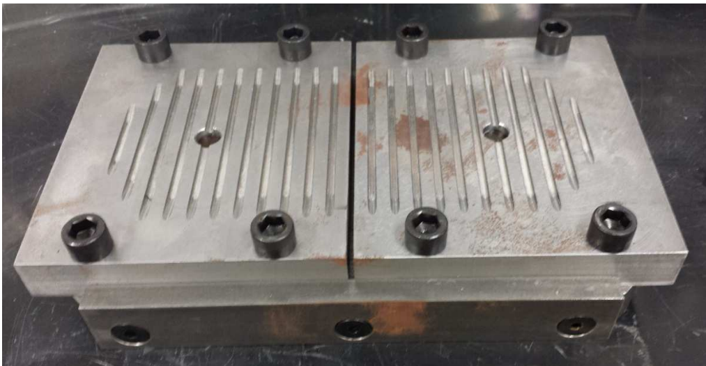
Figure 3.5. Overlay Tester Setup Plate and Specimen Plates
