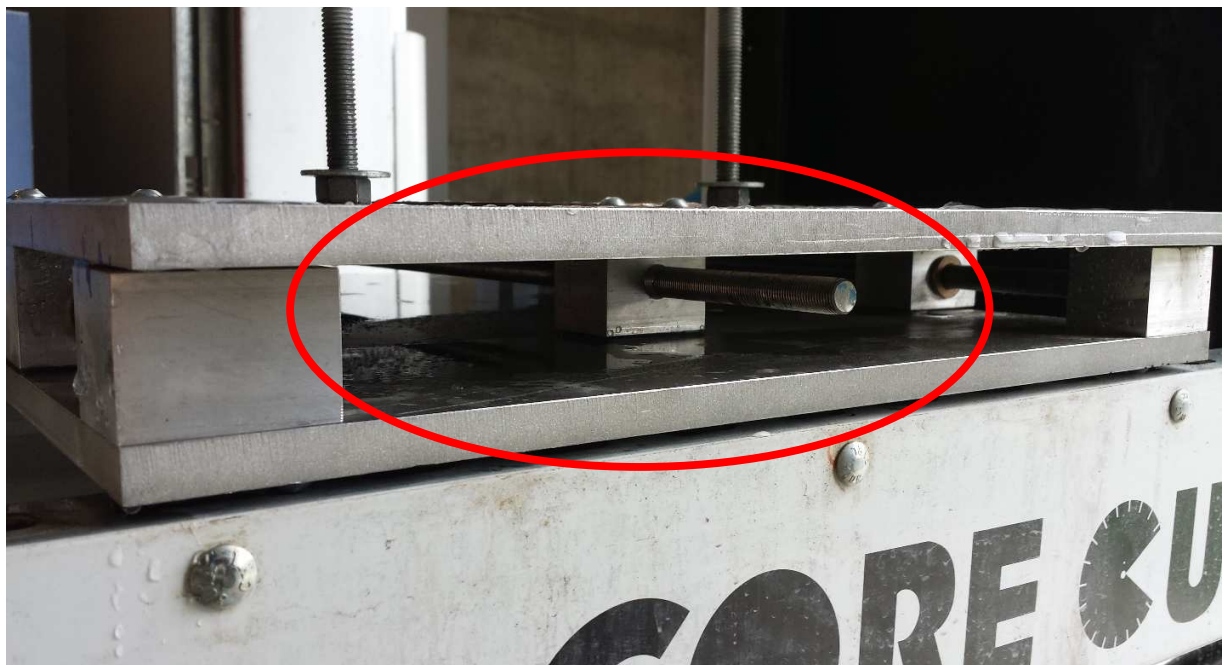
Figure 3.13. Threaded Rod for Displacement Control
