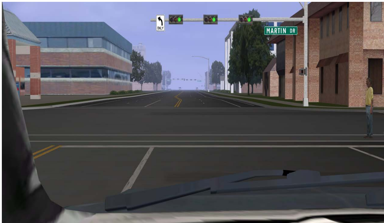
Figure 31. Driving simulator tile with standard crosswalk.
