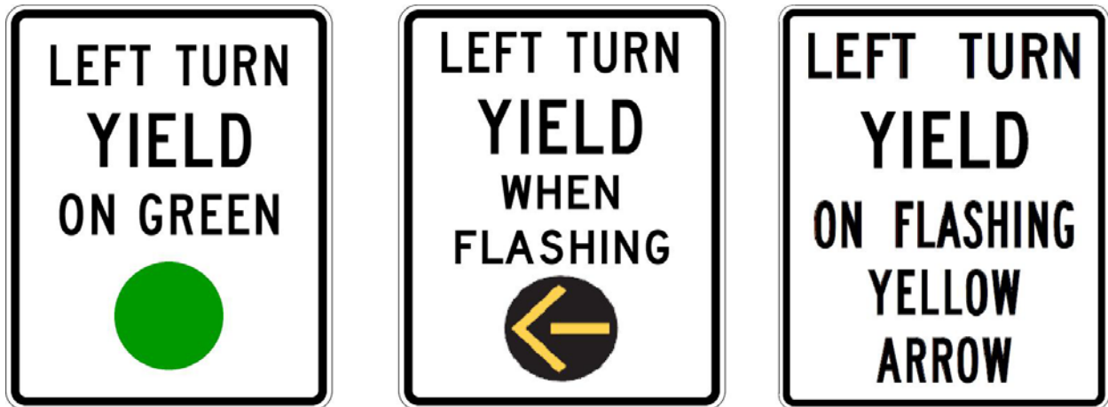
Figure 41. Supplemental signs used with PPLT signals. R10-12 (left), modified R10-12 (center), and R10-X12 (right).
