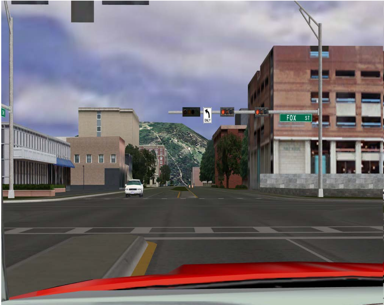
Figure 59. Sample image of an intersection with a FYA left-turn signal. At this point in the trial, the FYA signal would be displayed. In the image above, the signal is in the off phase of the flash. The oncoming vehicle is approximately 125 ft away and approaching at a speed of 50 mph.
