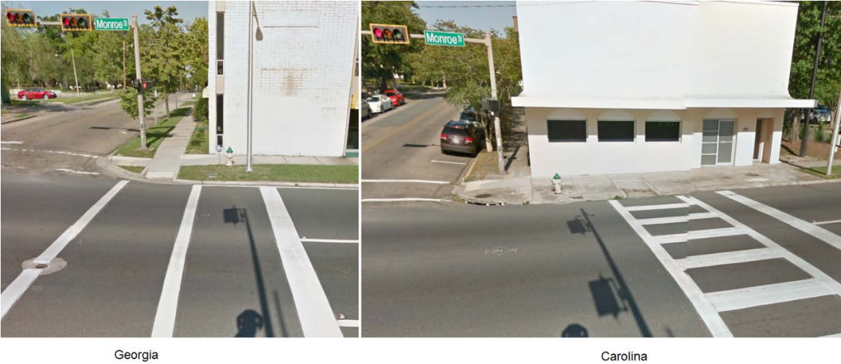
Figure 22. Comparison of crosswalk placement relative to the curb at Georgia and Carolina.
