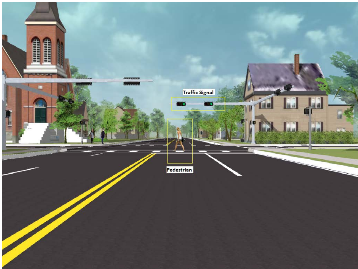
Figure 13. Interest areas used for the pedestrian detection task. This example shows the intersection from a simulated distance of 100 ft.
