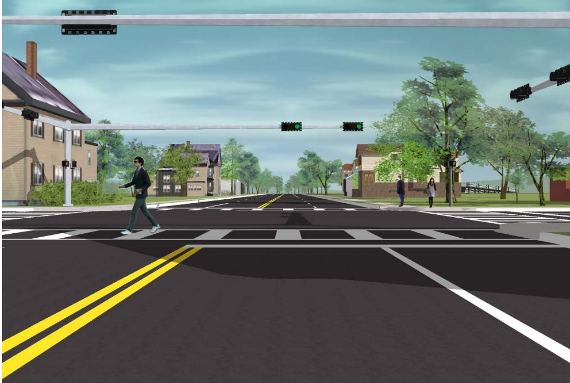
Figure 5. Example of a special emphasis marked crosswalk marking at 50 ft with a pedestrian crossing (left).
