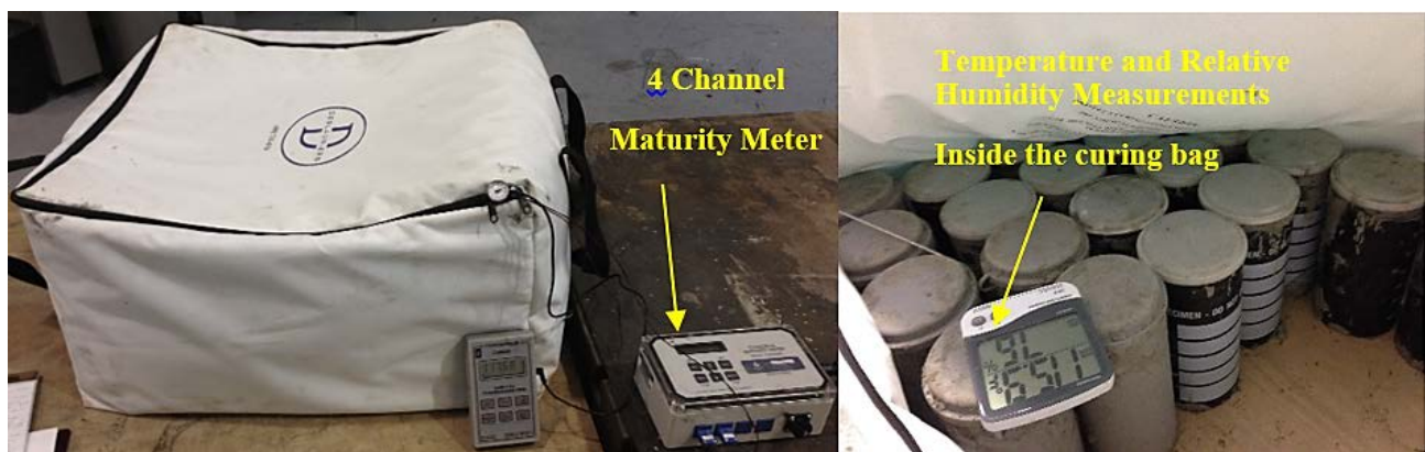
Figure 7.24: Curing bag with temperature monitoring devices
