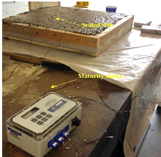
Figure 7.25: Instrumented small-scaled slab
