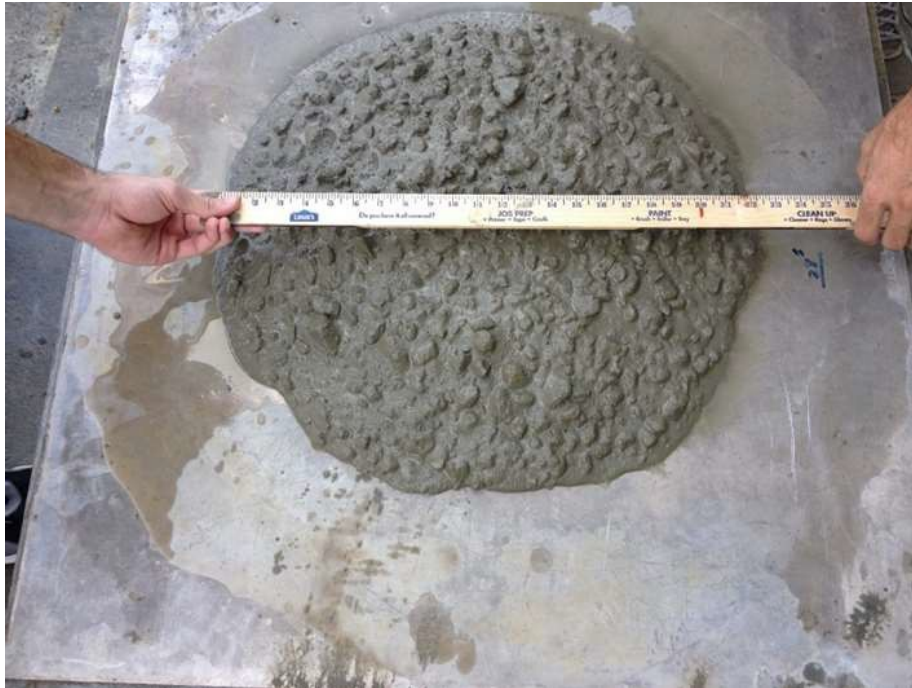
Figure 6.20: Slump flow test
