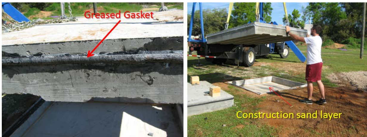
Figure 4.1: Model precast panels (6' x 6' x 8'') used in field testing
