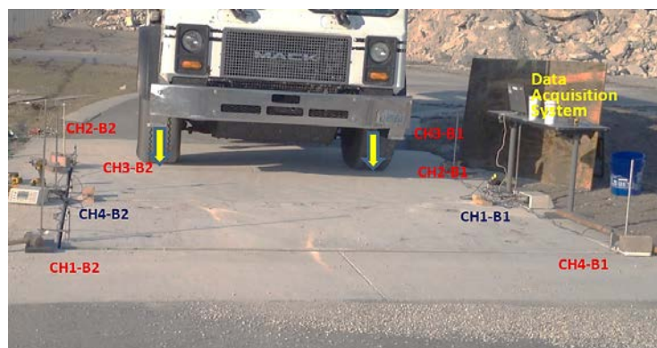
Figure 7.4: Configuration of LVDTs and wheel loads
