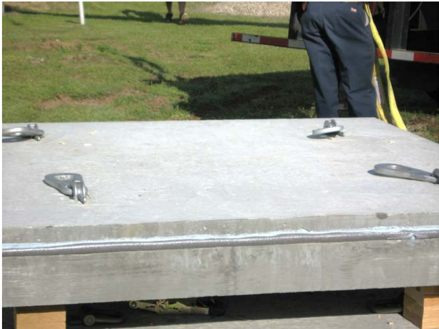
Figure 4.8: One-inch diameter backer rod inserted in the recess along the edge of model panel
