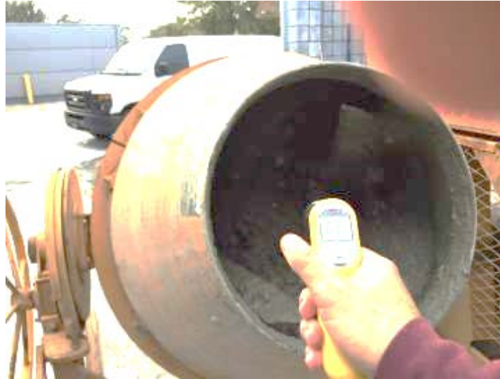
Figure 6.19: Temperature measurement of SCC mix
