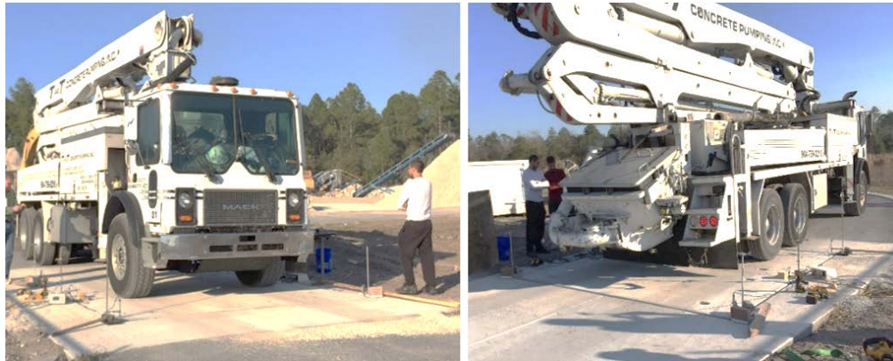
Figure 6.17: Front and rear view of the truck used in load testing of precast panels
