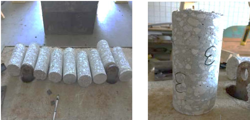
Figure 6.27: Core samples from the replacement slab – no sign of any segregation
