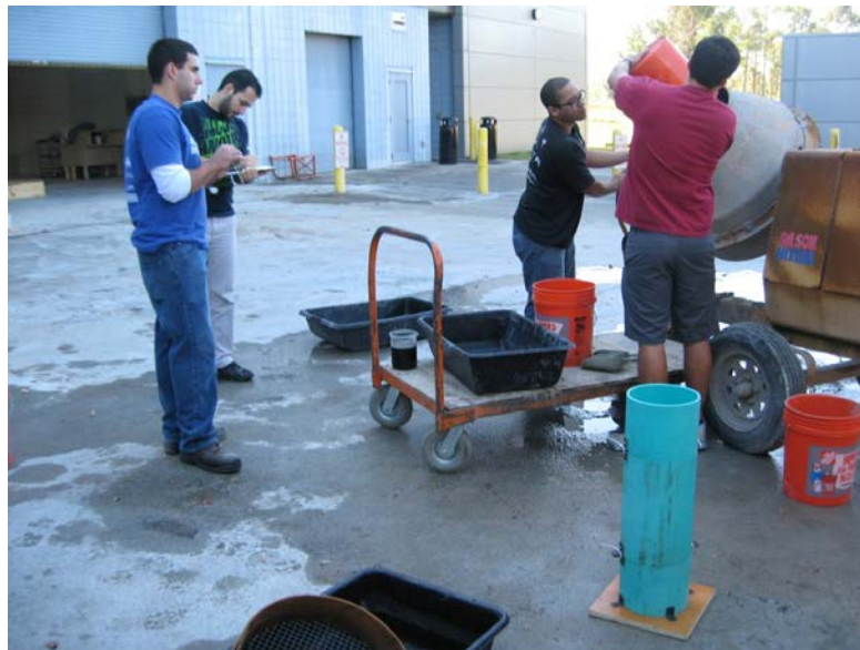
Figure 5.1: Batching of a trial mix at Civil Engineering Concrete Lab
