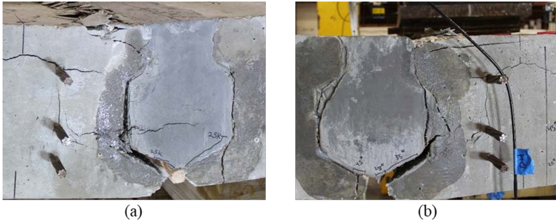
Figure D.52: 12A2-1: (a) failed specimen and (b) east side joint face showing similar rupture pattern with less amount of cracks
