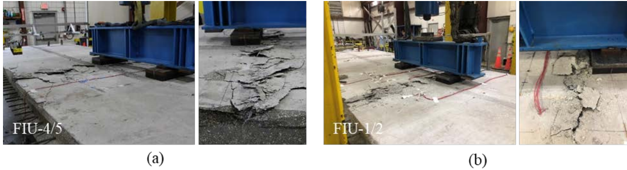
Figure 7.131: Crushing of FIU-5 and FIU-4 concrete at failure for Load Configuration 2-1: (a) overview and (b) crushing of UHPC in joint
