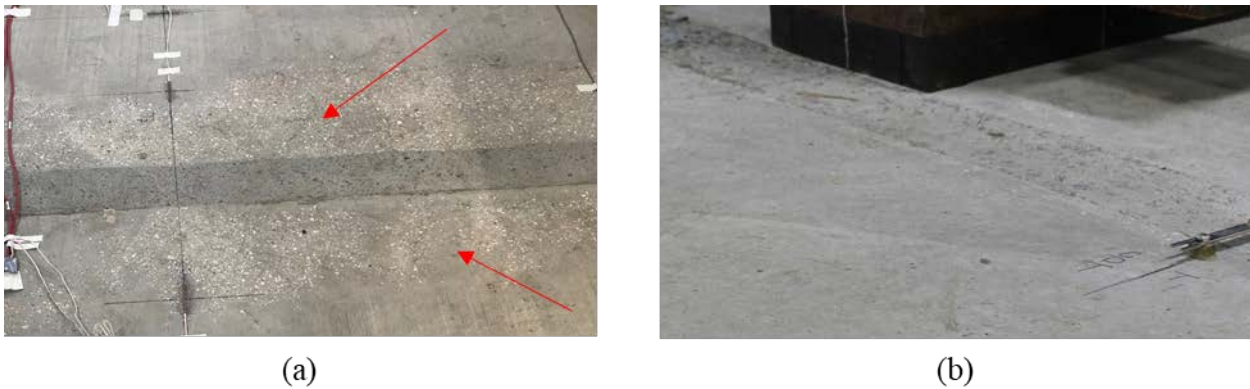
Figure 7.17: UHPC grinded surface: (a) surface finish after two days using gas grinder (showing precast abrasion), and (b) surface finish after one day using electric grinder
