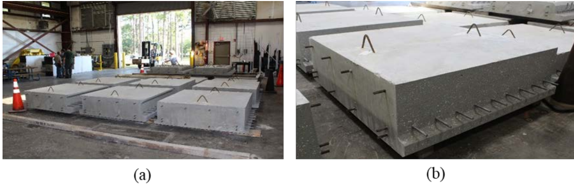
Figure 5.7: (a) Delivery of all slab-beam specimens, (b) beam showing strands, transverse reinforcement and lifting hooks (18-inch FDOT 1 shown)
