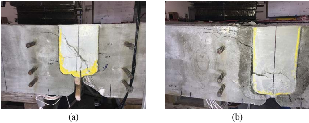
Figure 5.64: Cracking at failure for (a) 12F1-1 and (b) 12F2-1
