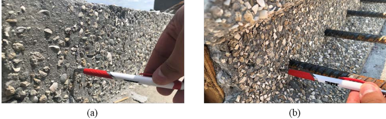
Figure 7.16: Master Finish HV retarder degrees of penetration: (a) light and (b) medium light
