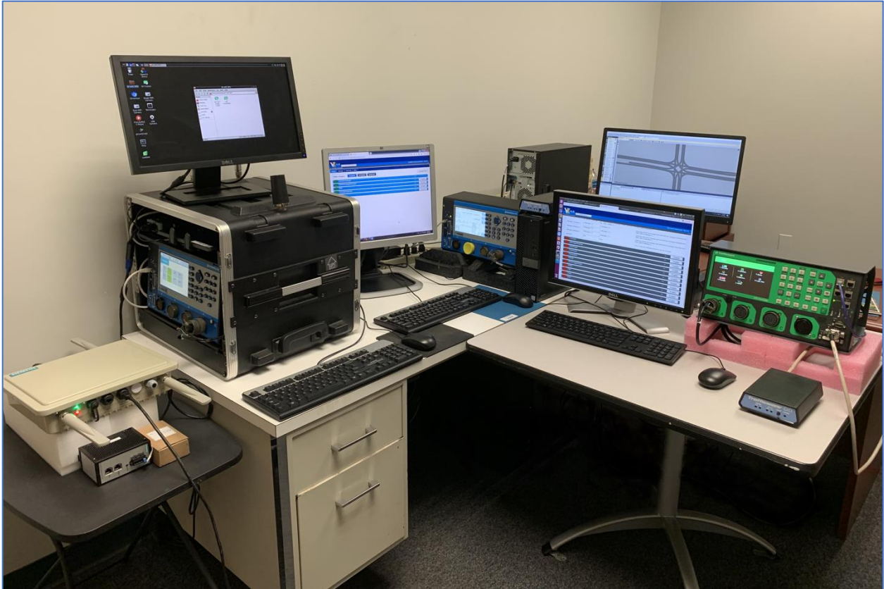
Figure 5-11 Connected Vehicle-to Infrastructure Applications Testing Environment
