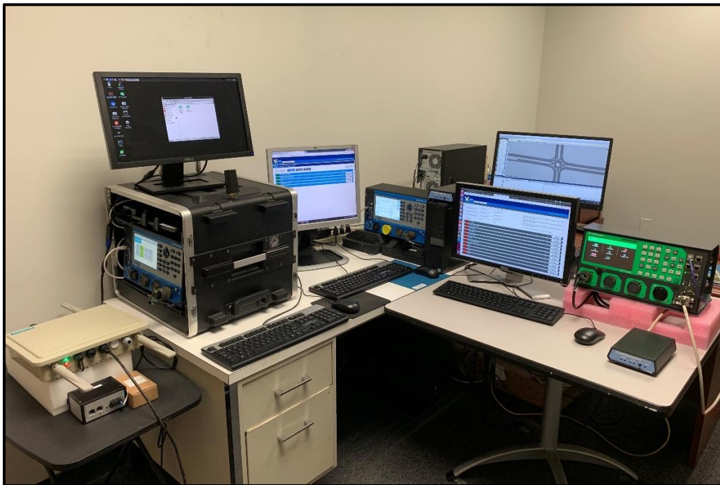
b) Hardware-in-the-loop Simulation platform Figure 7-2 (a-b) SILS and HILS platforms
