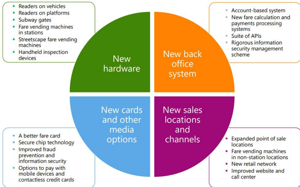
Figure 42. Components of the New System
