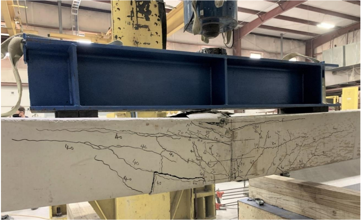
Figure 118: Crack propagation and failure mode of Specimen 10
