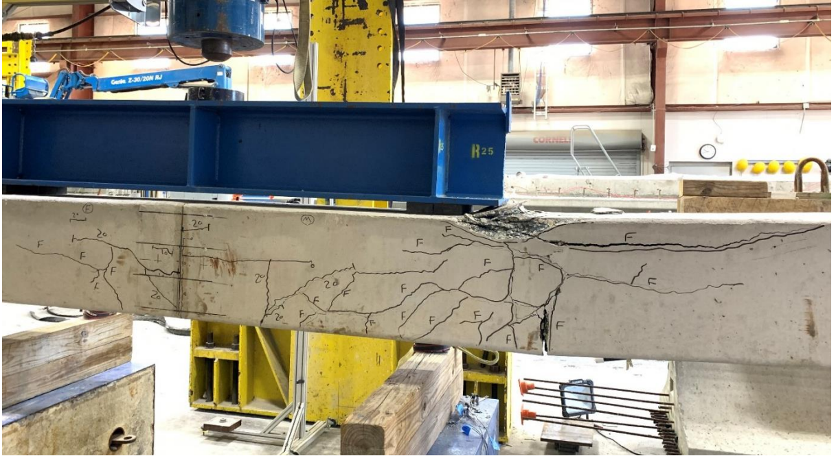
Figure 98: Crack propagation and failure mode of Specimen 6
