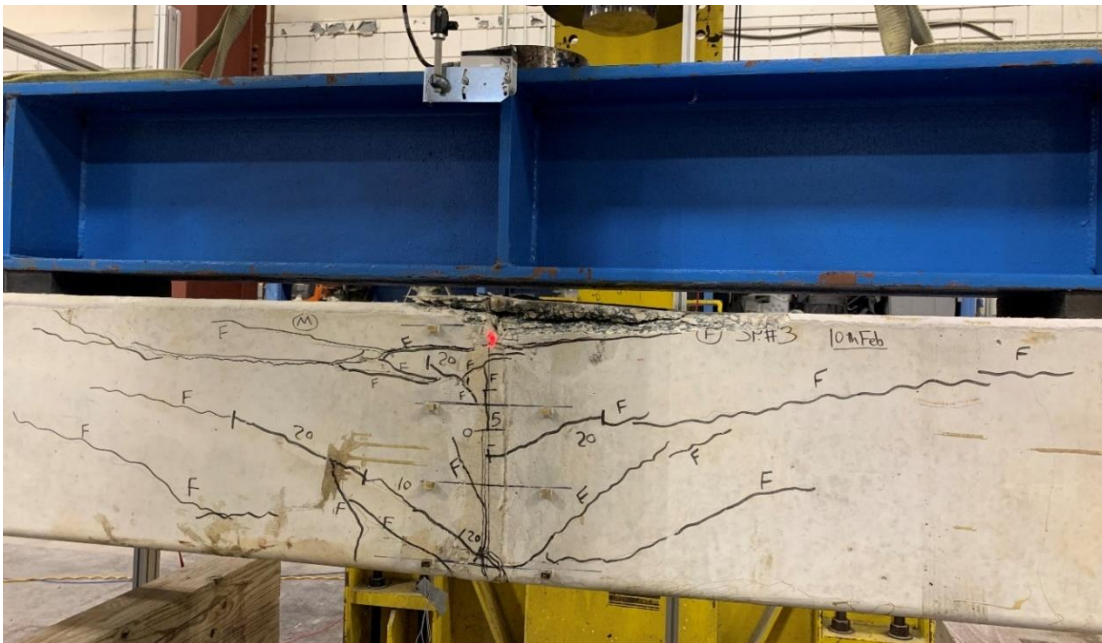
Figure 83: Crack propagation and failure mode of Specimen 3
