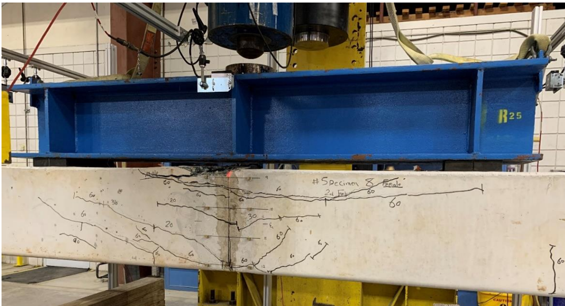
Figure 108: Crack propagation and failure mode of Specimen 8
