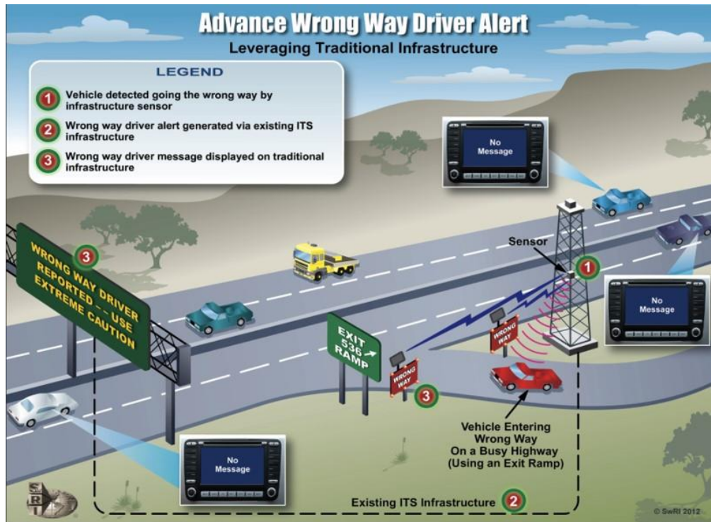
Figure 2-1: Advance Wrong-way Driver Alert – Leveraging Traditional Infrastructure (Randolph, 2014)
