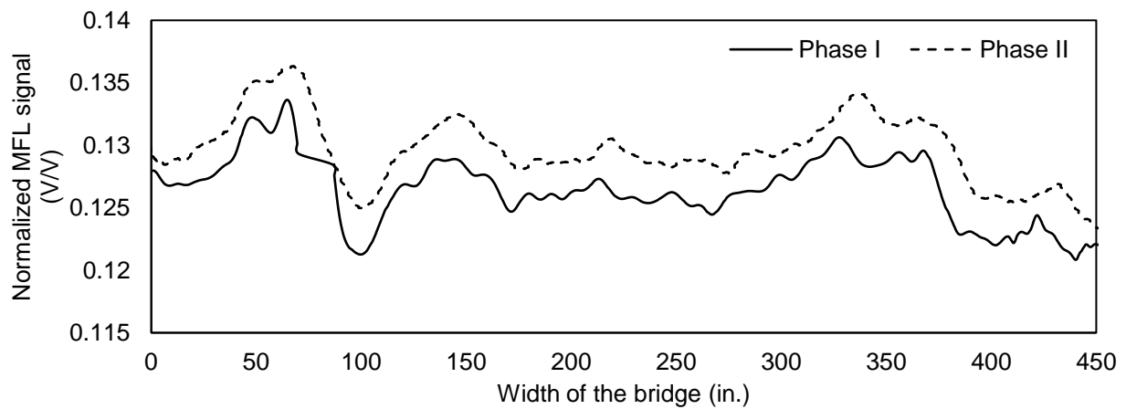
Figure B-33: Span 4, PT rod 1.
