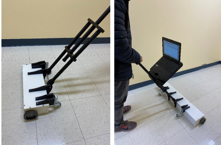
Figure 3-6: Final measurement units (a) 16 in. and, (b) 32 in. wide unit.
