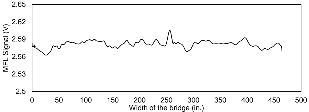
Figure 5-5: MFL signal taken between PT rods without magnetization (test S-1-0) (sensors with flux concentrators).
