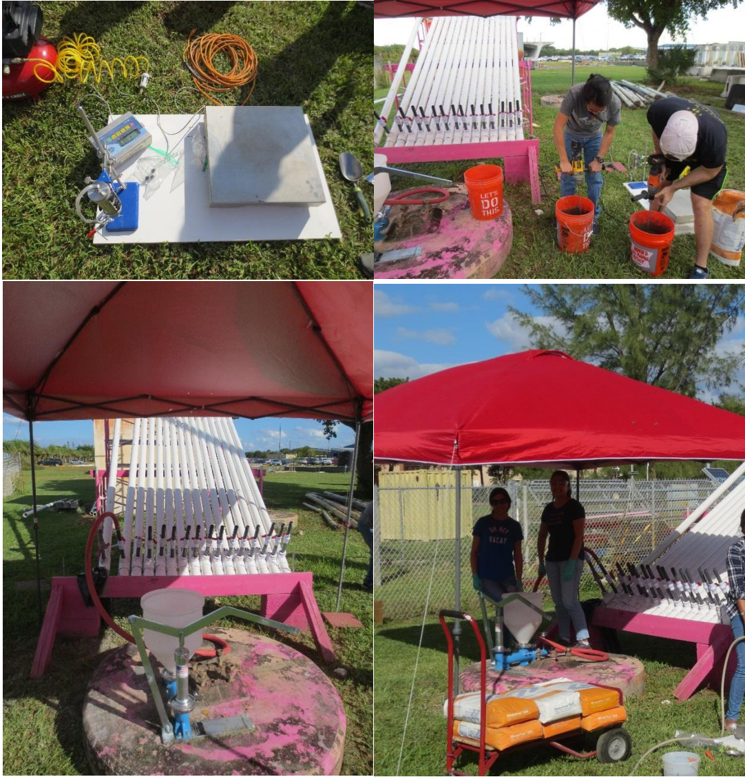
Figure 2.19. MIT Grout Mixing and Injection
