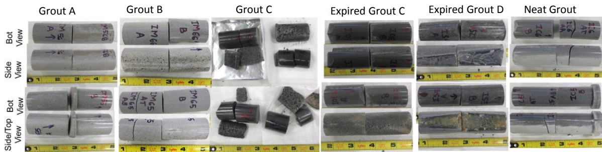
Figure A2. INT Tee-body test specimen after opening, cast with extra 10% mix water
