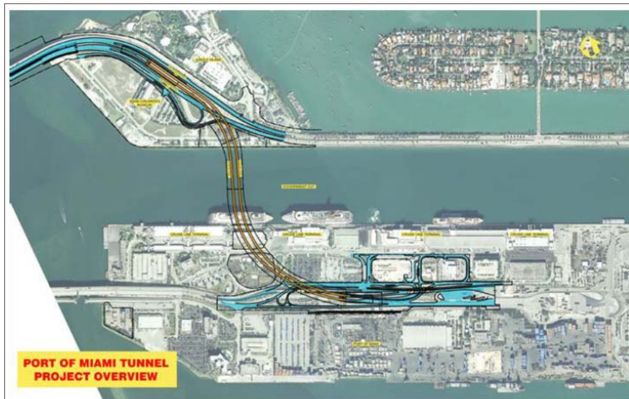
Figure 14 Port Miami Tunnel (Source: portofmiamitunnel.com)
