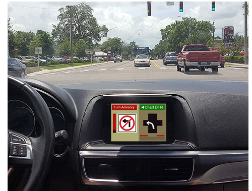
This CV is equipped with an app that talks to road infrastructure to help drivers make safer left turns.
