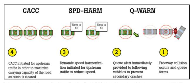
Figure 2-5 Combined Q-WARN/SPD-HARM/CACC Illustration (Mahmassani et al., 2012)
