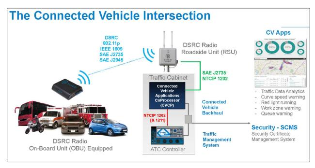
Figure 4-10 The Signal Controller and Econolite CV Co-Processer as Part of the Connected Vehicle Intersection (Provenzano, 2016; Mohaddes, 2017)
