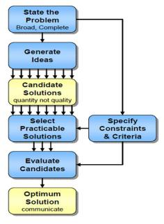
Figure 2-2 Basic Trade Study Techniques in the Concept Exploration as Presented in the Systems Engineering Guide (USDOT, 2007)
