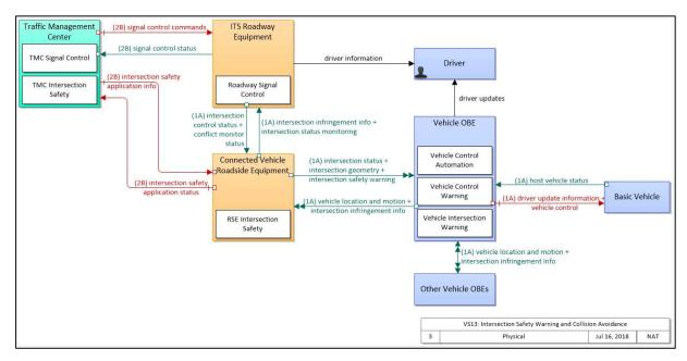
Figure 4-7 VS13 Intersection Safety Warning and Collision Avoidance (ARC-IT 8.2, 2019).
