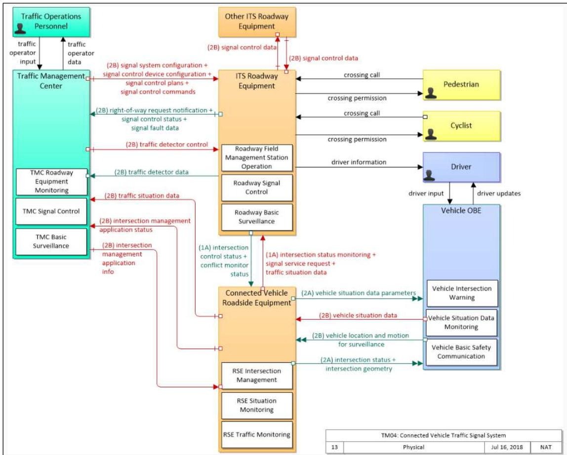
Figure 4-4 TM04 Connected Vehicle Traffic Signal System (ARC-IT 8.2, 2019)
