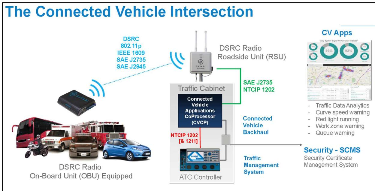
**Figure 4-10 The Signal Controller and Econolite CV Co-Processor as Part of the Connected Vehicle Intersection (Provenzano, 2016; Mohaddes, 2017)**
