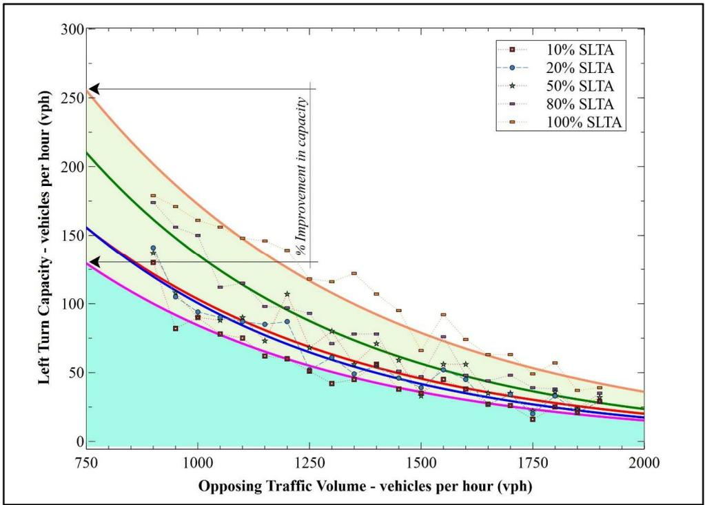
**Figure 5-19 Impact of SLTA on Left-Turn Capacity**
