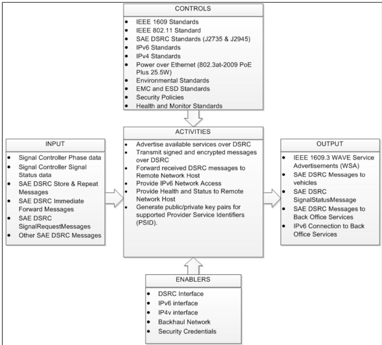
**Figure 4-12 Context Diagram of an RSU (Chang, 2017)**
