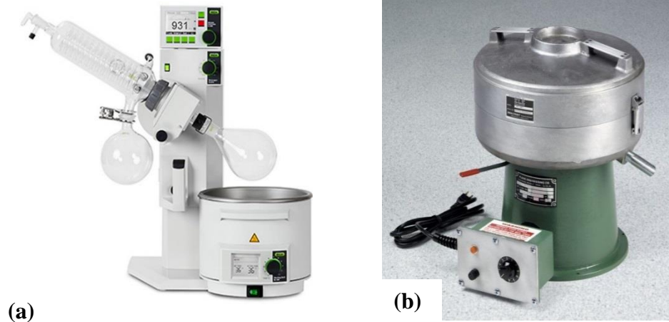
Figure 3-1. Binder Recovery Apparatus: (a) Rotary Evaporator and (b) Centrifuge Extractor.
