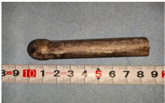
Metallic object found in grout
