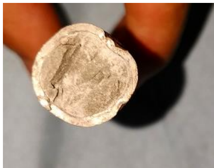
Metallic object found in grout
