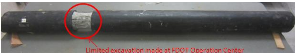
Figure 46. Tendon sample #2 before full autopsy.
