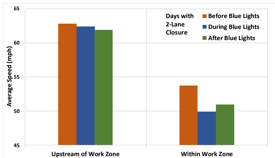
Figure 4-10. Overall Average Speeds Upstream of & within Work Zone for 2-Lane Closure
