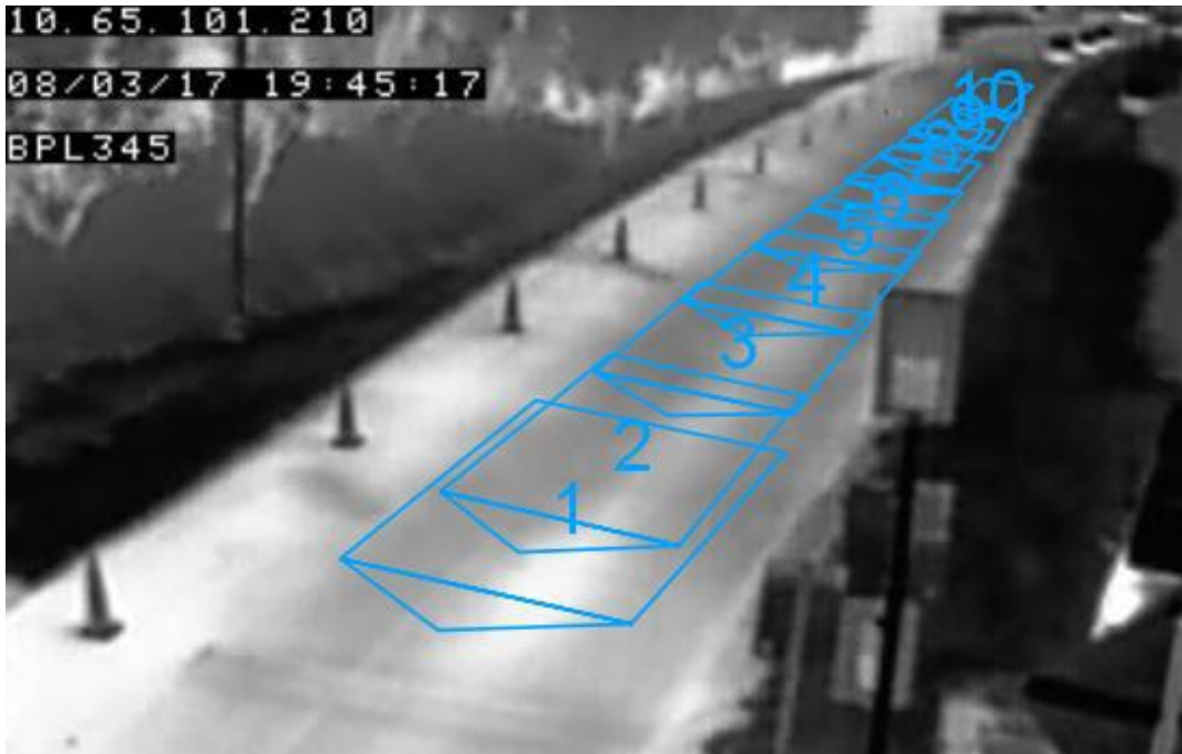
Figure 4-13. FLIR Video Camera Detection Zones for Queue Lengths
