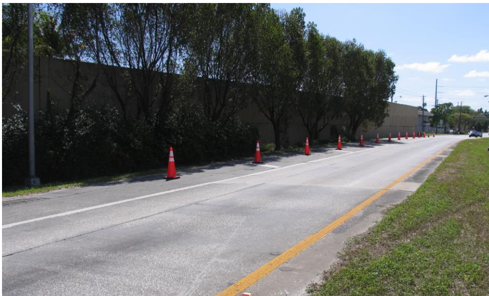
Figure 4-1. Traffic Cones Serving as Markers for Quick Distance Measurement
