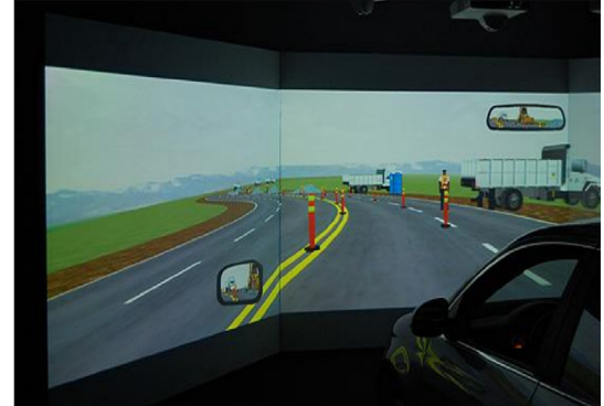
In this driving test, a highway with an express lane was simulated to gauge drivers' ability to identify lane markers.
