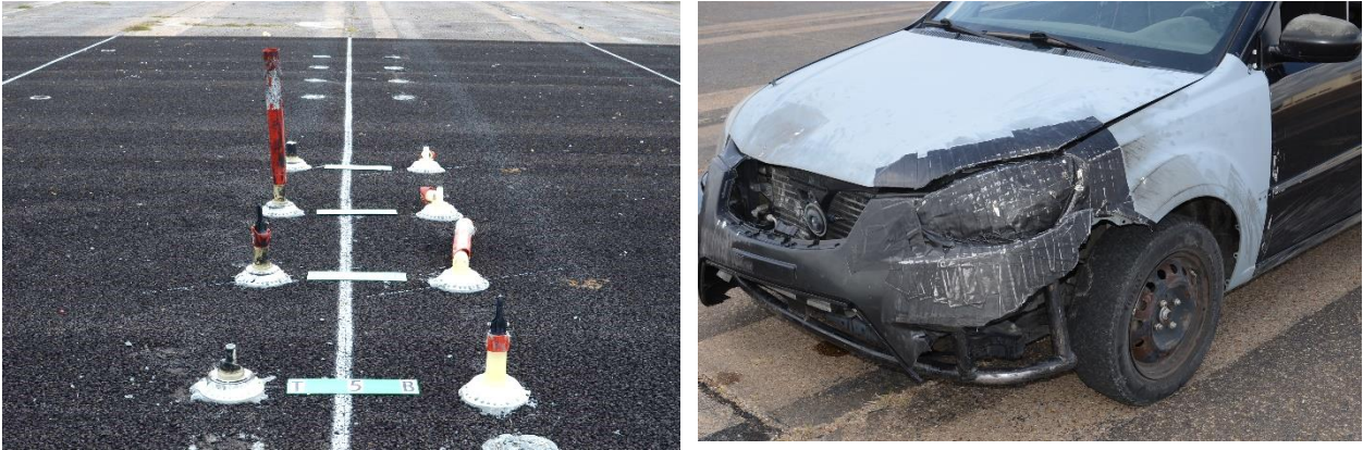
Figure 3.31. 607531-02-7 Delineators and Test Vehicle after Testing (Asphalt Surface).
