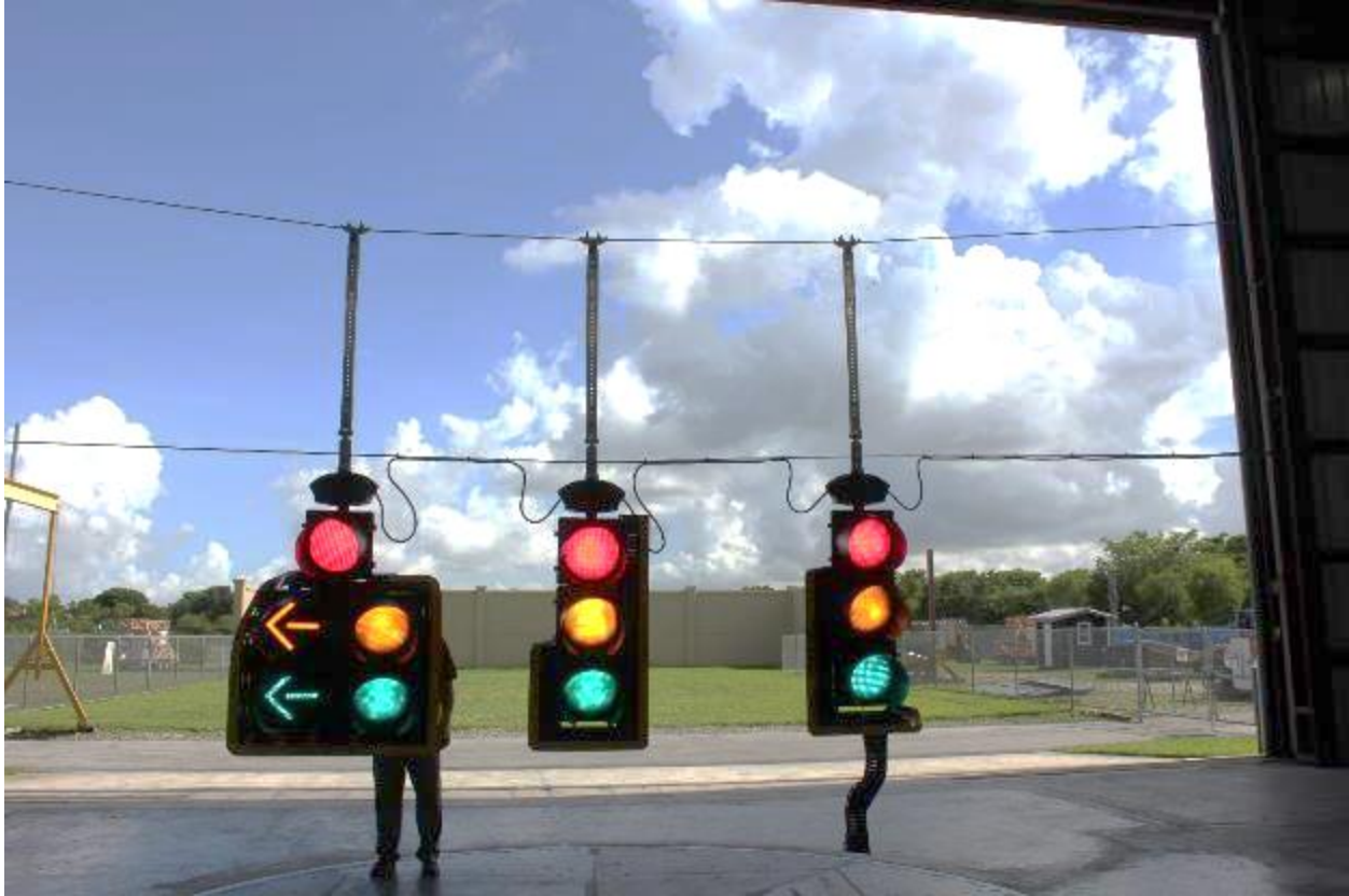
Figure 26: Signal Assembly after full wind speed test
