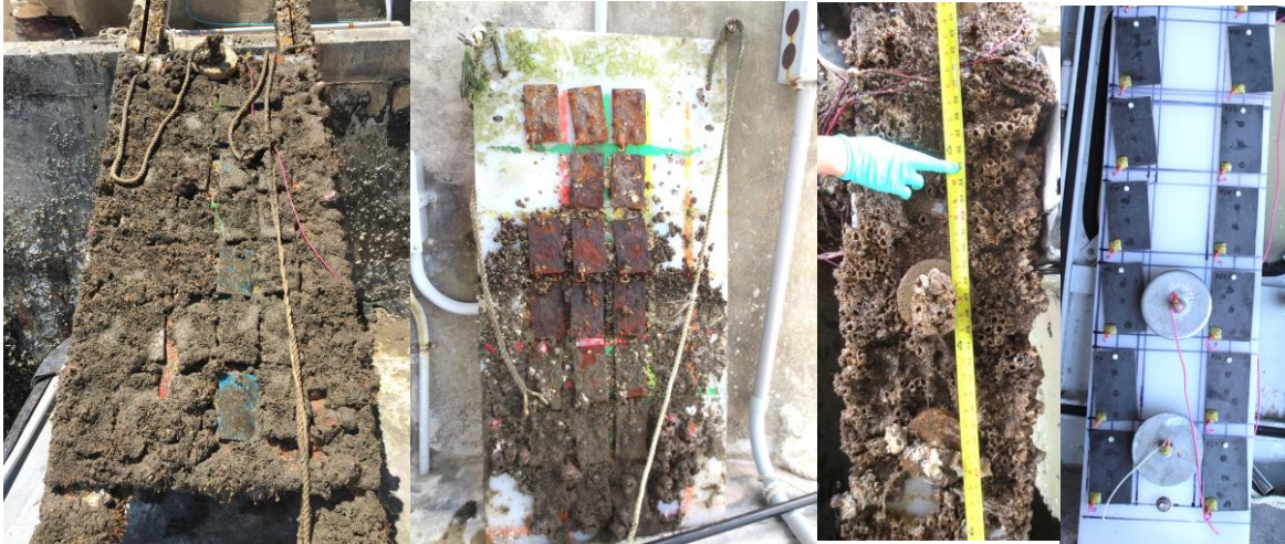
Figure 7.1. Typical Outdoor Exposure Test Rack.
