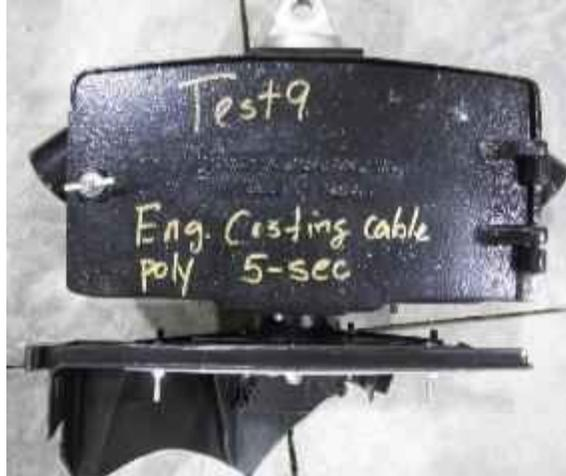
*Figure 162: Disconnect box with a piece of the 5-section signal*
