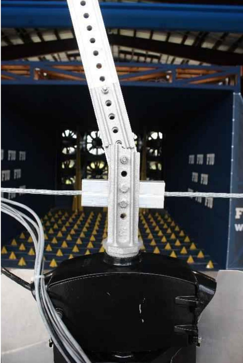
*Figure 181: Sheared Hanger Connection*
