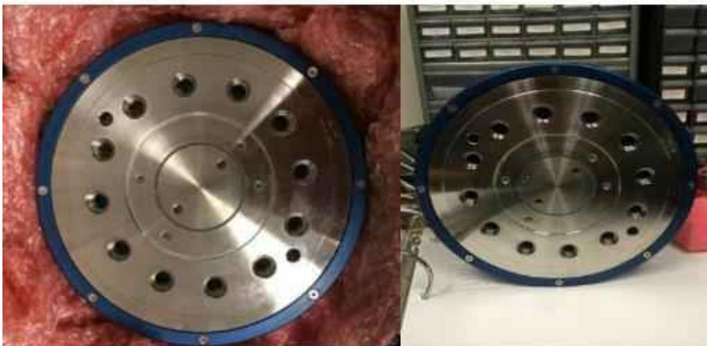
*Figure 7: Picture of -degree of freedom loadcells*
