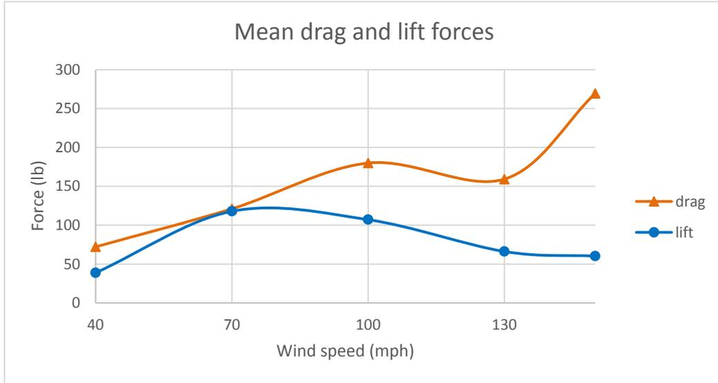
Figure H 1: Mean drag and lift forces on the traffic signals at 45 degrees wind direction
