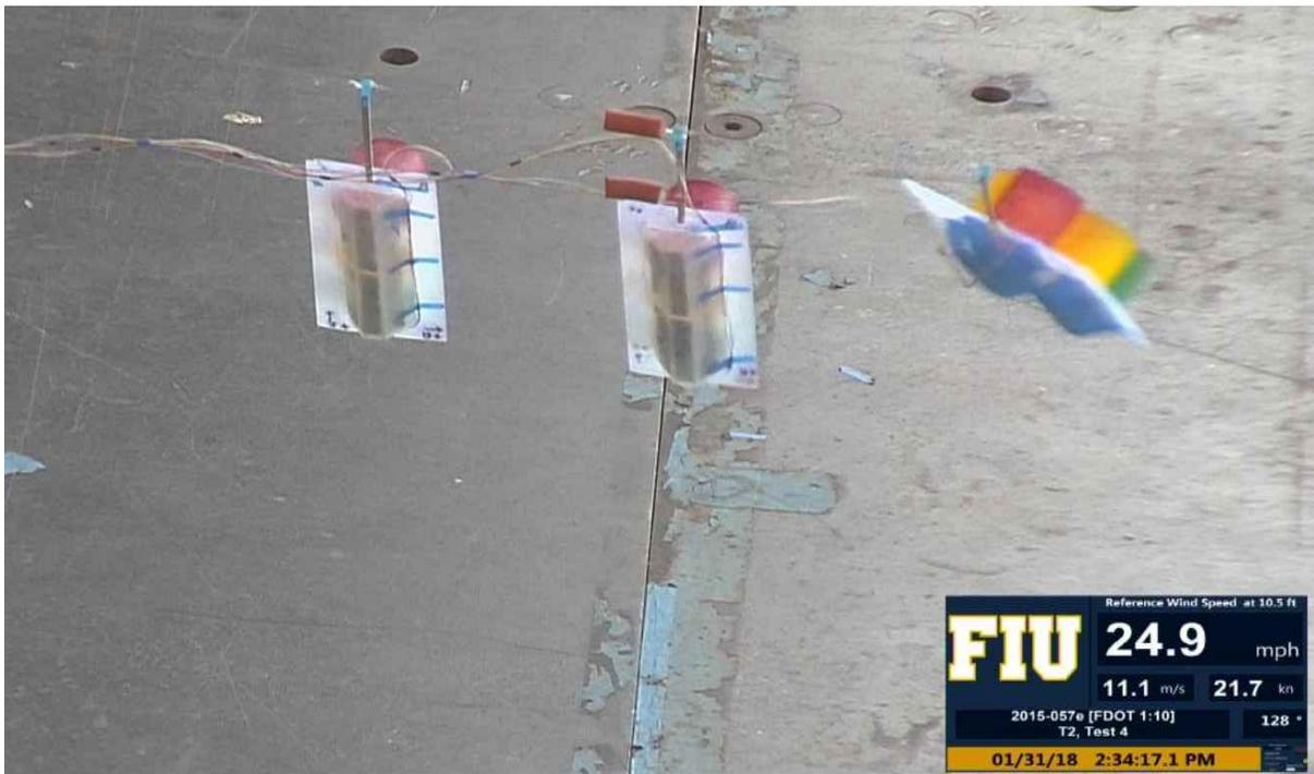
Figure 219: Fluttering at 135° angle of attack
