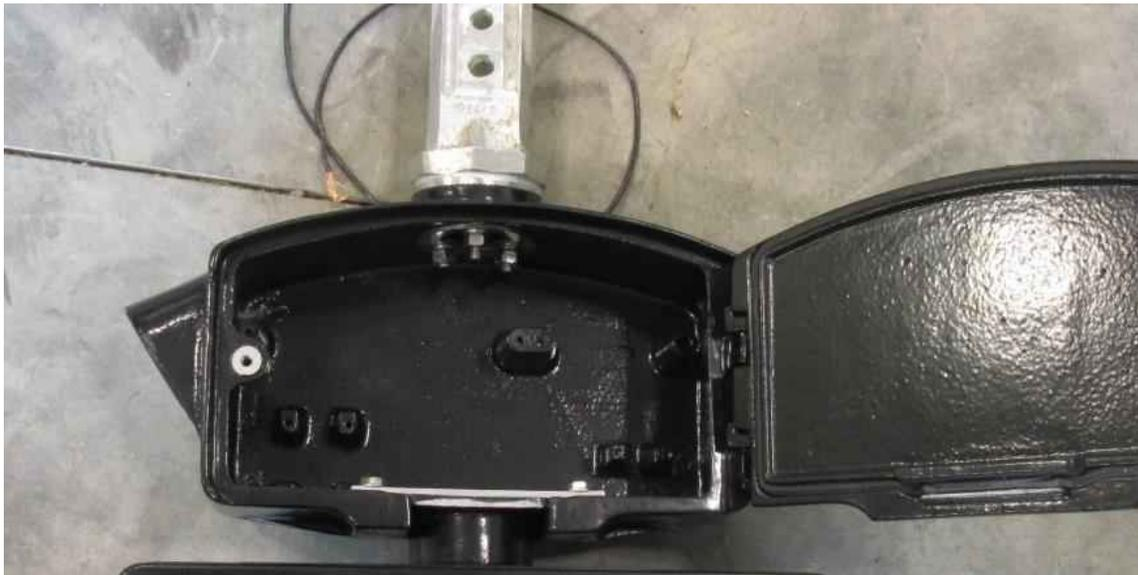
*Figure 131: Disconnect box for 3-section signal with no visible damage (all wiring removed)*
