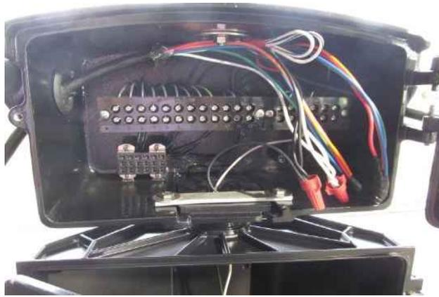
*Figure 114: Disconnect box for 3-section traffic signal after test*
