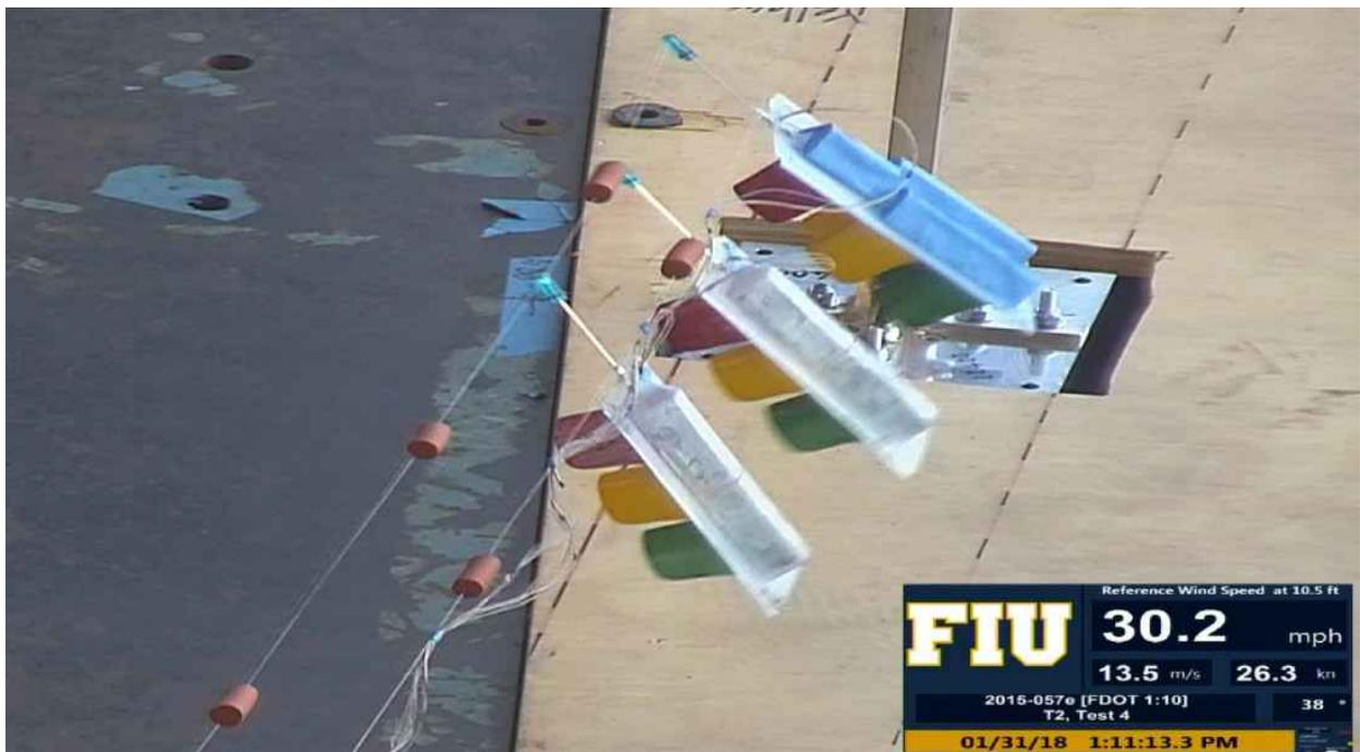
Figure 217: Aerodynamic instabilities at angle 45°
