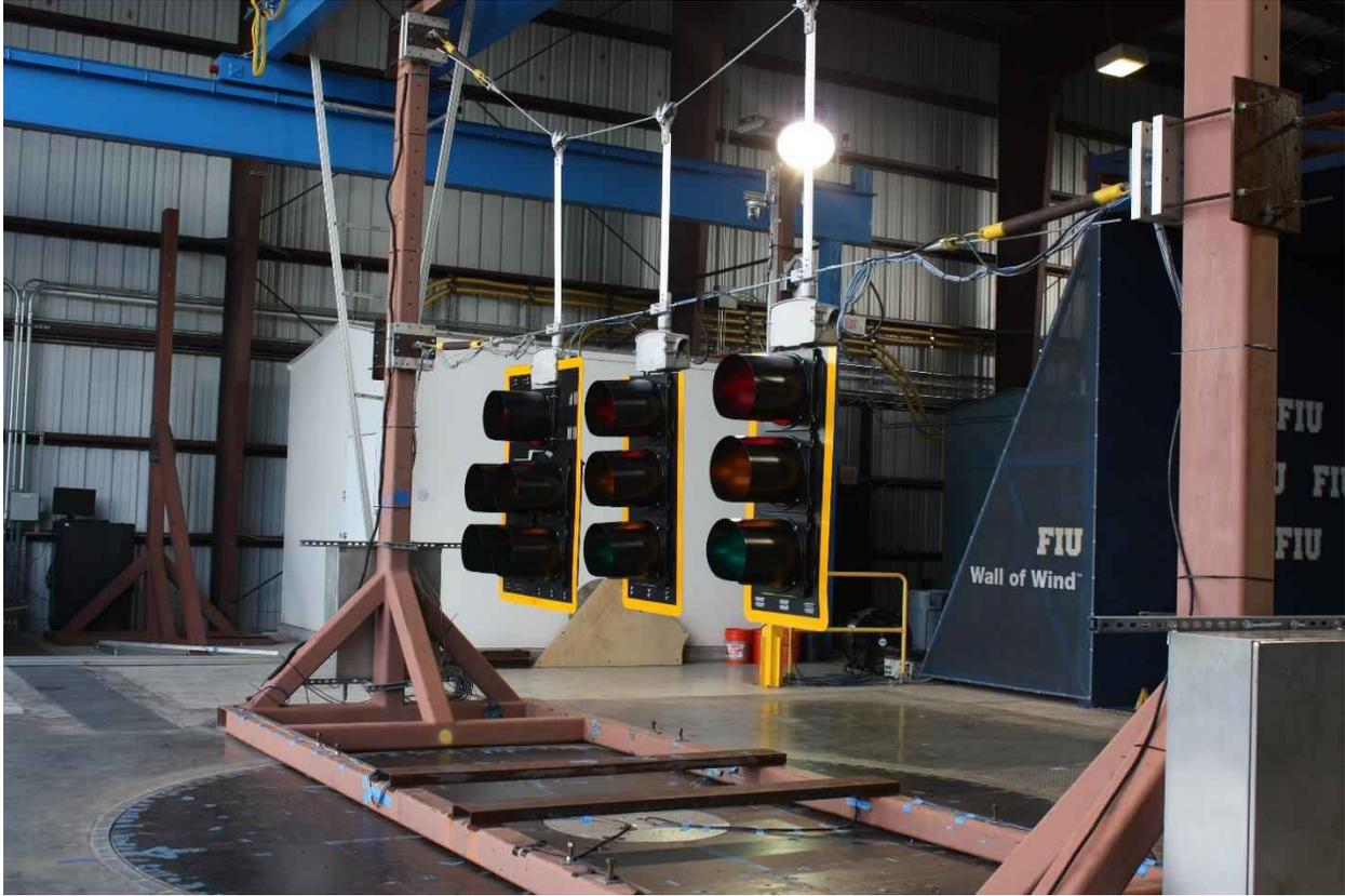
*Figure 230: Side view of the test rig with the traffic lights*
