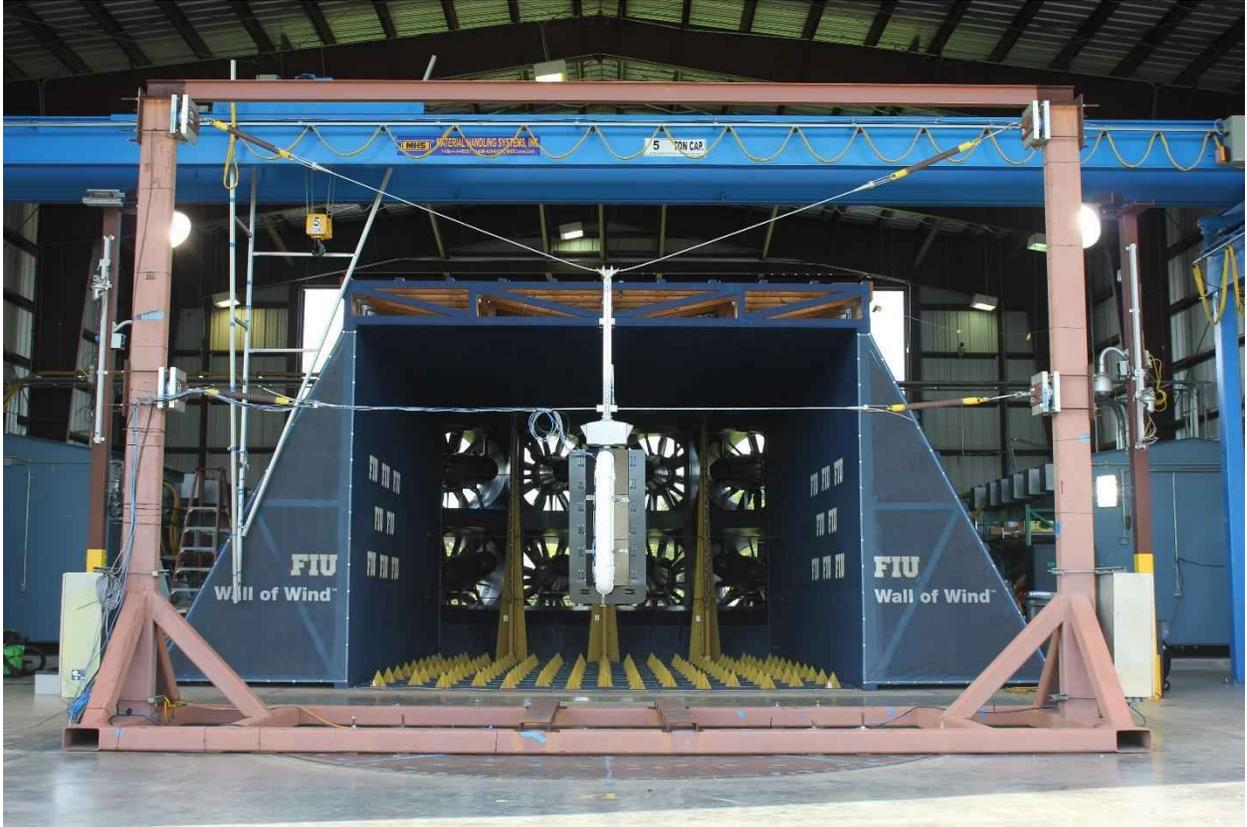
*Figure 257: Signal assembly installed on test rig (before testing) with liquid damper (with two liters of water)*
