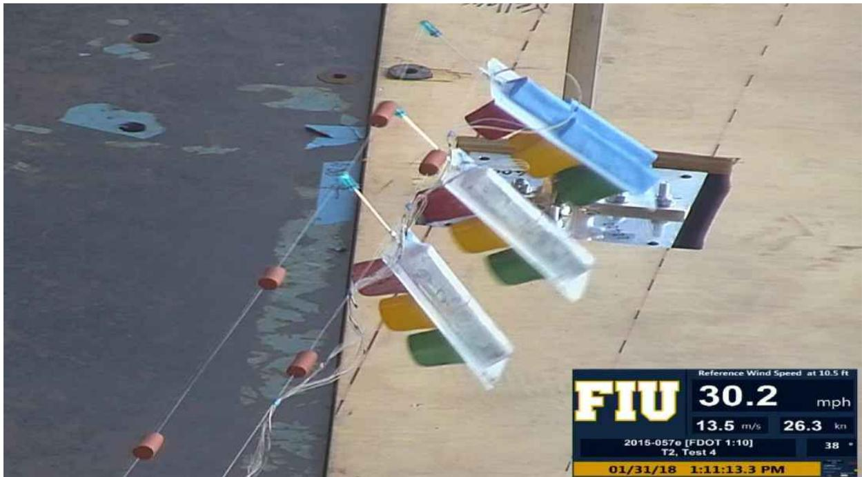
Figure 217: Aerodynamic instabilities at angle 45°
