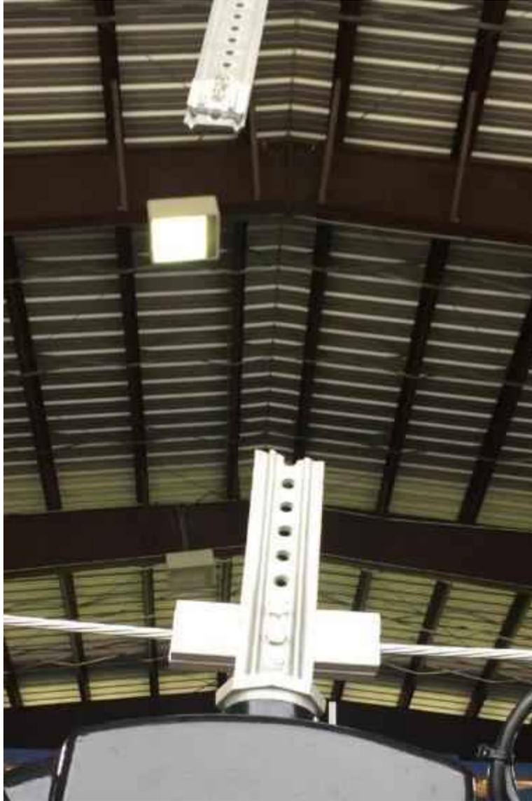
*Figure 33: Tri-stud adjustable hanger after Test 1 showing location of damage. No noticeable damage to the extruded aluminum messenger wire clamp*
