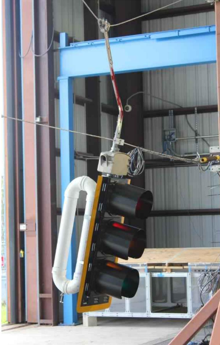
*Figure 281: "Liquid-damper-with-OL case" after 150 mph at 0 degrees*
