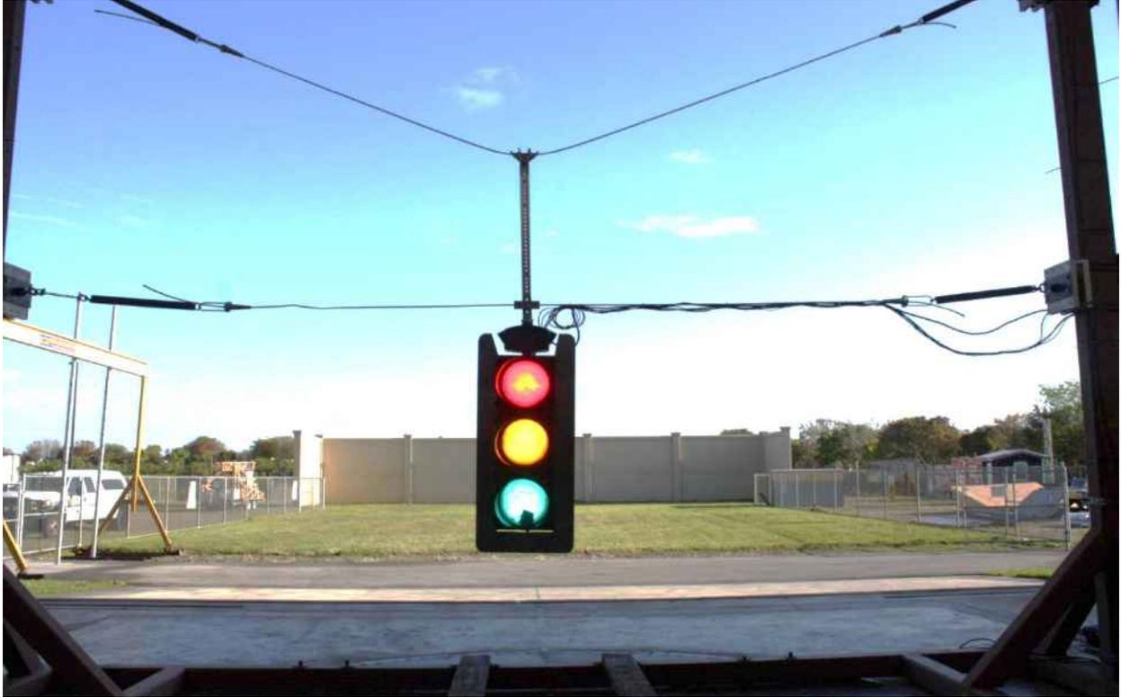
*Figure 166: Signal assembly installed on test rig (before testing)*
