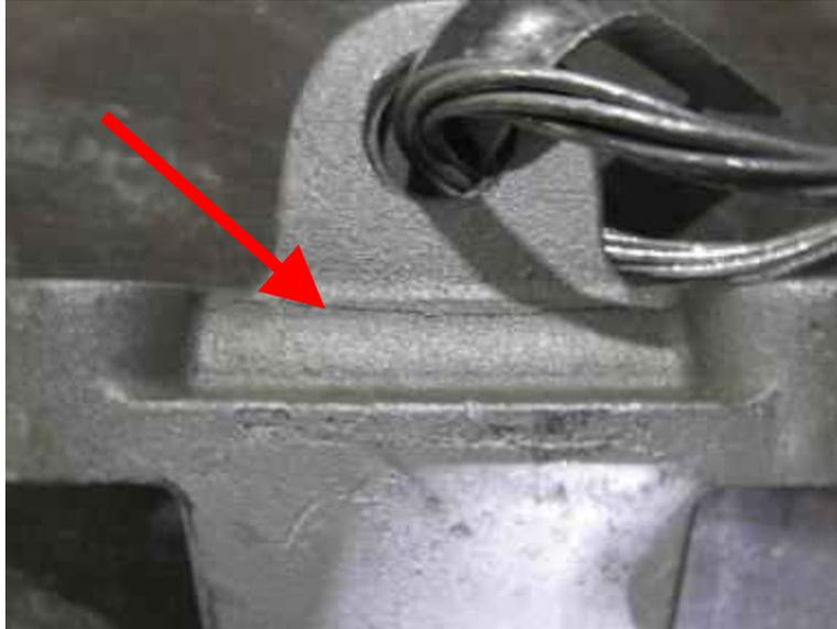
*Figure 160: Hairline crack on 5-section signal messenger clamp*
