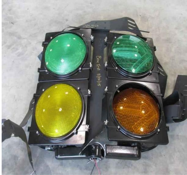
*Figure 128: Lower portion of 5-section signal that severed*
