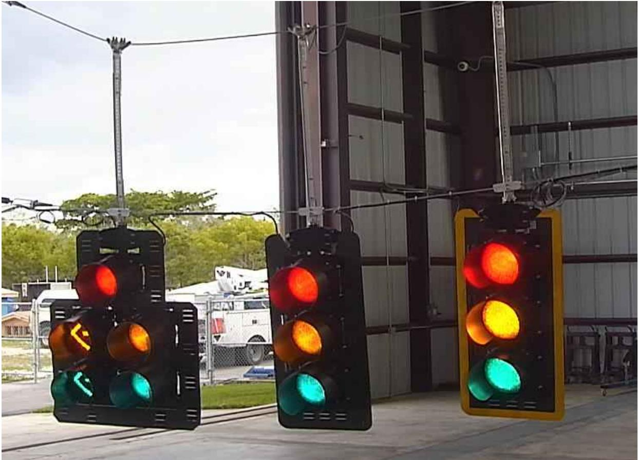
*Figure 116: Picture showing a portion of the test rig frame with the tri-stud adjustable hanger system*
