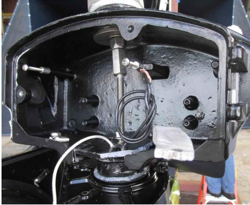
*Figure 83: Disconnect box for 5-section signal after the completion of test*
