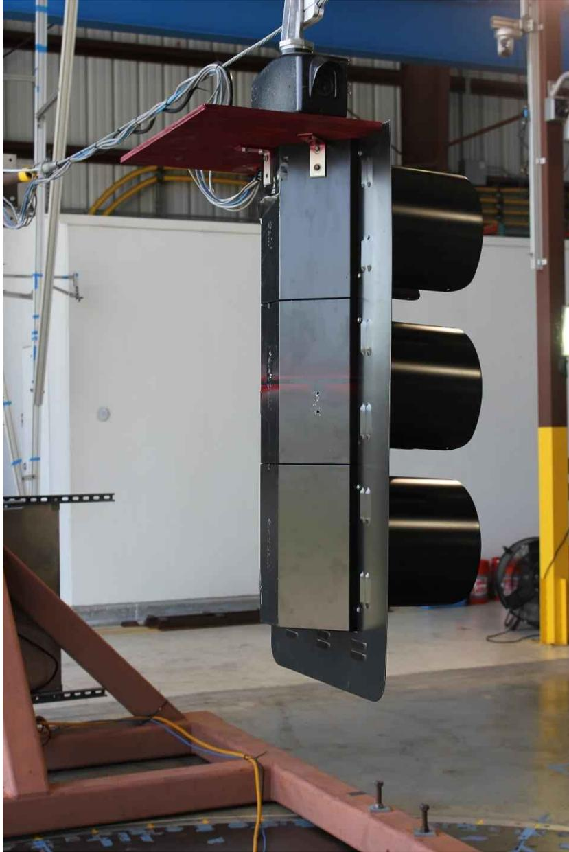
*Figure 261: Close up of fin located at top of signal housing*
