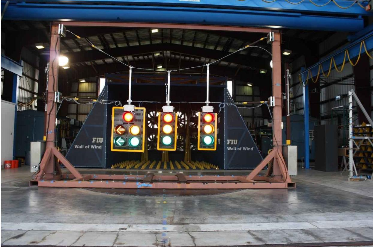
*Figure 231: Signal assemblies installed on test rig (before testing)*
