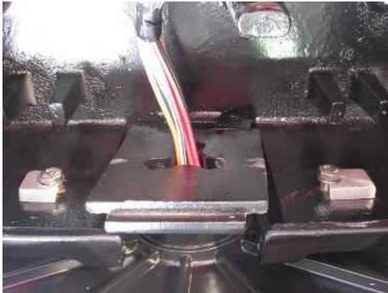
*Figure 97: Cracked lower clamp inside 5-section disconnect box*
