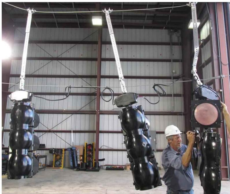
*Figure 82: Signal assembly after full wind speed test*
