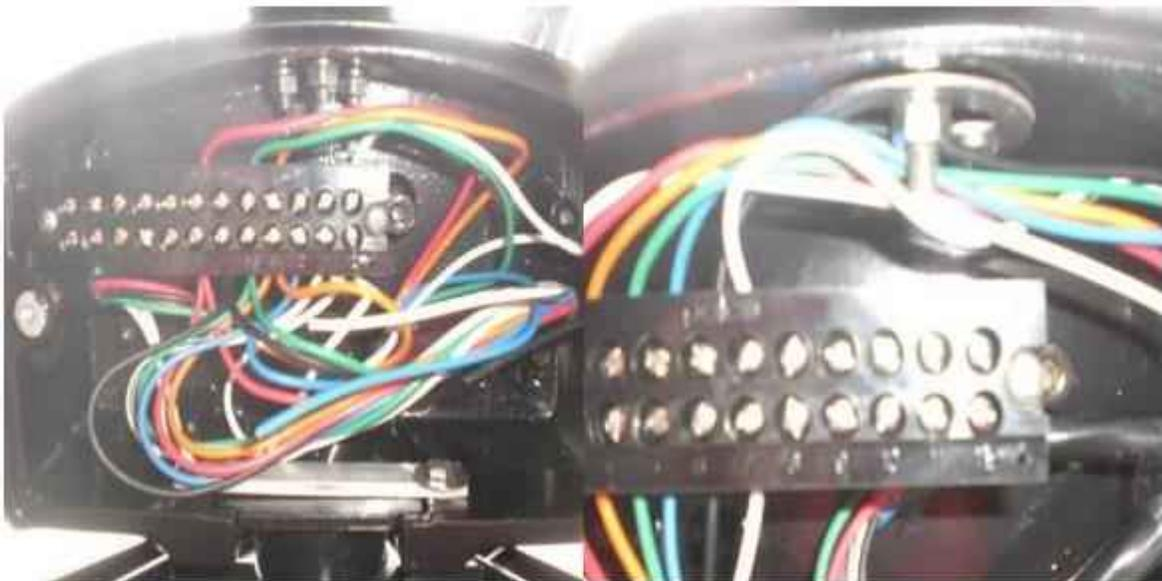
*Figure 51: Disconnect box for 4-section signal after Test 2 showing no noticeable damage*
