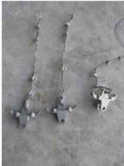
*Figure 99: Steel cable hangers after full wind test*
