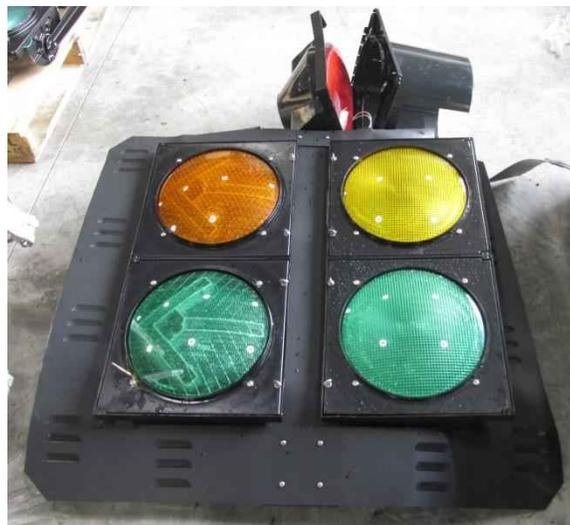
*Figure 145: 5-section polycarbonate signal after completion of full test cycle*
