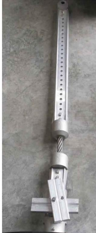
*Figure 144: Pelco adjustable hanger assembly after test completion*
