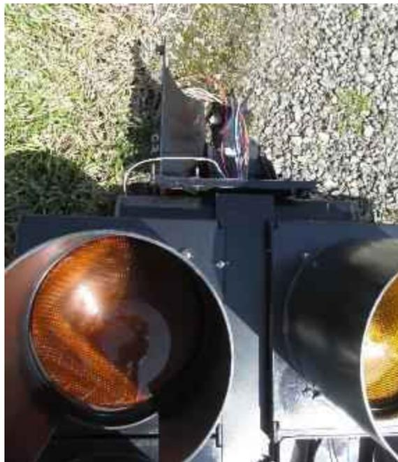
*Figure 161: 5-section polycarbonate signal cracked at the top*
