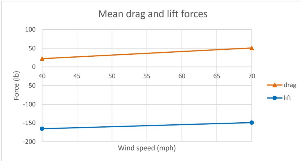
*Figure D 4: Mean drag and lift forces on the traffic signals at 80 degrees wind direction*
