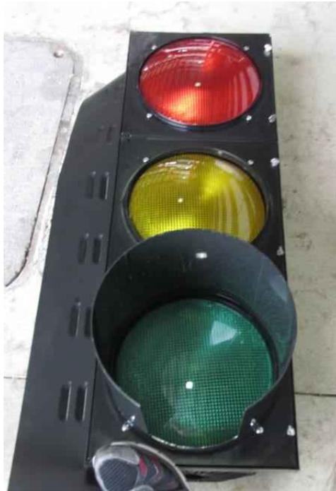
*Figure 146: 3-section polycarbonate signal after completion of full test cycle*
