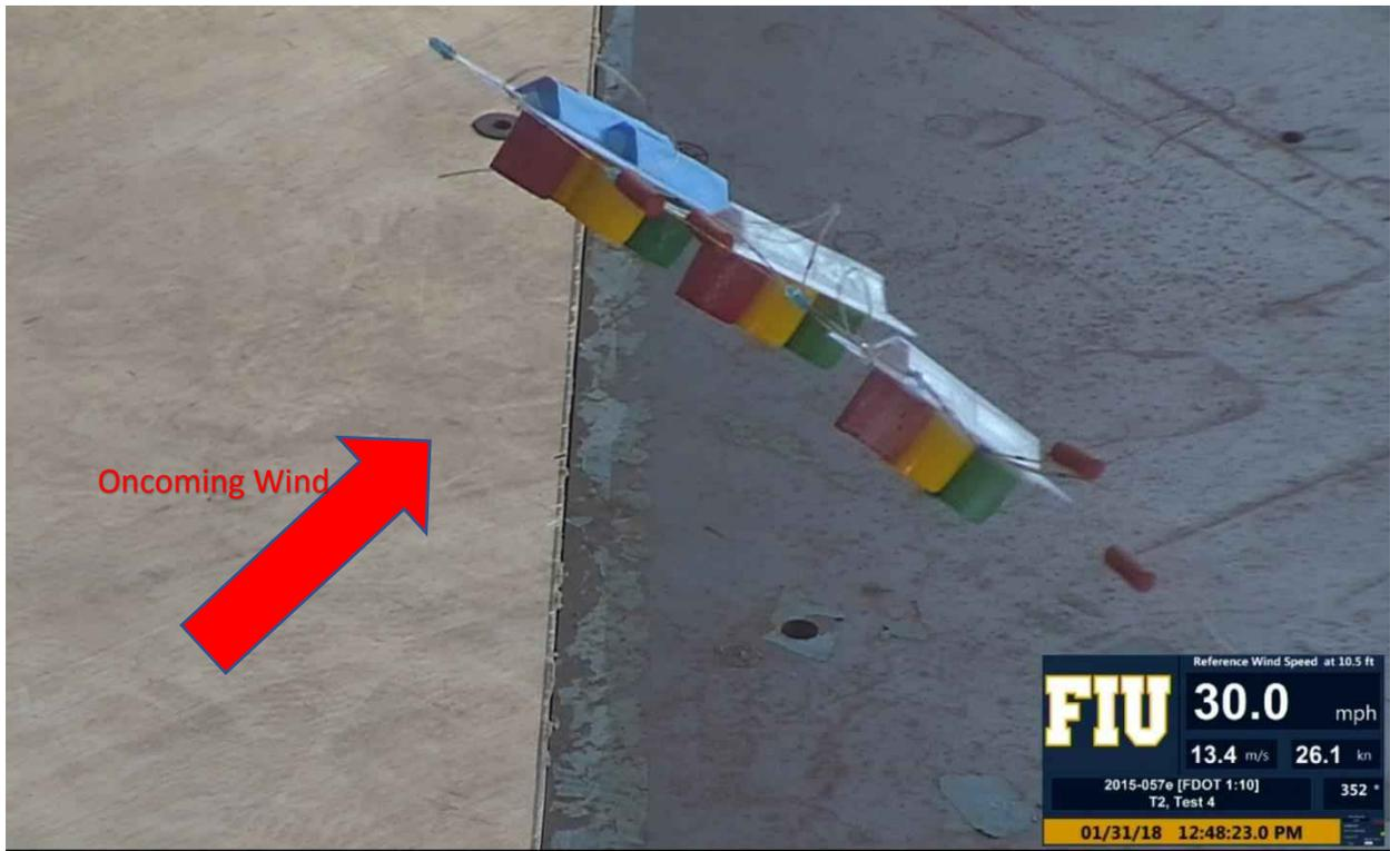
Figure 216: Backward tilting of traffic signals
