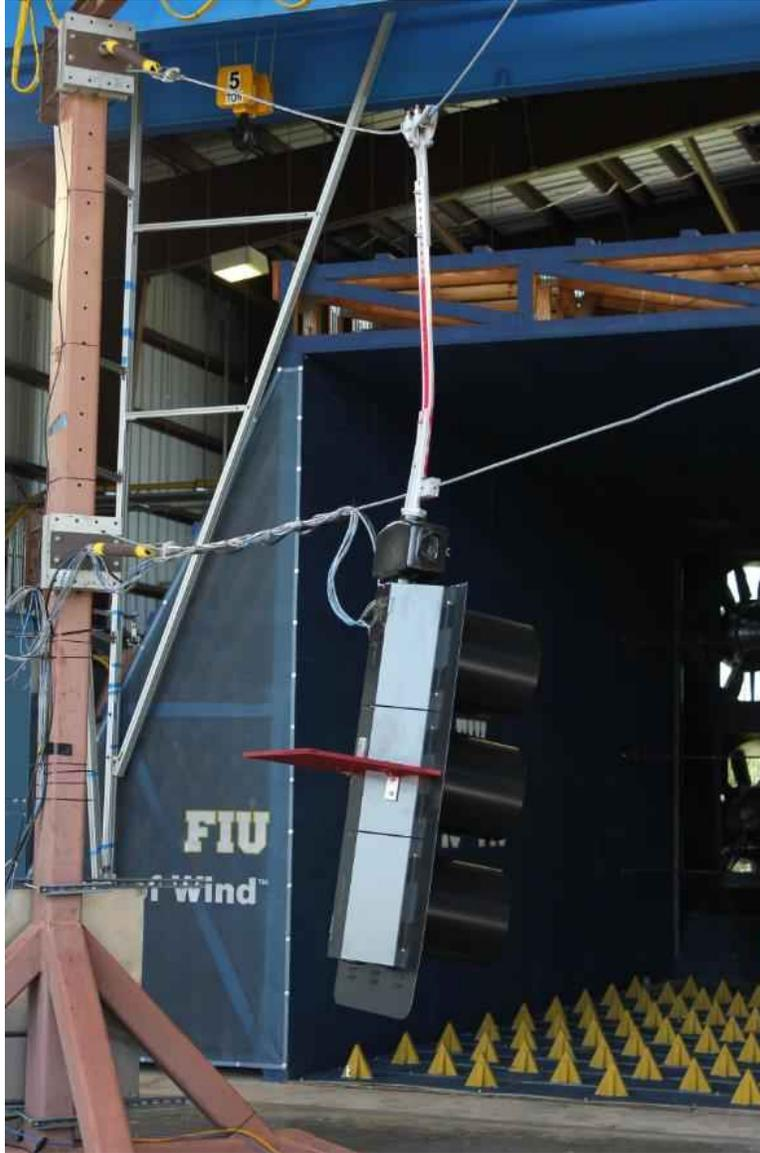
*Figure 283: "Fin-at-middle case" after 150 mph at 0 degrees*
