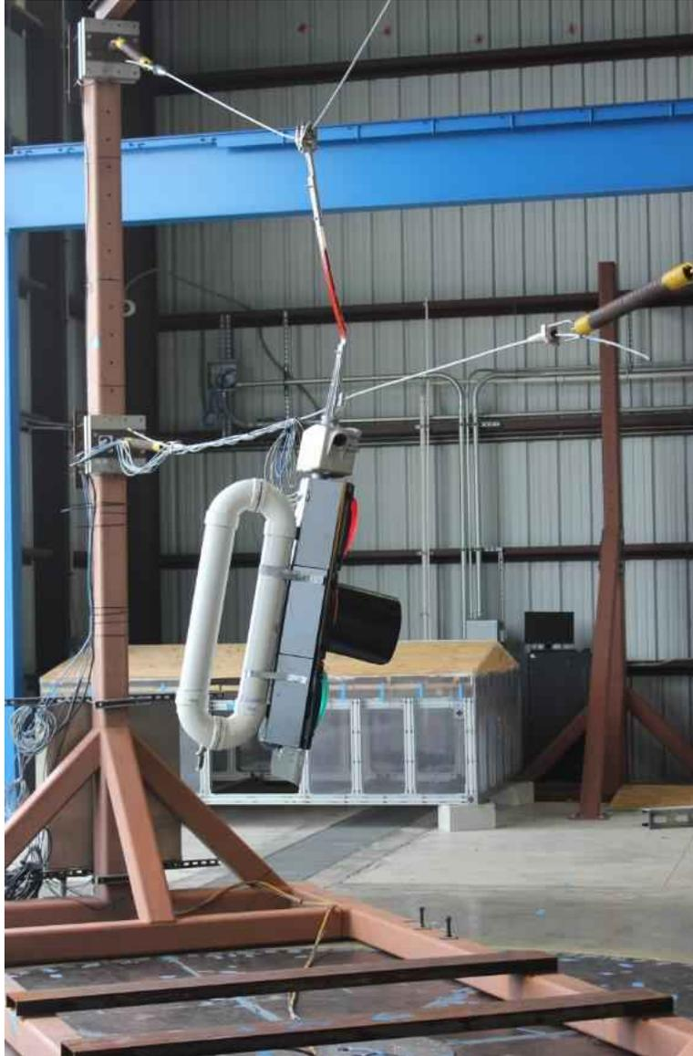
*Figure 280: "Liquid-damper-with-2L case" after 150 mph at 0 degrees*
