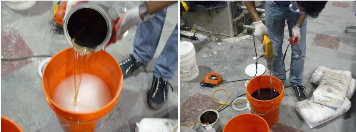
Figure A-7: Parts A & B (resin & hardener) mixed for 2 minutes using a drill and mixing prop
