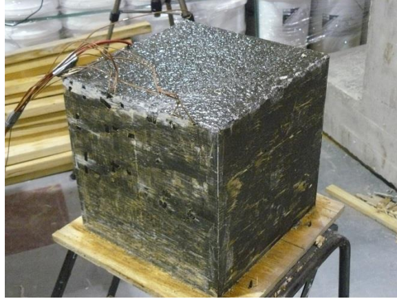
Figure A-11: Five surfaces of specimen in contact with the ambient environment
