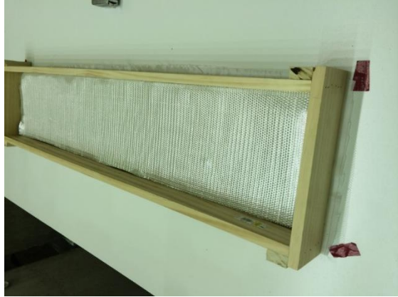
(b) Putting the side mold and laying the top glass fiber sheets
