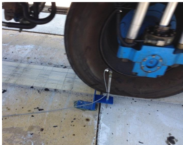
Figure 5.7 Instrumentation Plan on Decks and Support Beam (a) Strain Gauges on Support Beams, and (b) Relative Deflection Recording Device
