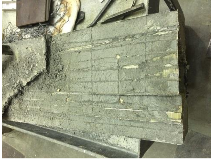
Figure 4.13 Bond between UHPC and Top FRP
