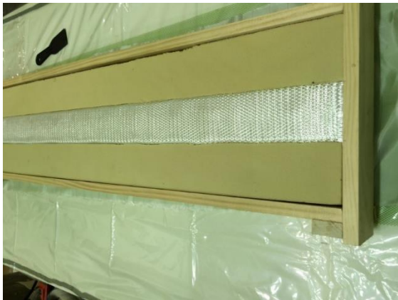
(c) Installing foam and laying shear fiber
