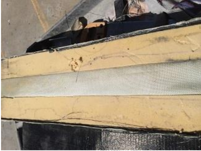
Figure 4.11 The FRP Cloth after Testing
