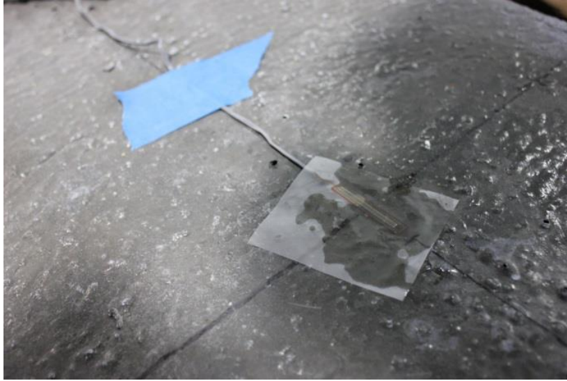
Figure A.1 Strain Gauge Attached to the Top Surface of the UHPC (Specimen 1T1S)
