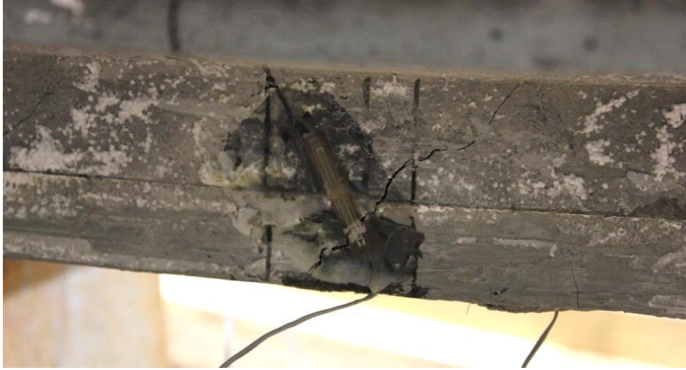
Figure B.1 Strain Gauge Attached to the Web (Specimen 1T1S)
