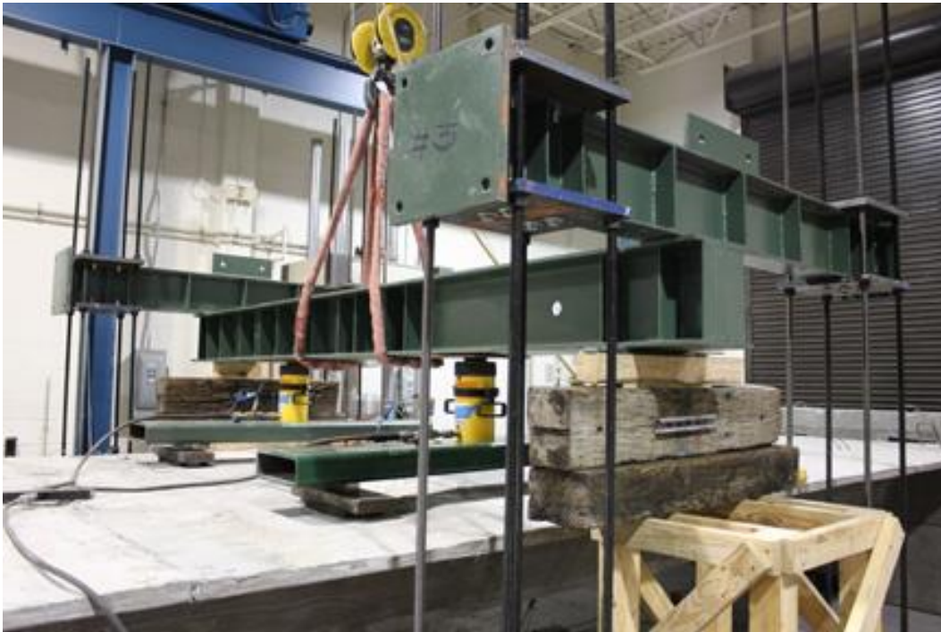
Figure B1. Test Setup for Service Load Position 1 and Ultimate Load Test
