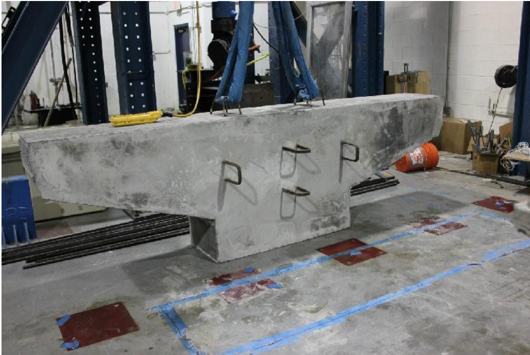
Figure D9. Specimen after Demolding
