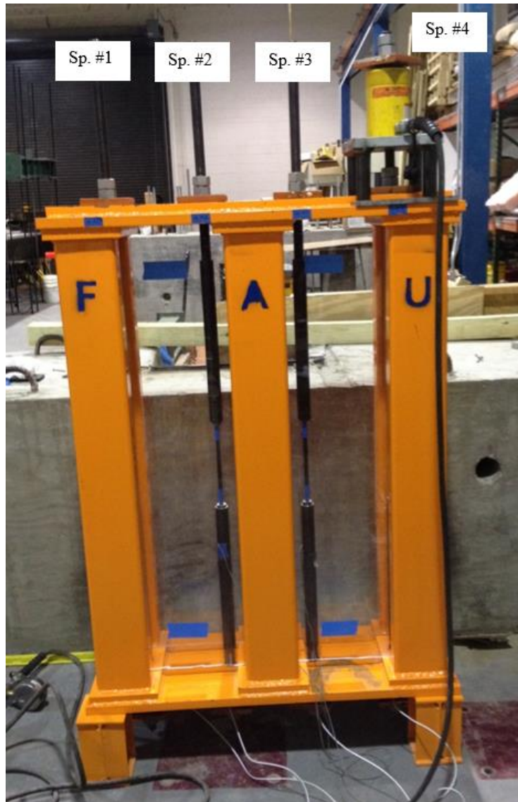
Figure 4.21 Four Specimen Loaded onto the Frame
