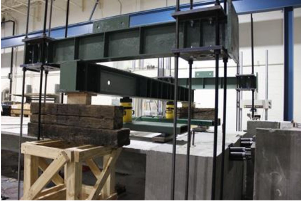
Figure B3. Test Setup for Service Load Position 3
