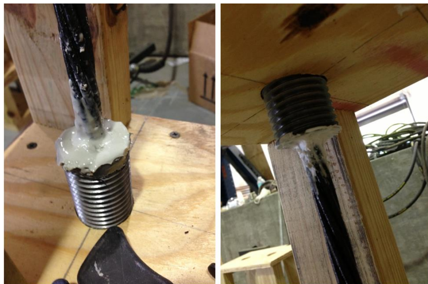
Figure 4.5 Epoxy Filler in Curing Process
