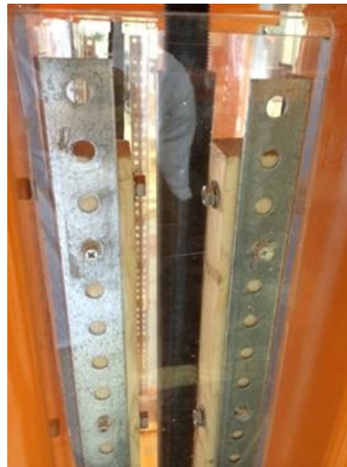
Figure 4.16 Protective Screen in Testing Frame
