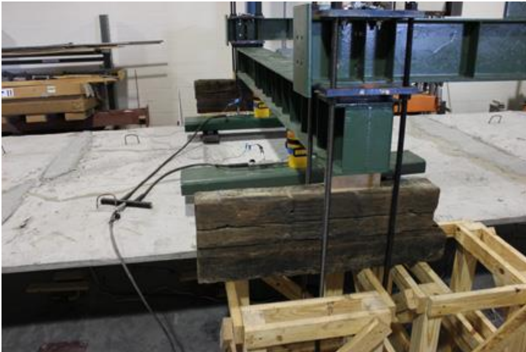
Figure B2. Test Setup for Service Load Position 2
