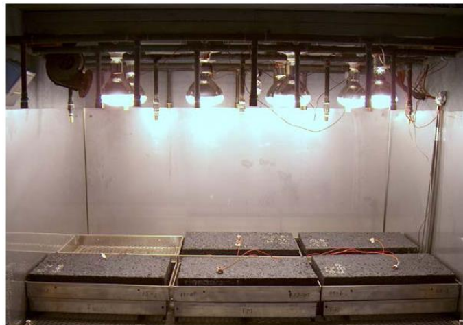
Figure 4-1 Accelerated Pavement Weathering System (APWS)
