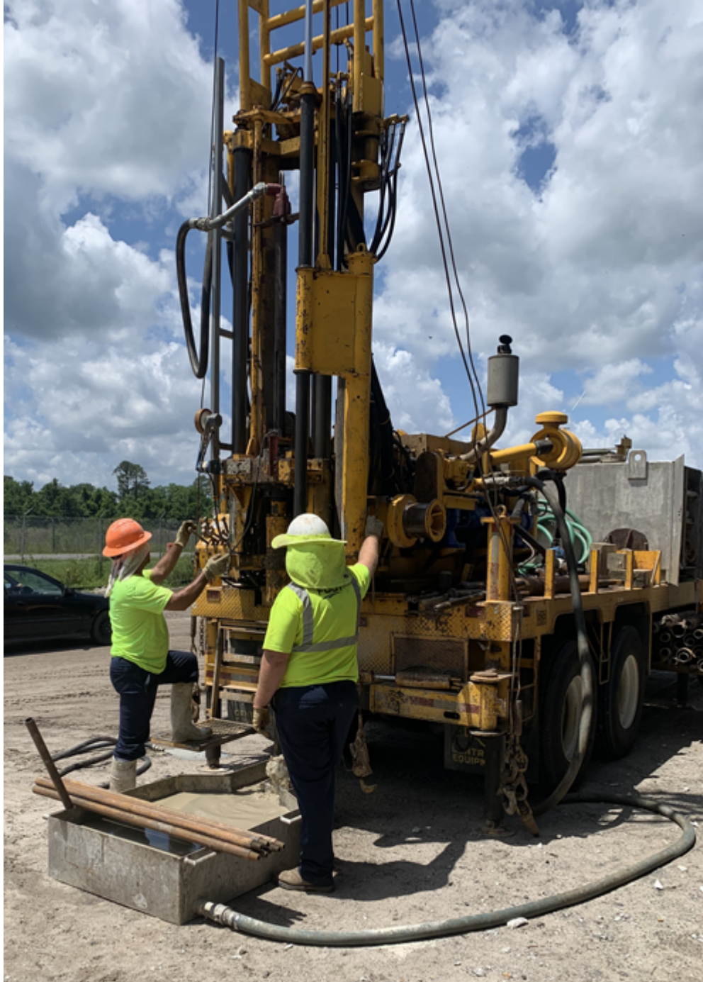
Figure 3-33 Photo of FDOT SMO Drill Rig used for SPT WLC 3 near Station 1239+20 testing
