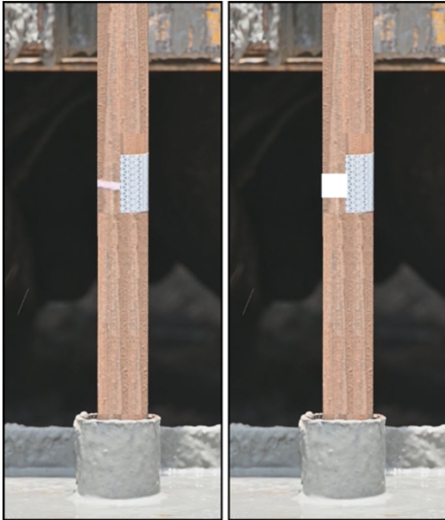
Figure 6-36 Proposed SPT Rod Chalk Line and PDM Tape Placement (Left) or White Electrical Tape and PDM Reflective Tape Layout (Right)
