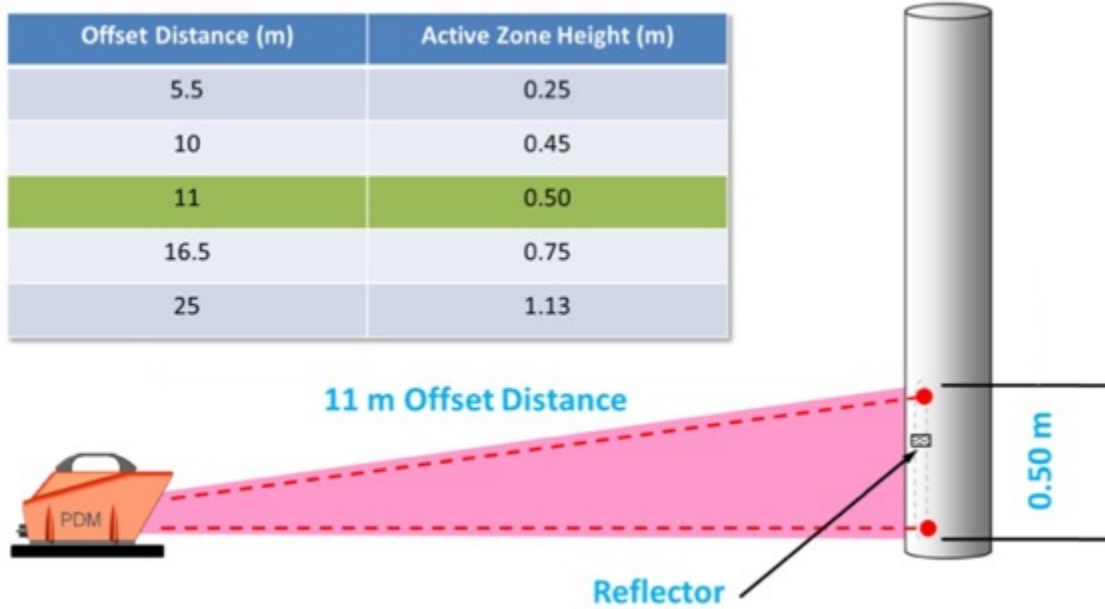
Figure H-1 Schematic of Inopiles Operation within Active Zone
