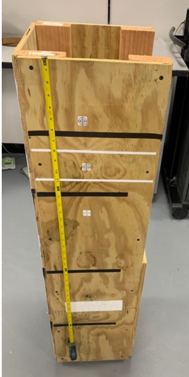
Figure D-7 Laboratory wooden simulated pile with PDM and CMS markings
