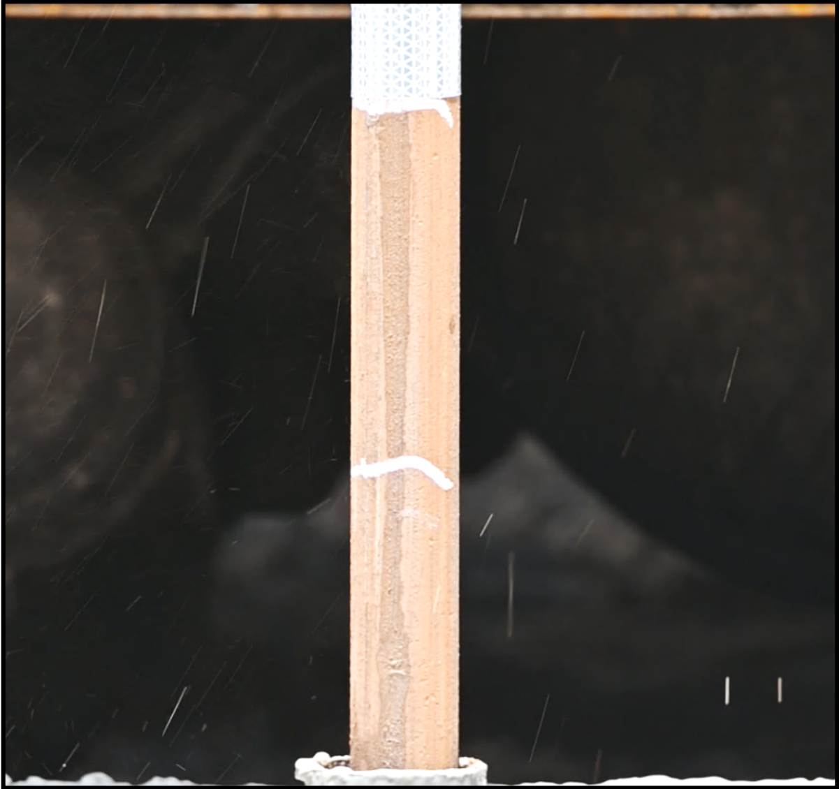
Figure 6-37 Video Frame with White Streaks from Drilling Mud, from Wekiva CMS Tests
