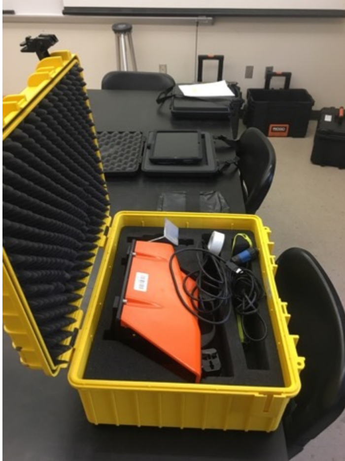
Figure H-2 Inopiles PDM in Case, leveling bag and Surface Pro®
