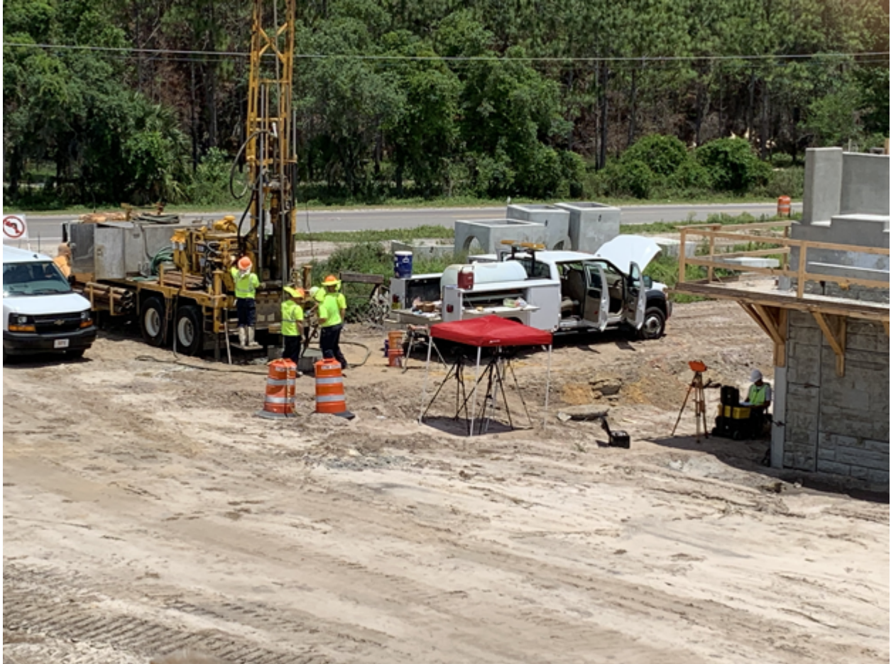
Figure 3-29 Photo of FDOT SMO Drill Rig used for SPT/PDM/CMS WLC 2 near Station 833+09 testing
