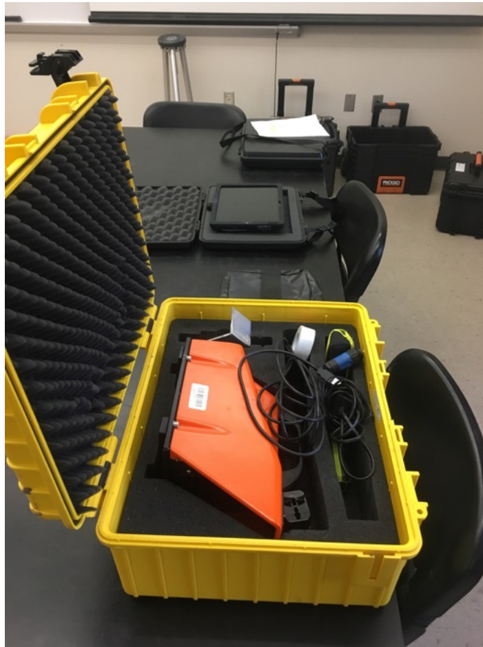
Figure 4-2 Inopiles PDM in Case, Leveling Bag, and Surface Pro®
