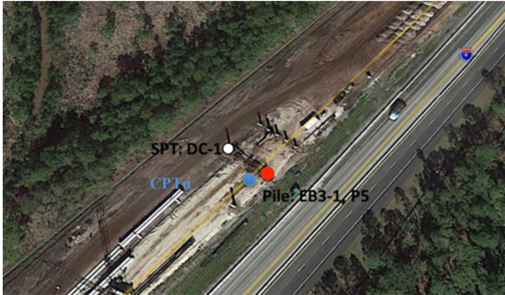
Figure 3-24: Test piles, SPT boring, and CPTu sounding locations for I-4 Widening Daytona
