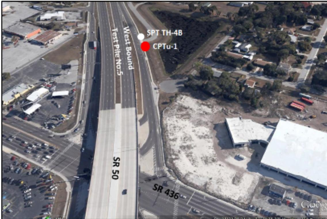
Figure 3-12: Test piles, SPT boring, and CPTu sounding locations for SR50/SR436
