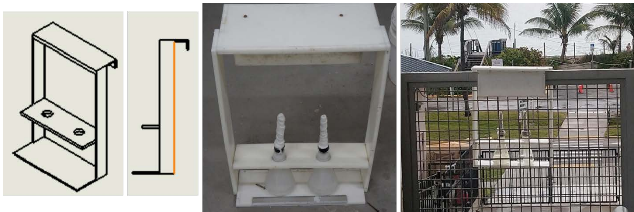
Figure 14. Wet candle setup deployed on the railing at SeaTech (21 ft 8" above MHWL). Left drawing, center front view, right deployed.
