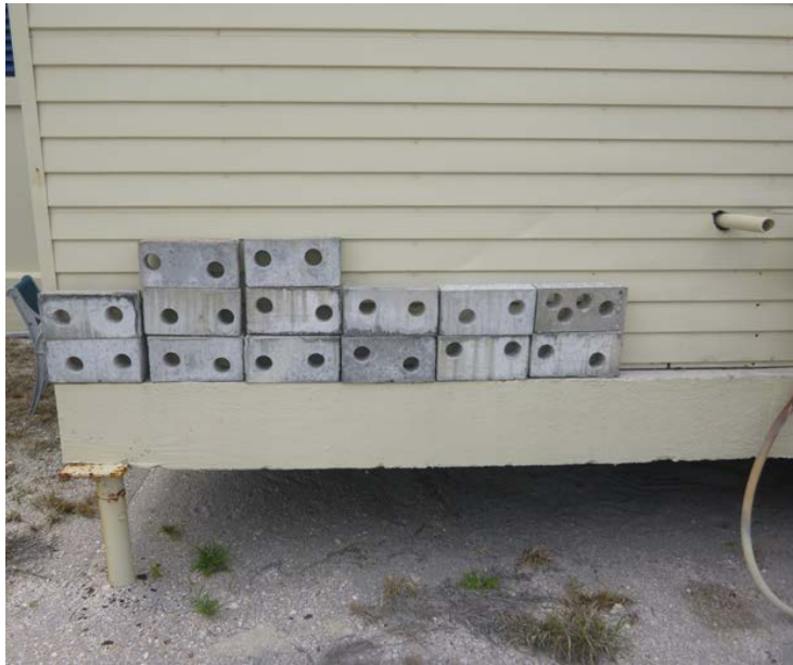
Figure 9. DCL samples exposed at the east site
