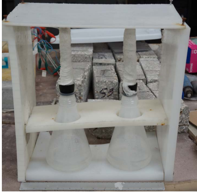
Figure 13. Wet candle setup deployed on the east site, at approximately 12 ft above MHWL.
