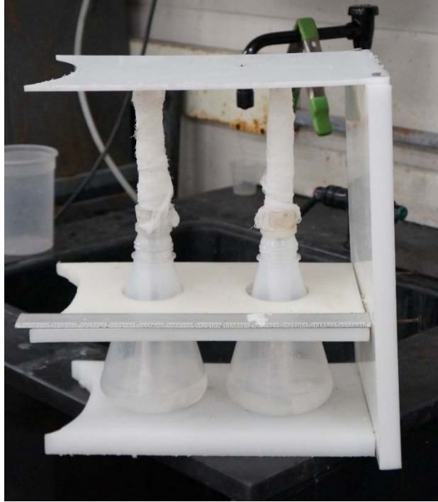
Figure 15. Setup for wet candle deployed on the palm tree next to bridge #860160.
