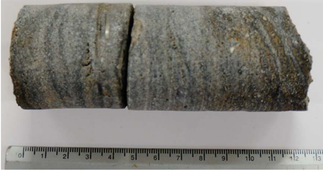
Figure 59. Shows a core obtained on bent 8 east column at 12 ft above MHWL (with CP jacket)
