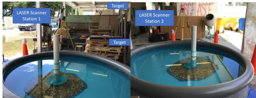
FIGURE 4-5. Laser scanner setup: station 1 (left); station 2 (right)
