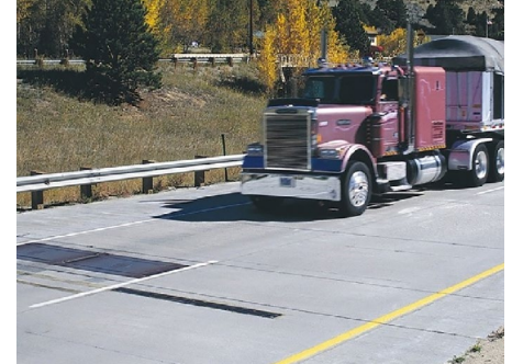
A truck approaches sensors embedded in the pavement that can capture the weight, the number of axles, and other information.
