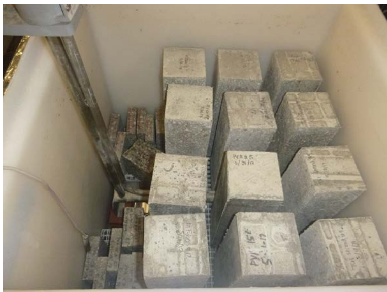
Figure 23. Samples being immersed in seawater (1 week wet one week dry).
