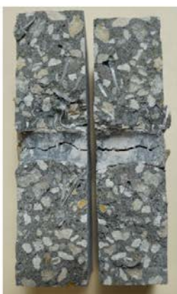
Figure 174. Visual inspection after modified IDT on mix 3 samples (HH)
