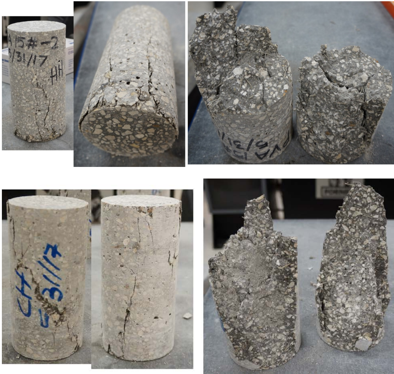
Figure 131. Visual inspection of fiber distribution after compression test on cores of mix 6
