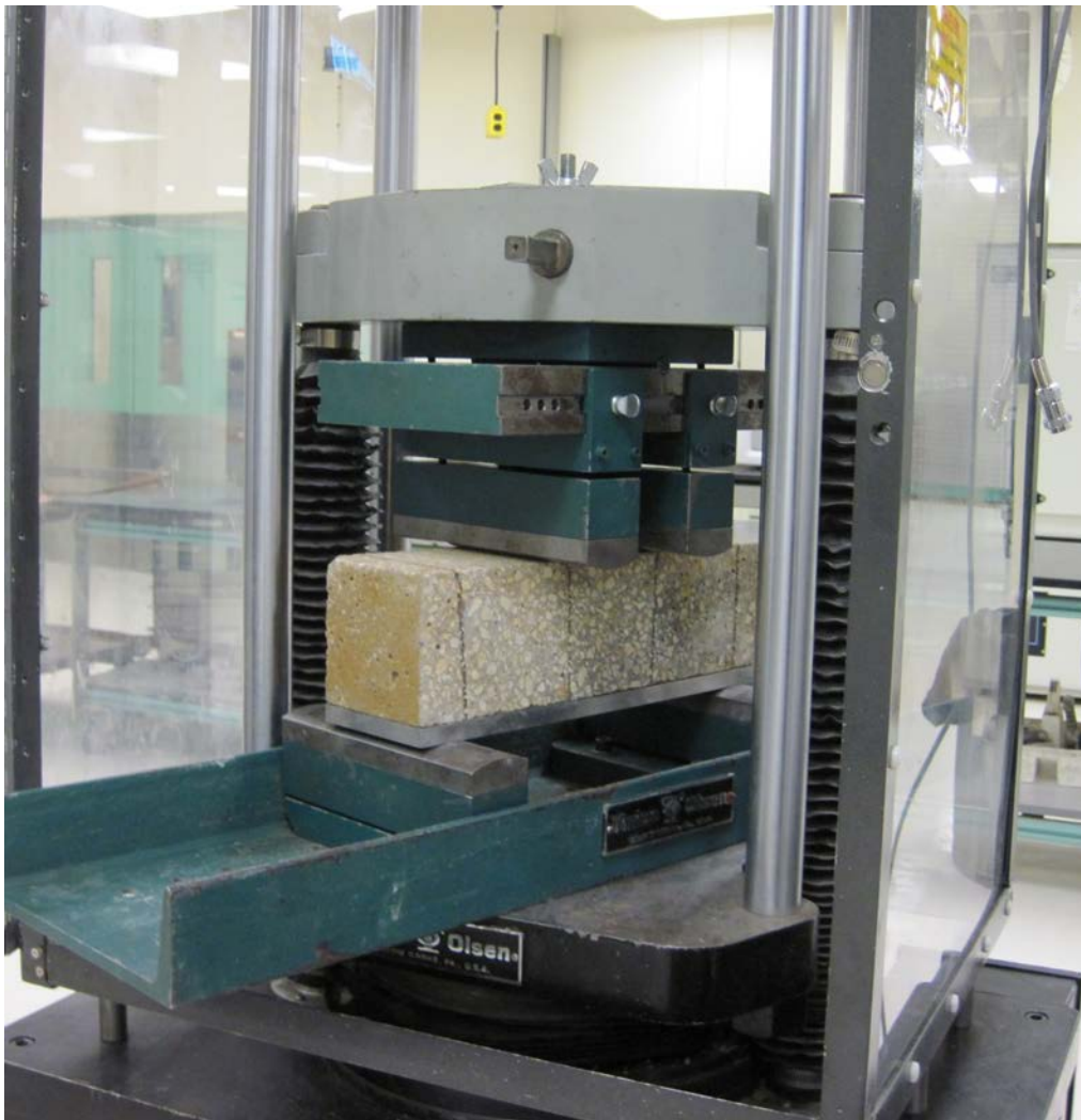
Figure 63. Sample in machine loaded to initial crack
