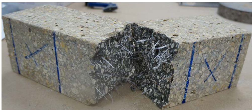
Figure 74. SW-LpH mix 5 beams after residual strength testing.
