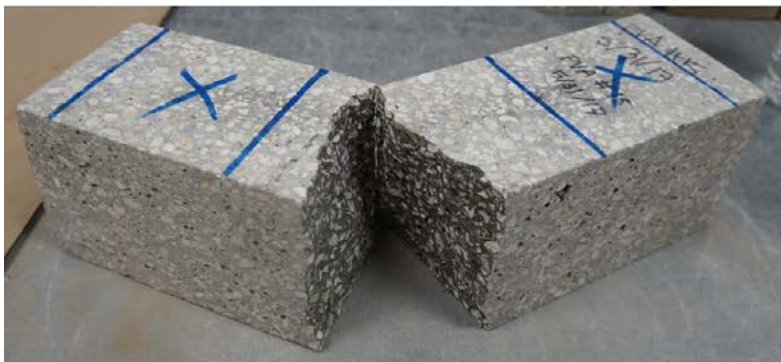
Figure 168. Fiber distribution after residual strength tests on beams of mix 6
