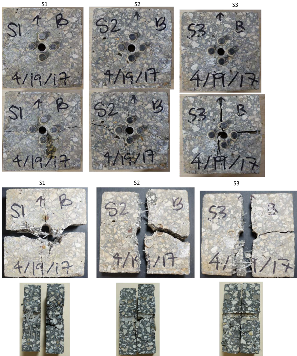
Figure 204. Visual inspection after modified IDT on mix 1 samples (at barge)
