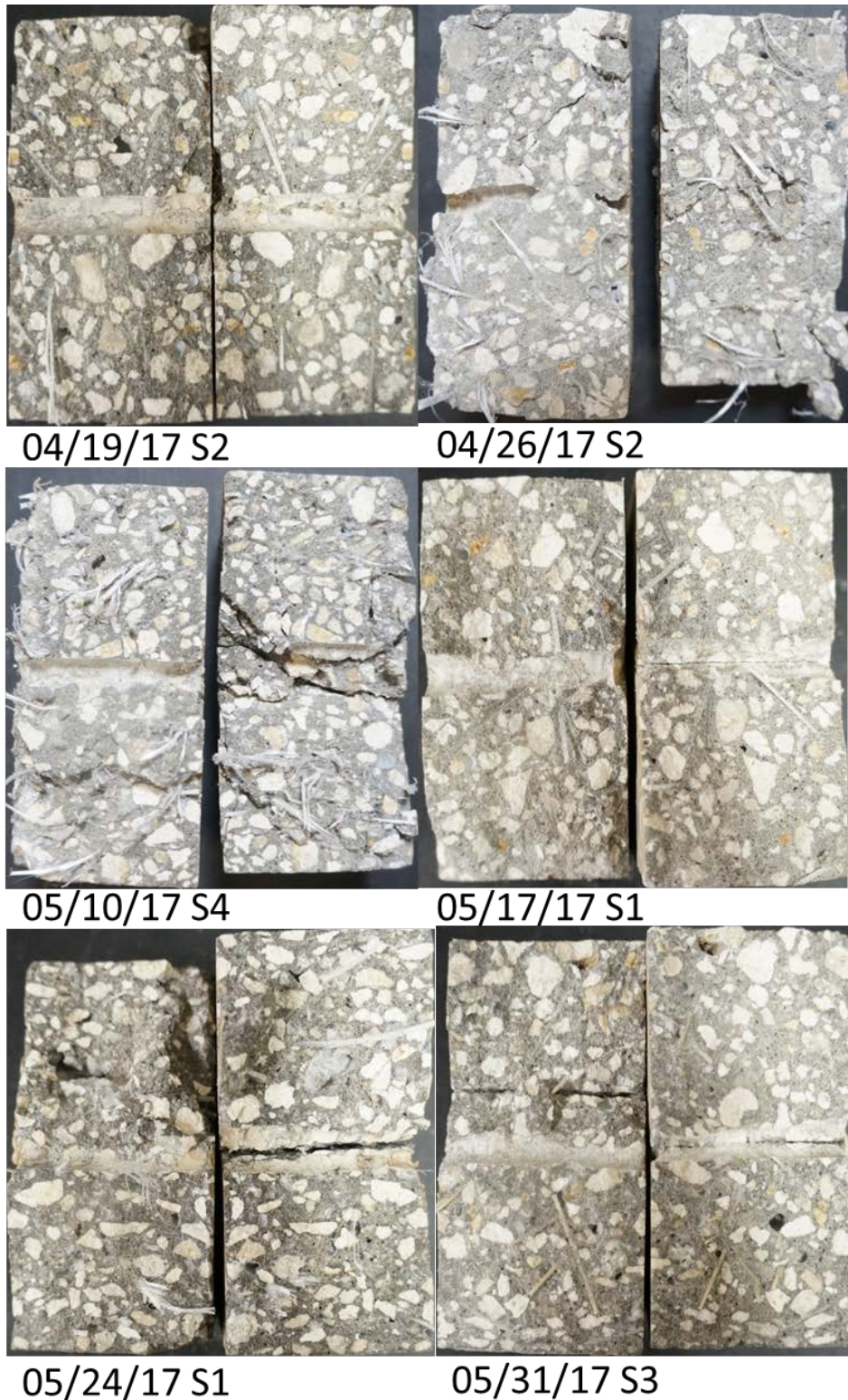
Figure 90. Fiber distribution on 2"-thick specimens exposed at the barge
