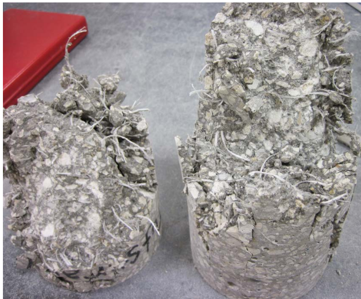
Figure 59. HH mix 2 sample after hammering.
