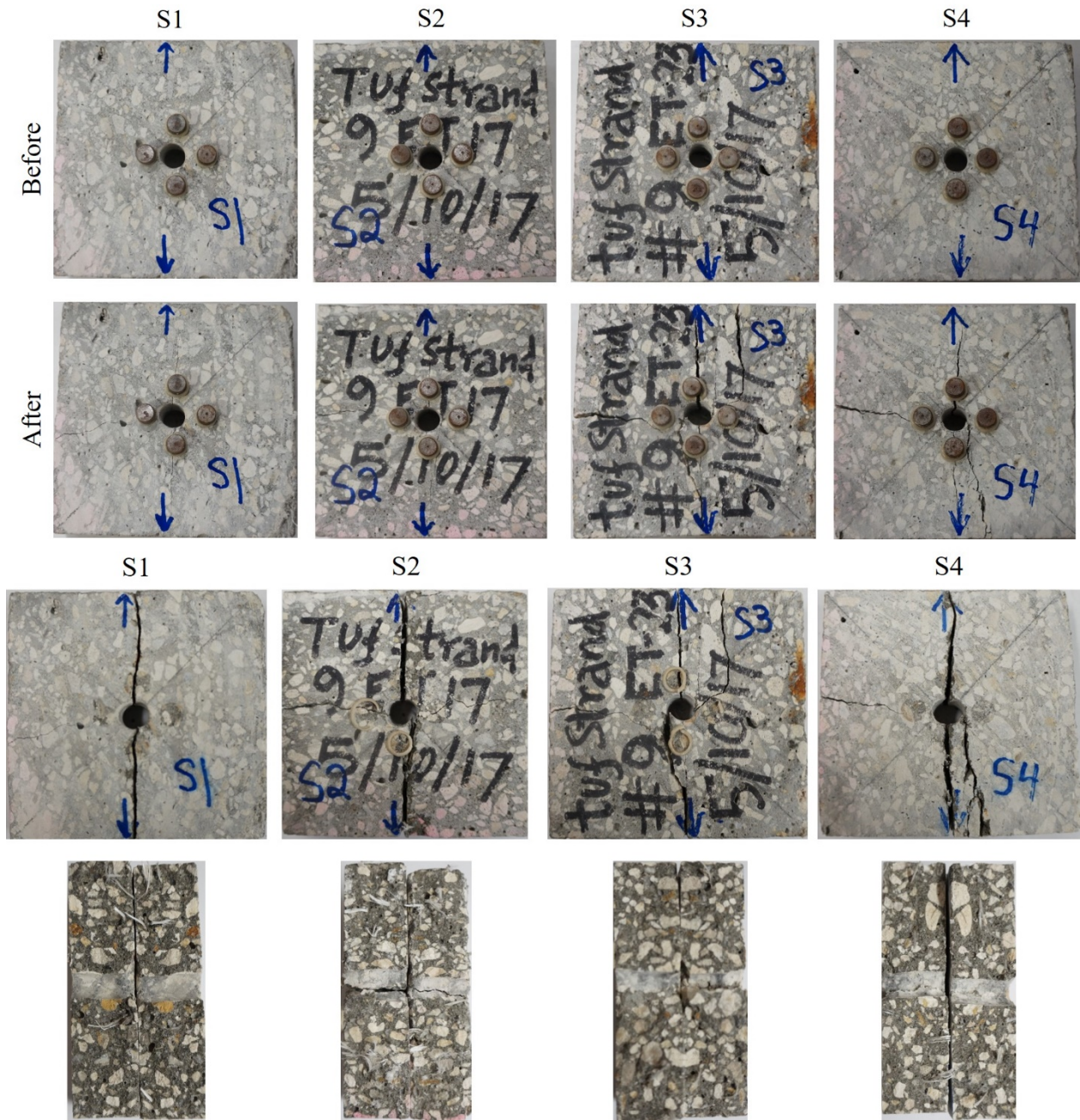
Figure 219. Visual inspection samples of mix 3 exposed in high humidity
