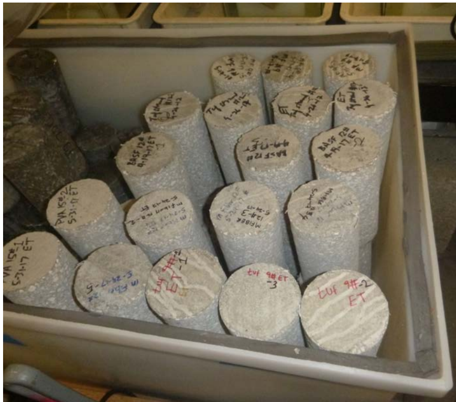
Figure 17. Cores while exposed in a high humidity environment.
