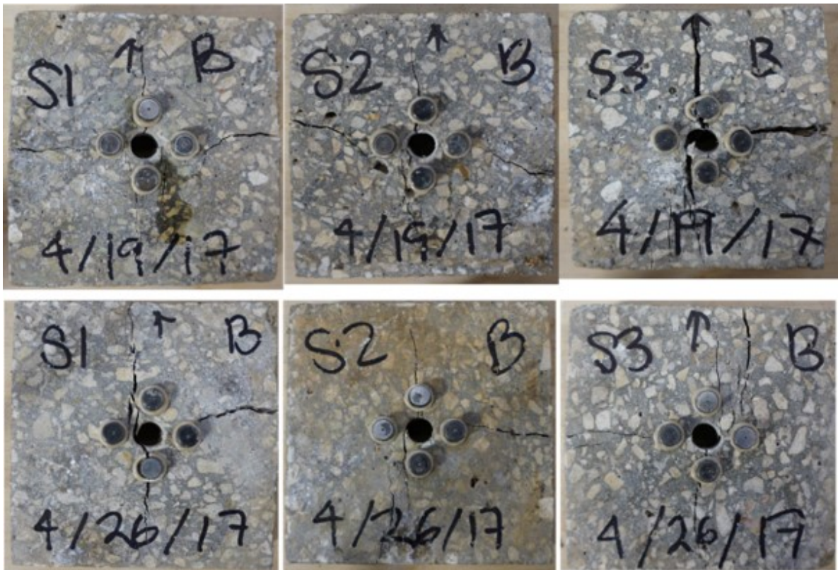
Figure 87. Mix 1 (top row) and mix 2 (bottom row) samples after modified IDT testing (immersed in intercoastal waters)
