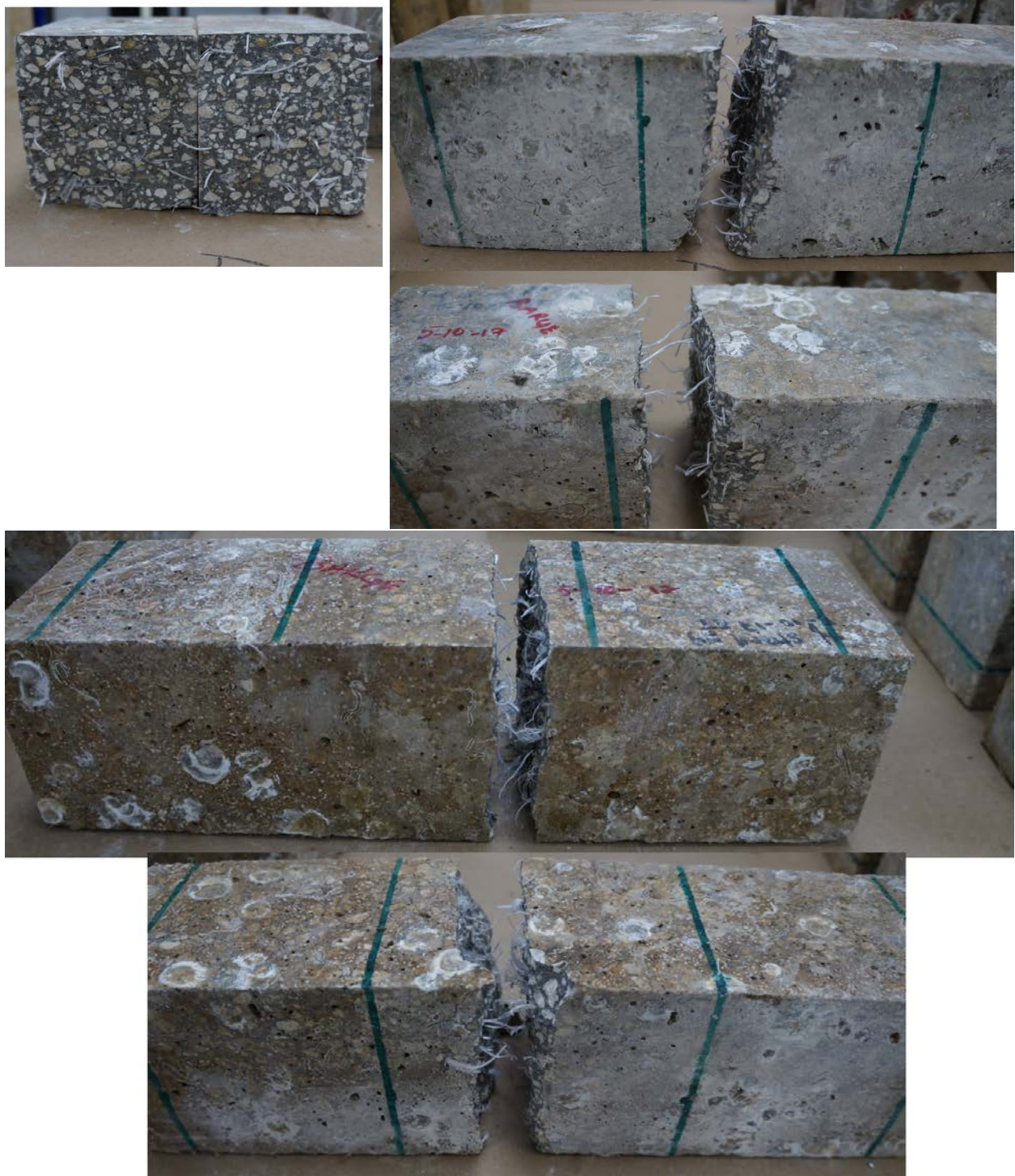
Figure 155. Fiber distribution after residual strength tests on beams of mix 3
