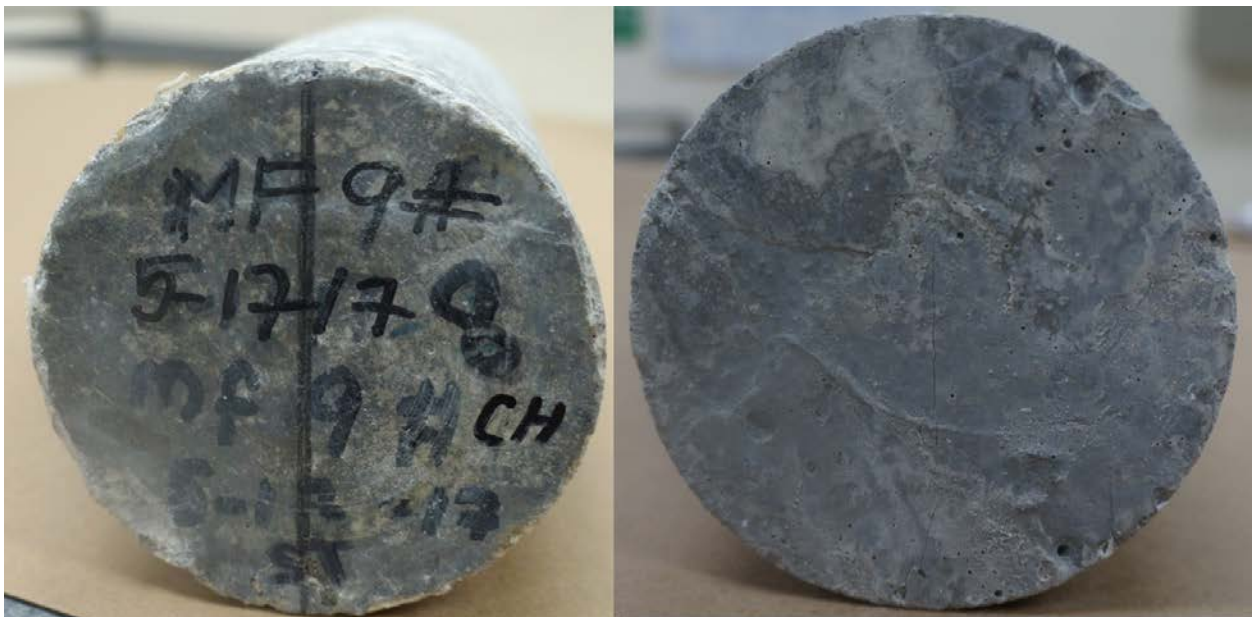
Figure 62. CH mix 4 (5/17/17) samples after performing split test. Both core ends are shown.
