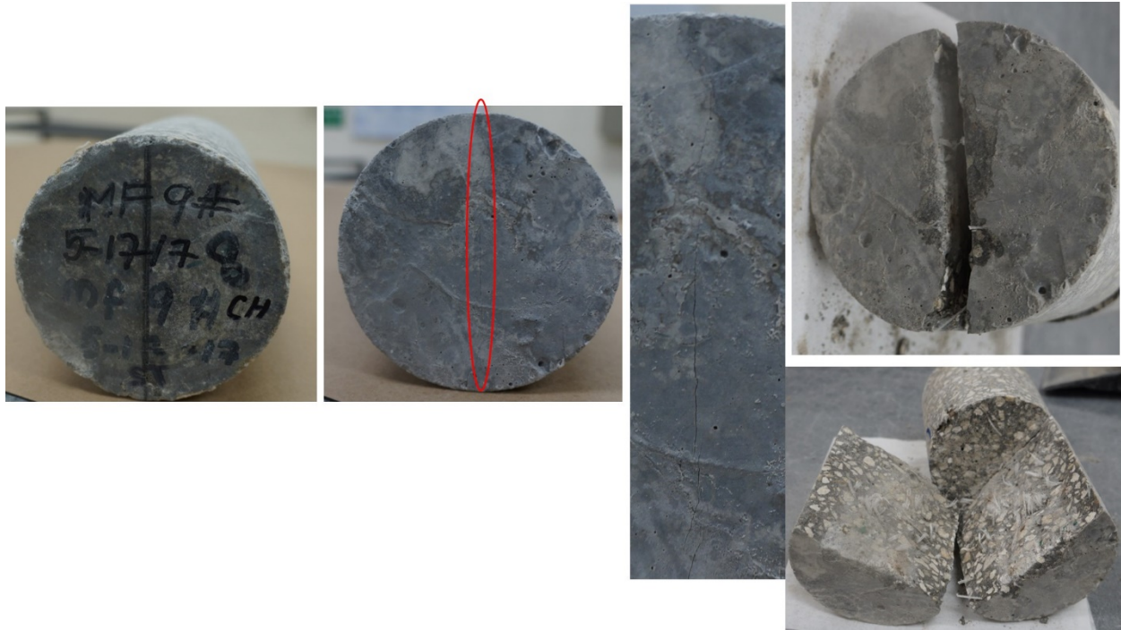
Figure 138. Visual inspection after split-tensile tests on cores of mix 3
