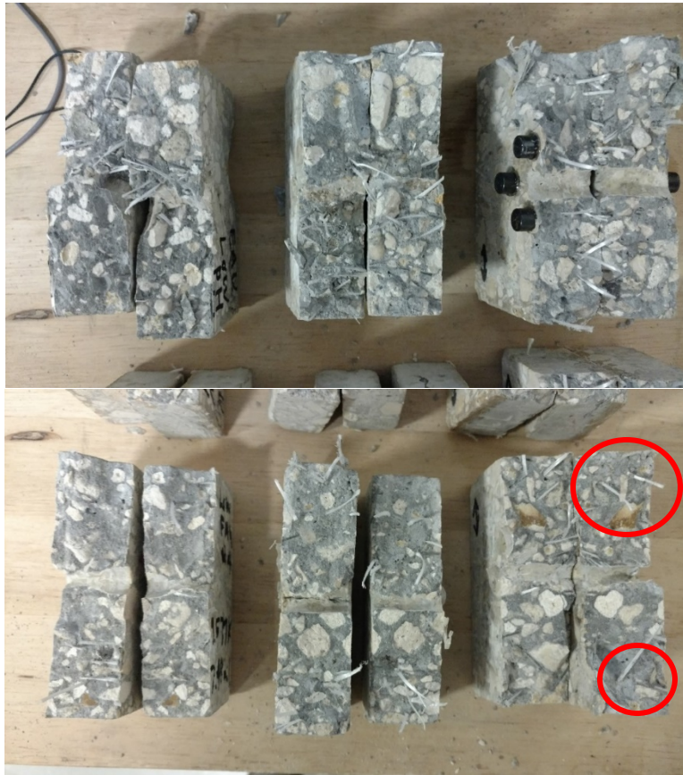
Figure 84. Modified IDT samples subjected to low pH.
