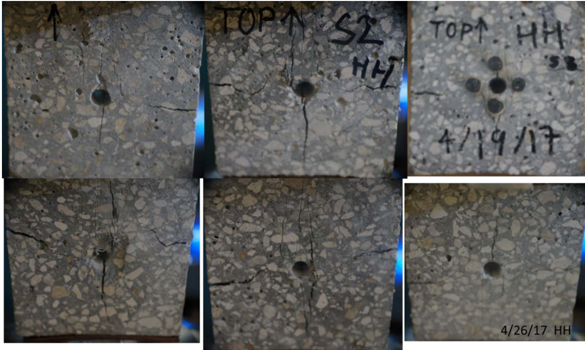
Figure 86. Mix 1 (top row) and mix 2 (bottom row) samples after modified IDT testing (high humidity)
