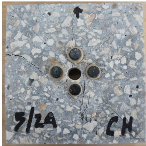
Figure 183. Visual inspection after modified IDT on mix 4 sample (CH)
