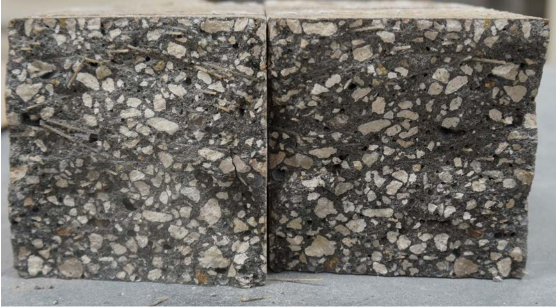
Figure 76. Mix 6 beam after residual strength test (exposed immersed in intercoastal waters)
