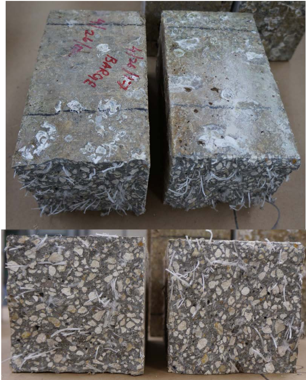
Figure 68. Mix 2 beam after residual strength test (immersed in intercoastal waters).
