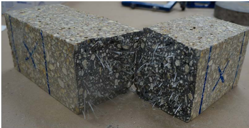
Figure 73. Carbonation depth on mix 4 sample (SW-LpH) after residual strength test.
