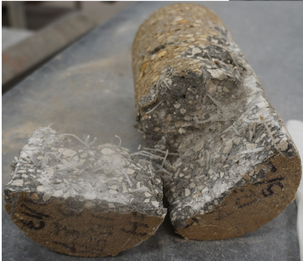
Figure 144. Visual inspection after split-tensile tests on cores of mix 5
