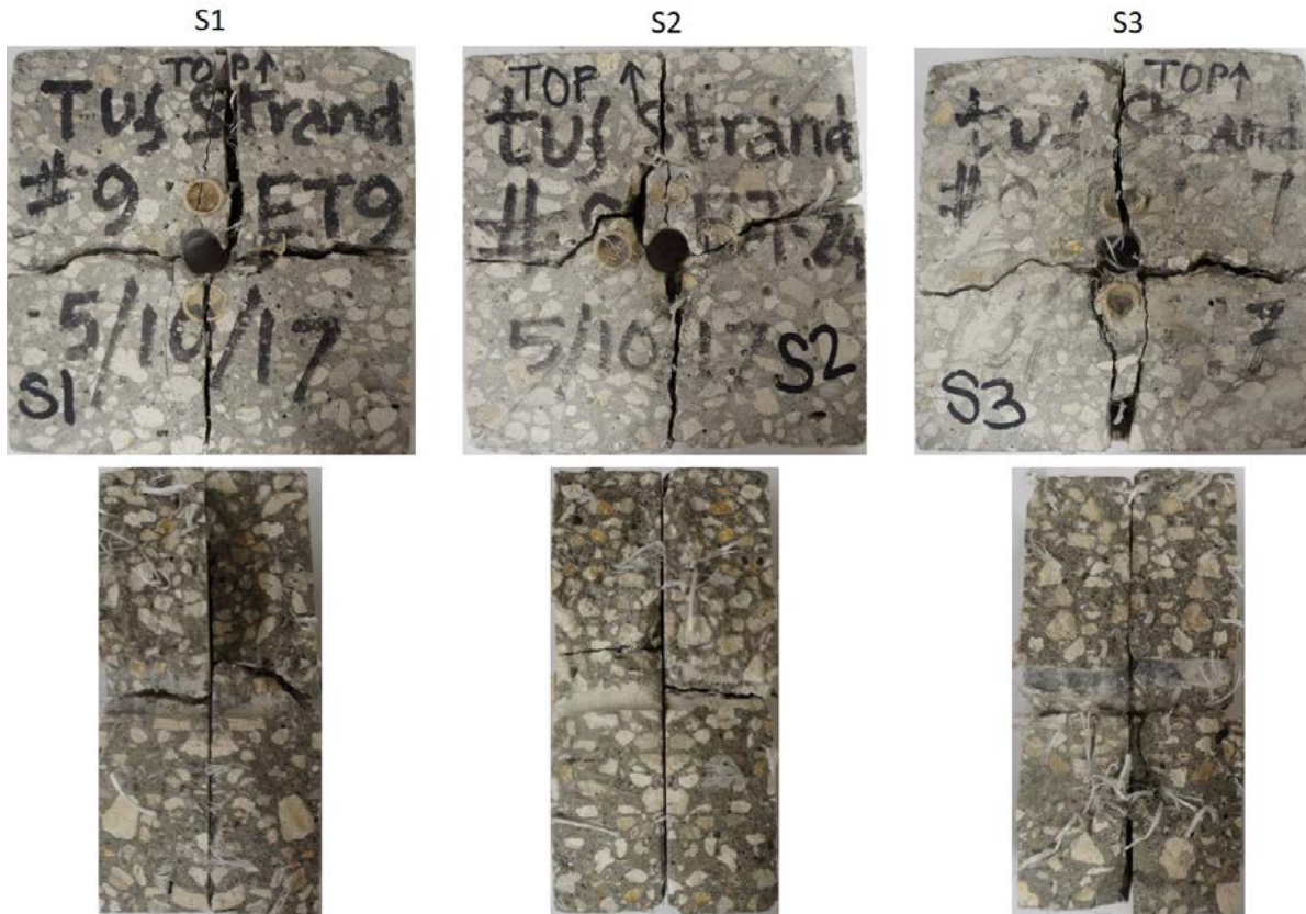
Figure 175. Visual inspection after modified IDT on mix 3 samples (HH)
