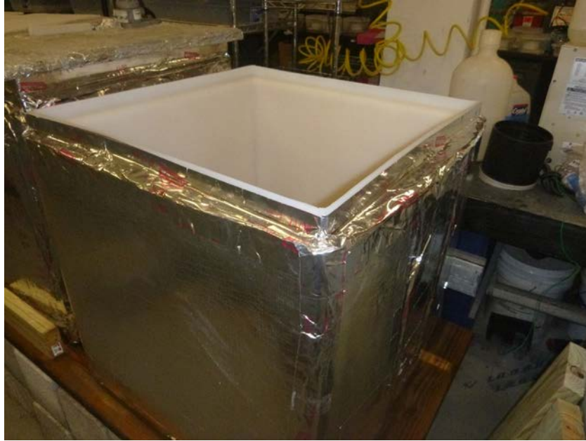
Figure 15. 24" × 24" × 24" container with the insulation installed.
