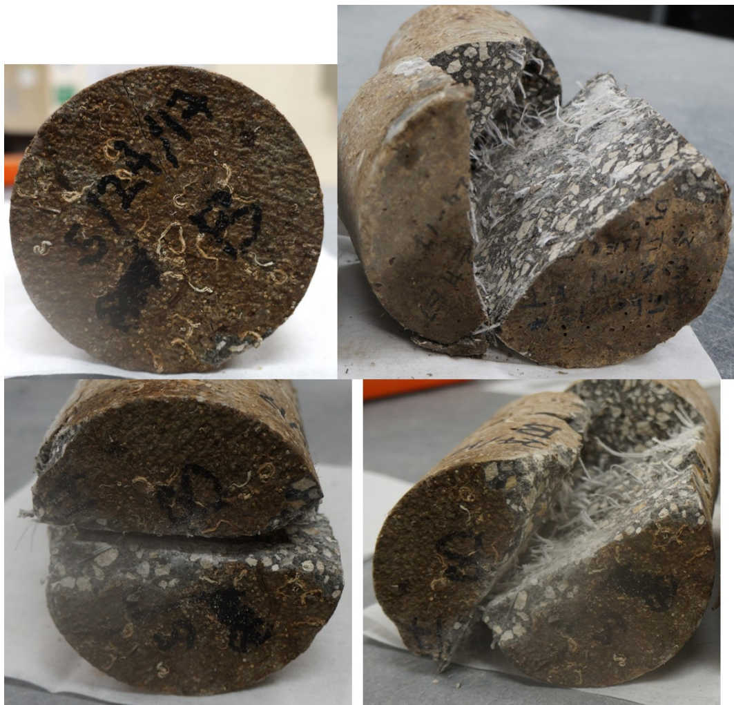
Figure 142. Visual inspection after split-tensile tests on cores of mix 5
