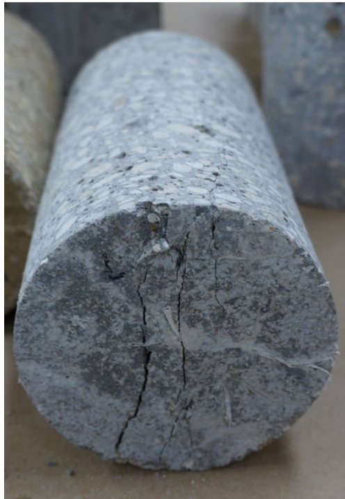
Figure 136. Visual inspection after split-tensile tests on cores of mix 2
