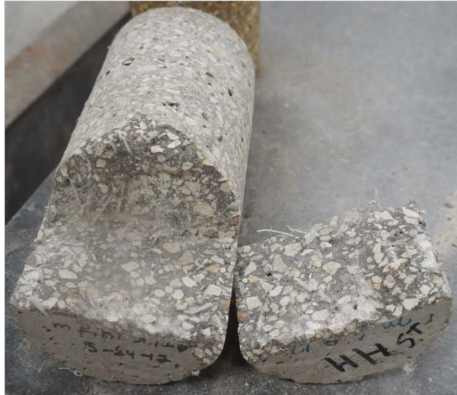
Figure 143. Visual inspection after split-tensile tests on cores of mix 5
