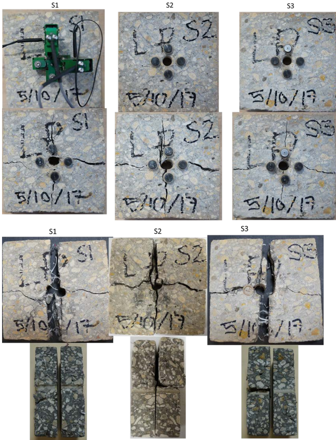
Figure 194. Visual inspection after modified IDT on mix 3 samples (SW_LpH)
