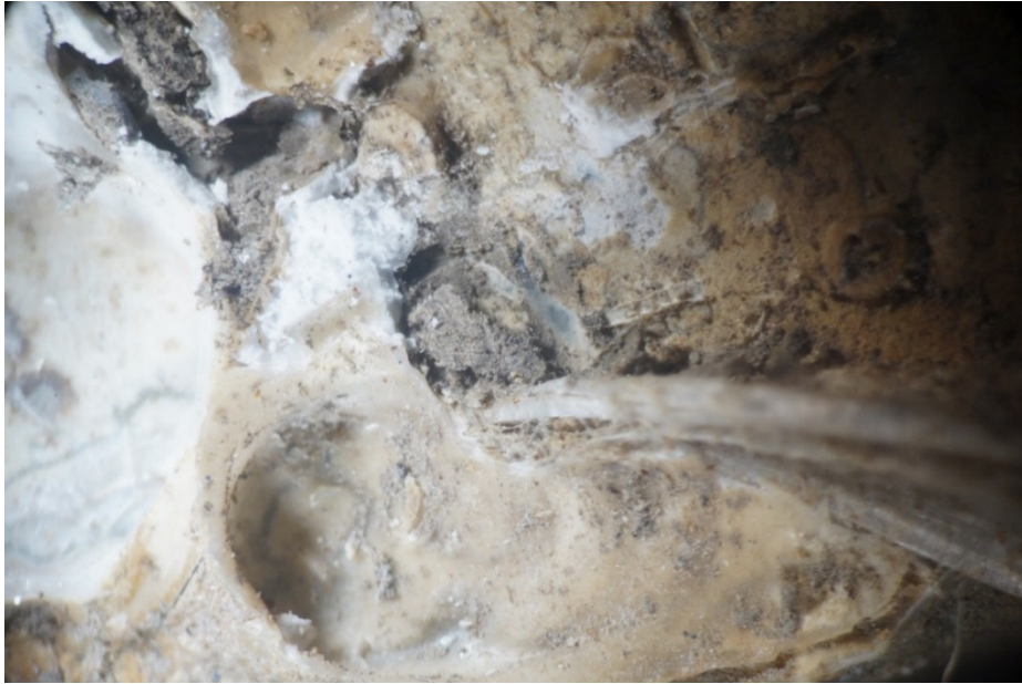
Figure 83. Close-up on fibers and possible marine growth
