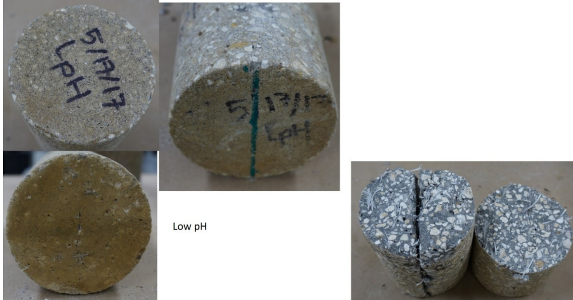
Figure 141. Visual inspection after split-tensile tests on cores of mix 4
