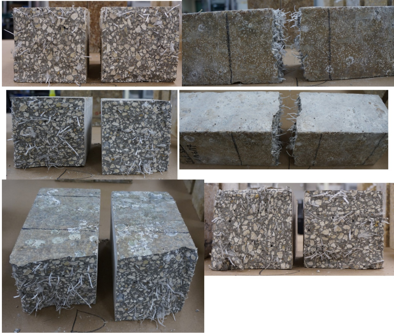
Figure 150. Fiber distribution after residual strength tests on beams of mix 2
