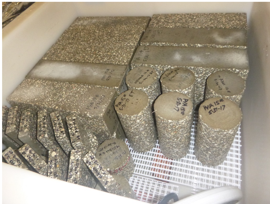
Figure 24. Samples exposed in seawater with the solution pH adjusted (dry cycle).
