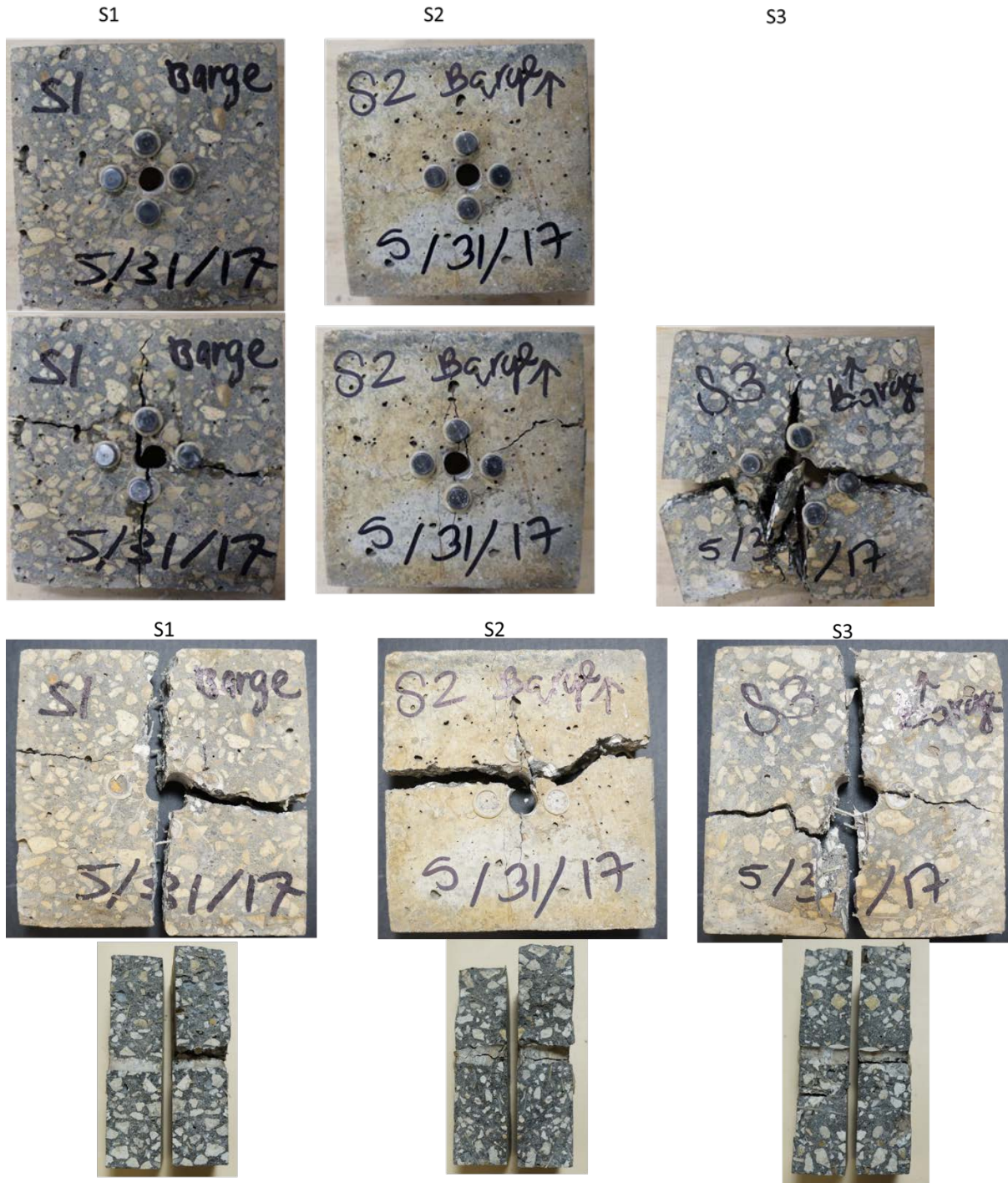
Figure 210. Visual inspection after modified IDT on mix 6 samples (at barge)
