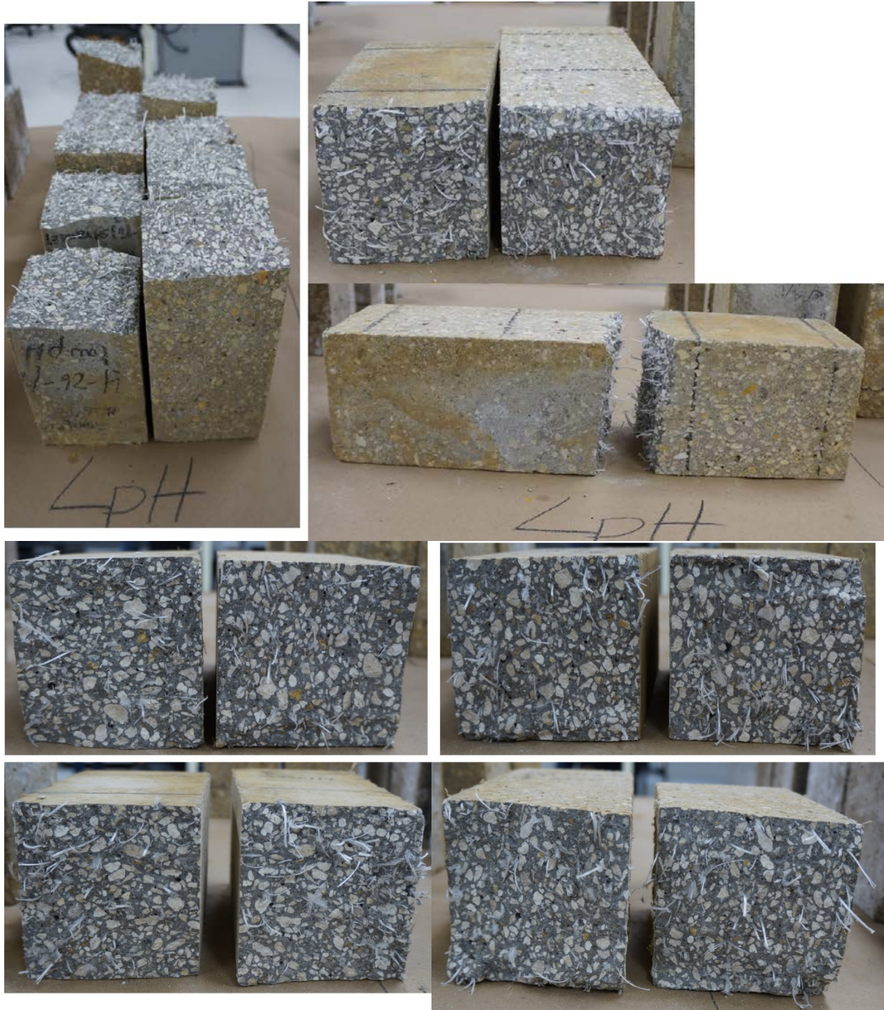
Figure 151. Fiber distribution after residual strength tests on beams of mix 2
