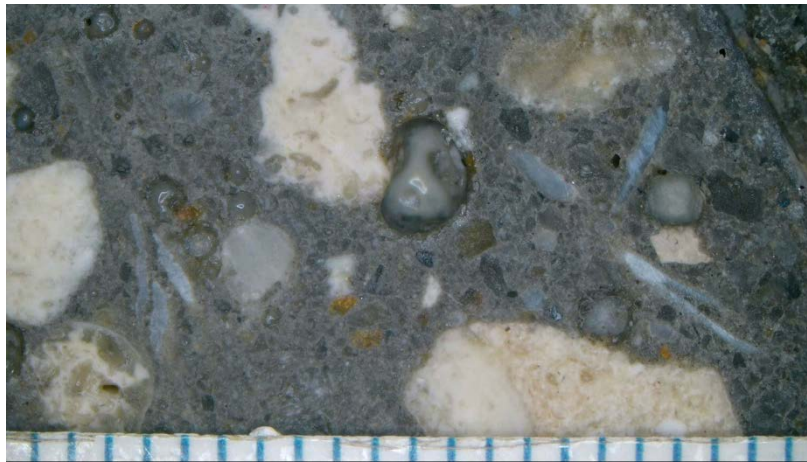
Figure 96. Mix 3 sample. Image showing several fibers in the cut-off surface
