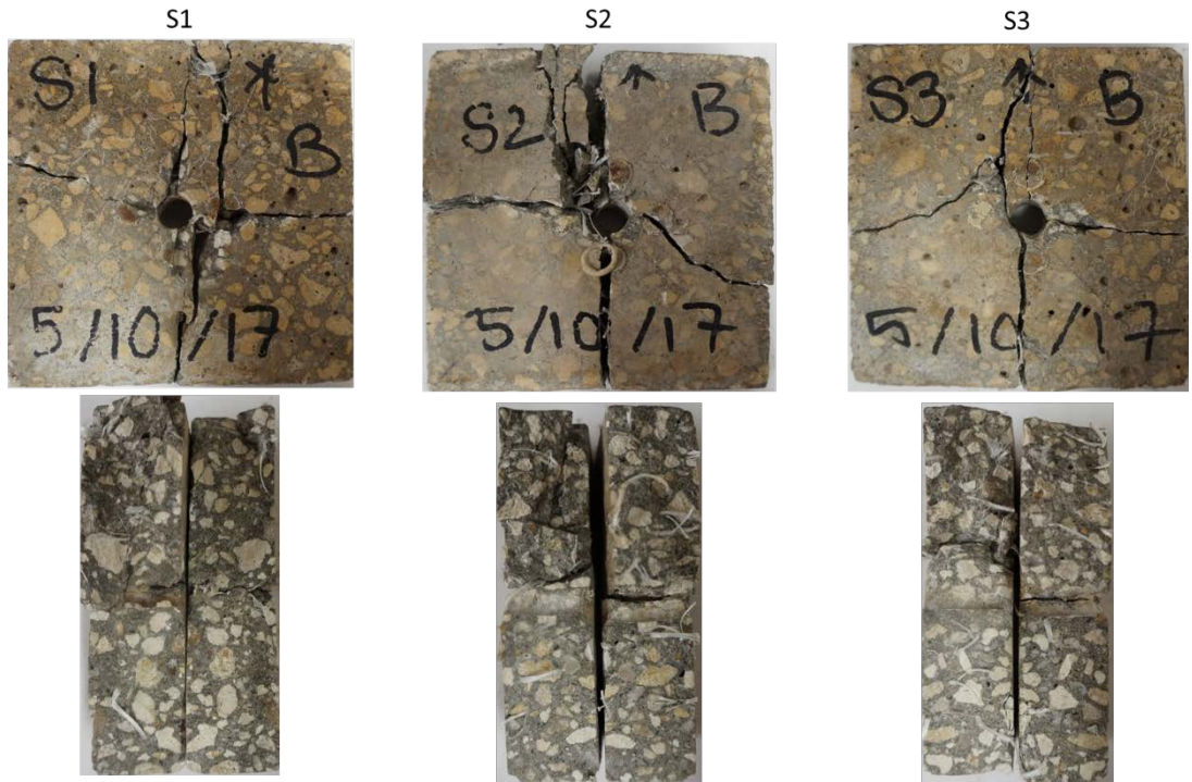
Figure 207. Visual inspection after modified IDT on mix 3 samples (at barge)
