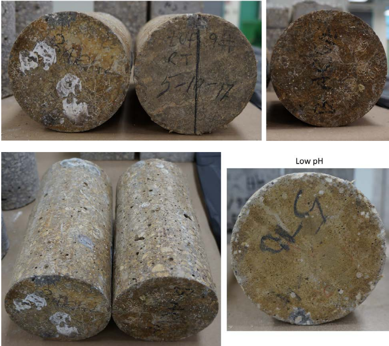
Figure 137. Visual inspection after split-tensile tests on cores of mix 3
