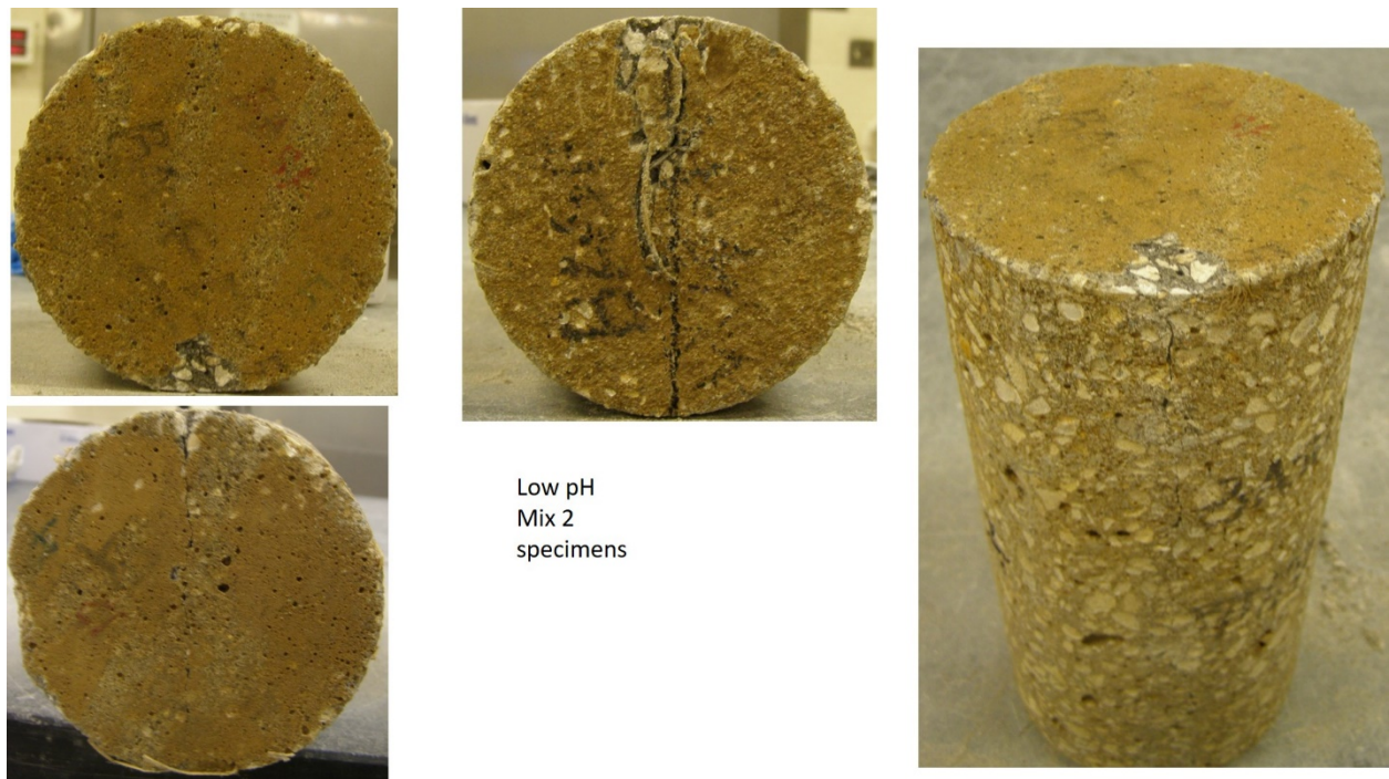
Figure 134. Visual inspection after split-tensile tests on cores of mix 2
