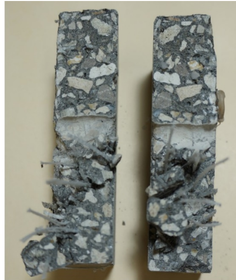
Figure 184. Visual inspection after modified IDT on mix 5 sample (CH)
