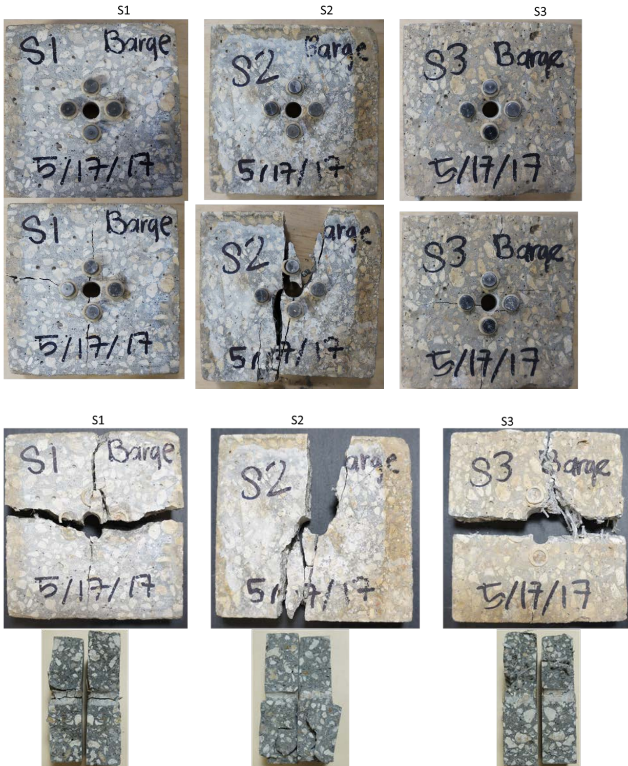
Figure 208. Visual inspection after modified IDT on mix 4 samples (at barge)
