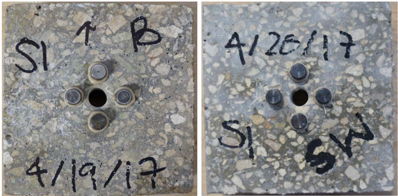
Figure 85. IDT specimens with steel gauges glued prior to testing.
