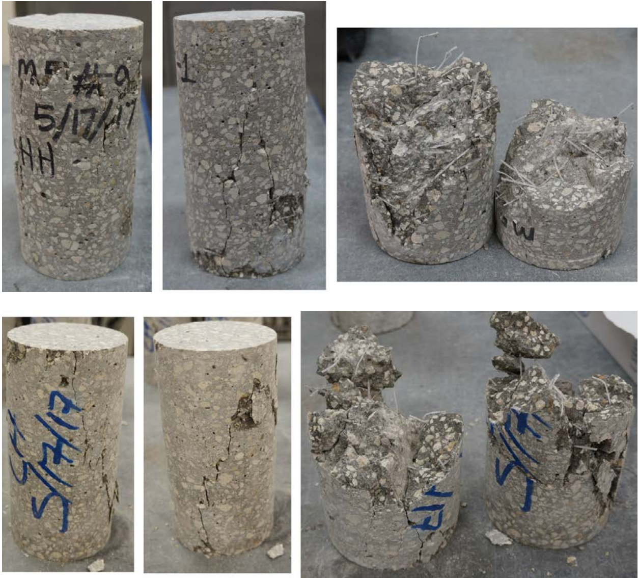
Figure 129. Visual inspection of fiber distribution after compression test on cores of mix 4
