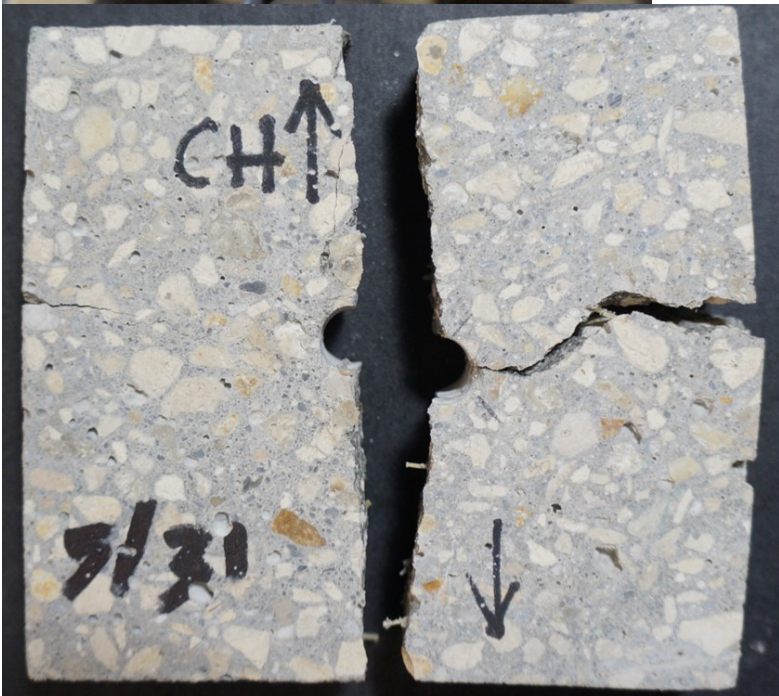
Figure 185. Visual inspection after modified IDT on mix 6 sample (CH)
