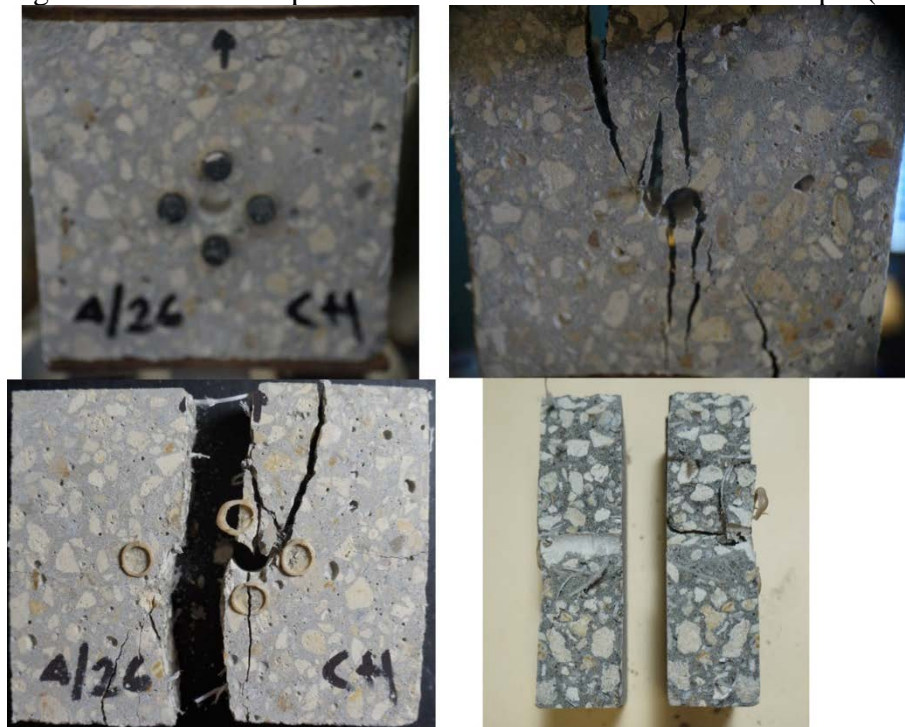
Figure 181. Visual inspection after modified IDT on mix 2 sample (CH)
