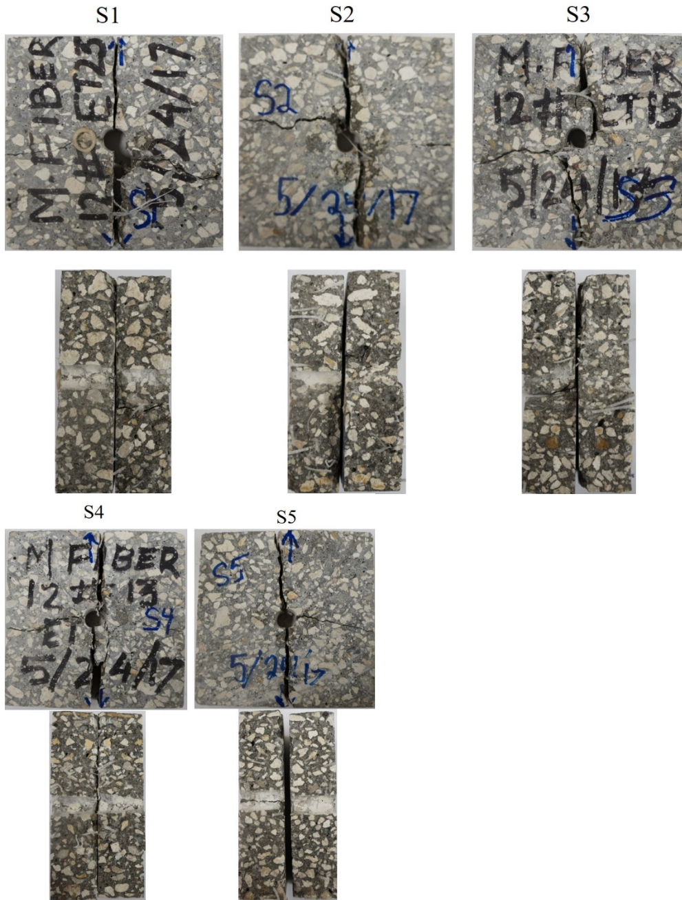
Figure 222. Visual inspection samples of mix 5 exposed in high humidity
