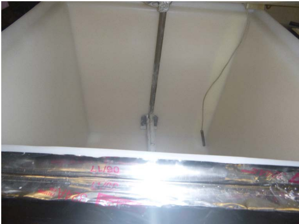
Figure 14. 24" × 24" × 24" showing the heater but before placing solution
