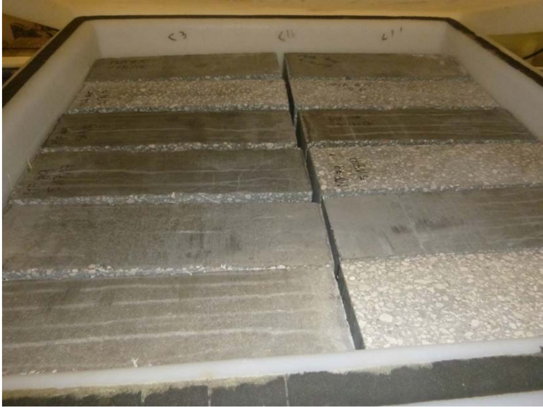
Figure 16. Beams from the different mixes stored in a high humidity environment.
