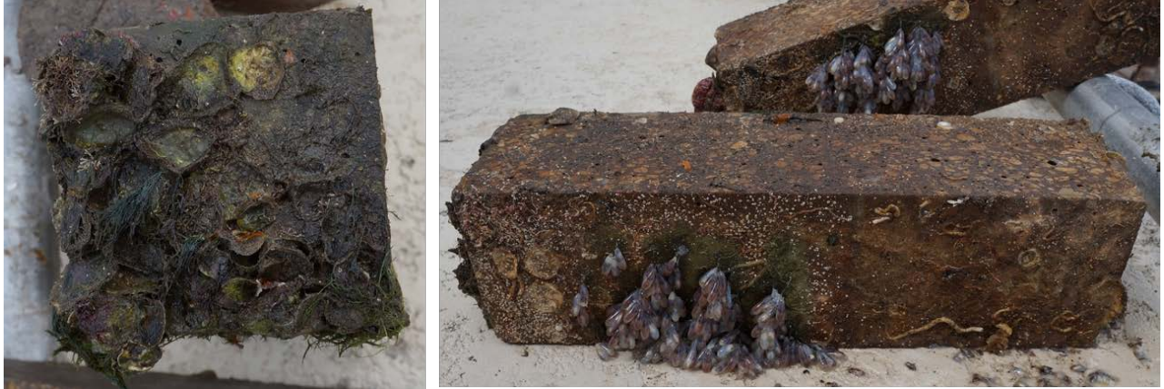
Figure 53. Beams with marine growth.
