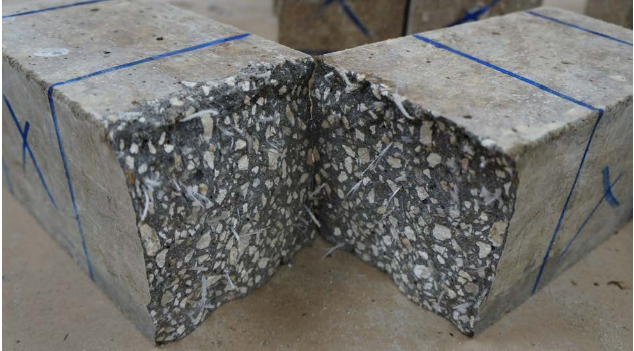
Figure 71. Mix 4 samples after residual strength test (sample exposed at the barge)
