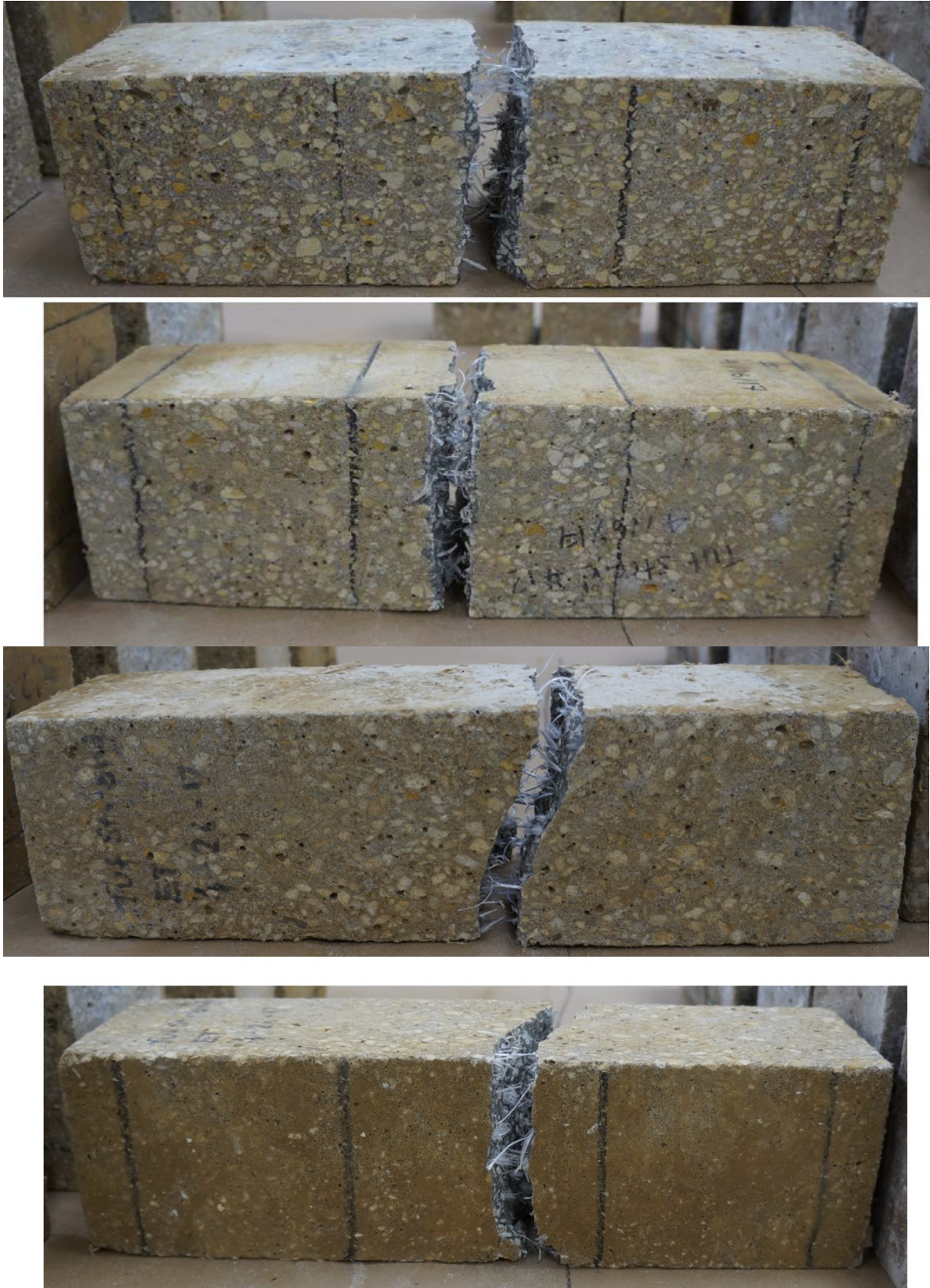
Figure 152. Fiber distribution after residual strength tests on beams of mix 2
