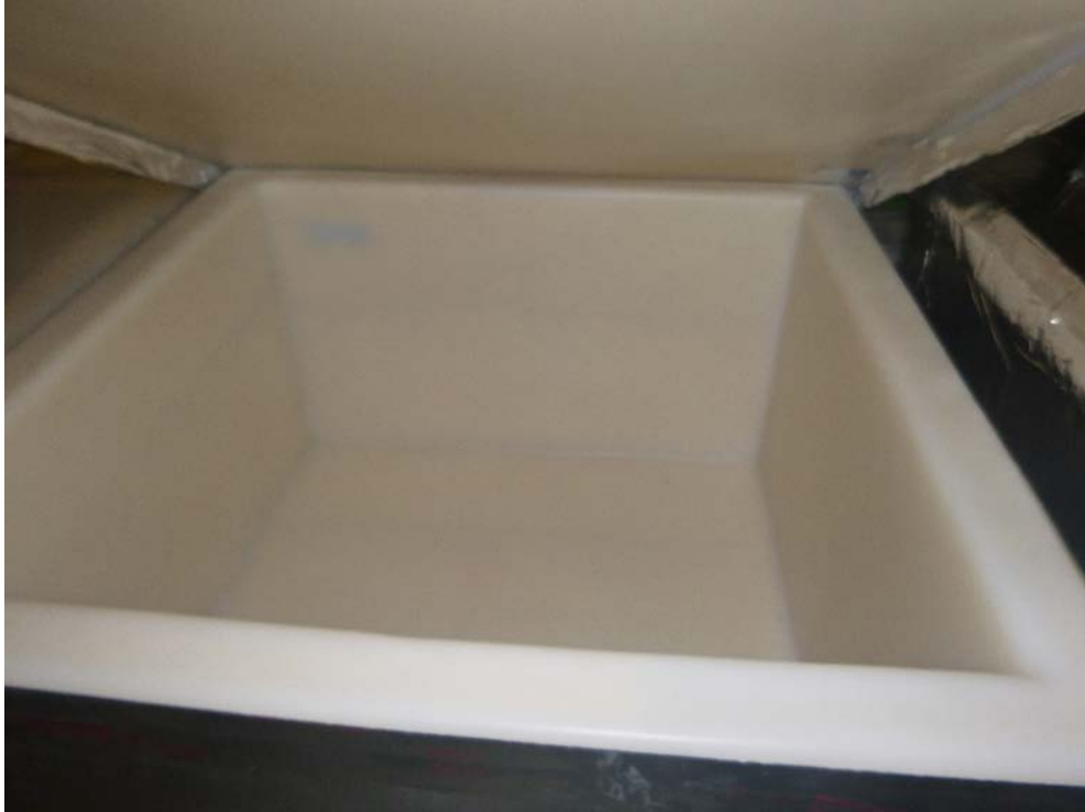
Figure 13. 30" × 30" × 18" container after installing insulation and prior to placing specimens
