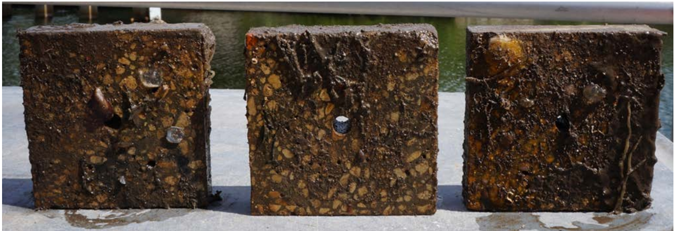
Figure 54. One-inch thick MIDT specimens with marine growth
