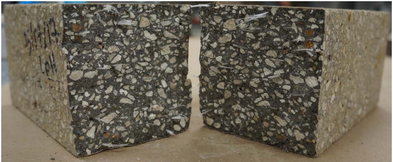
Figure 72. Mix 4 sample (SW-LpH) after residual strength test.
