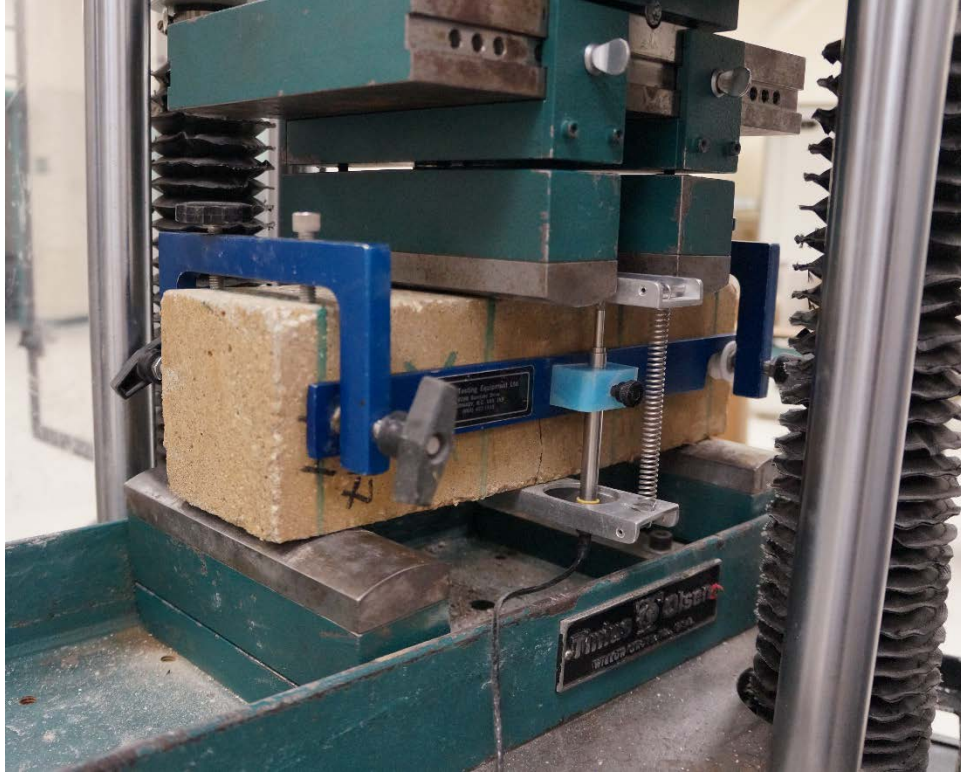
Figure 64. Beam sample being tested for residual strength with LVDTs
