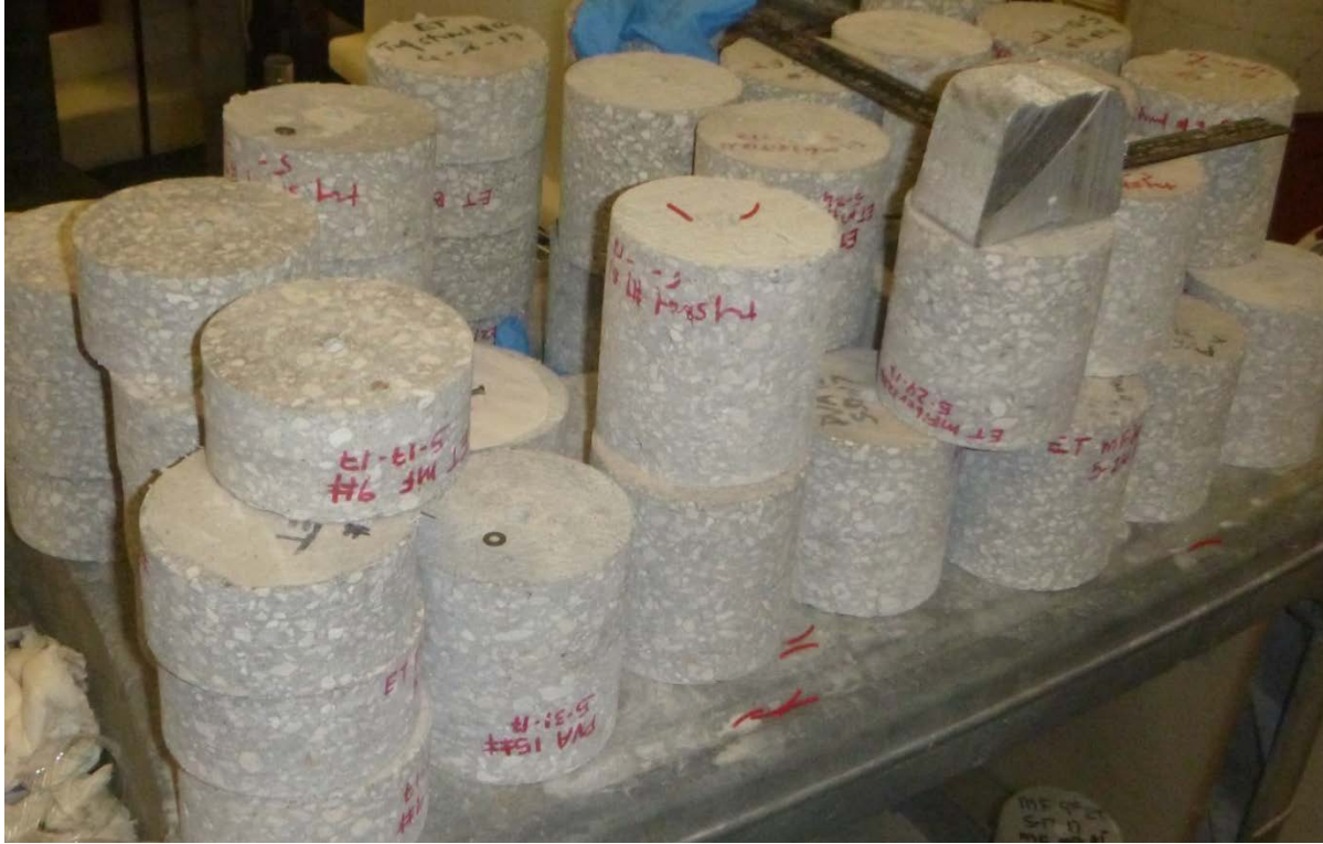
Figure 6. Cut and drilled cylinders to be used after exposure to a modified split tensile test
