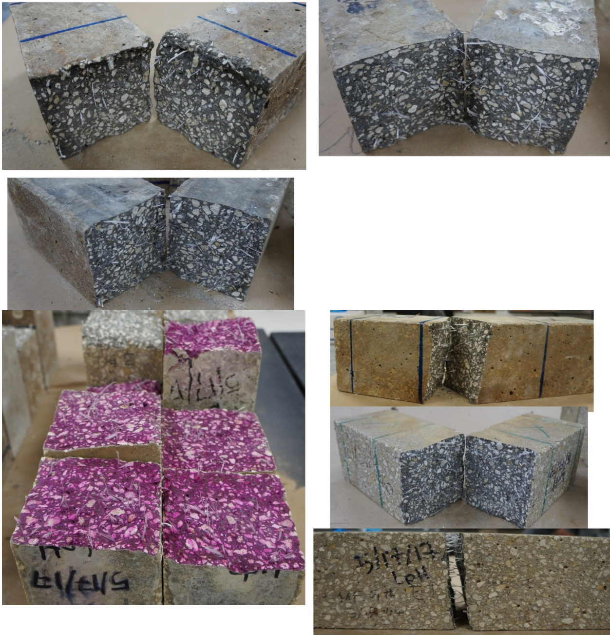
Figure 159. Fiber distribution after residual strength tests on beams of mix 4
