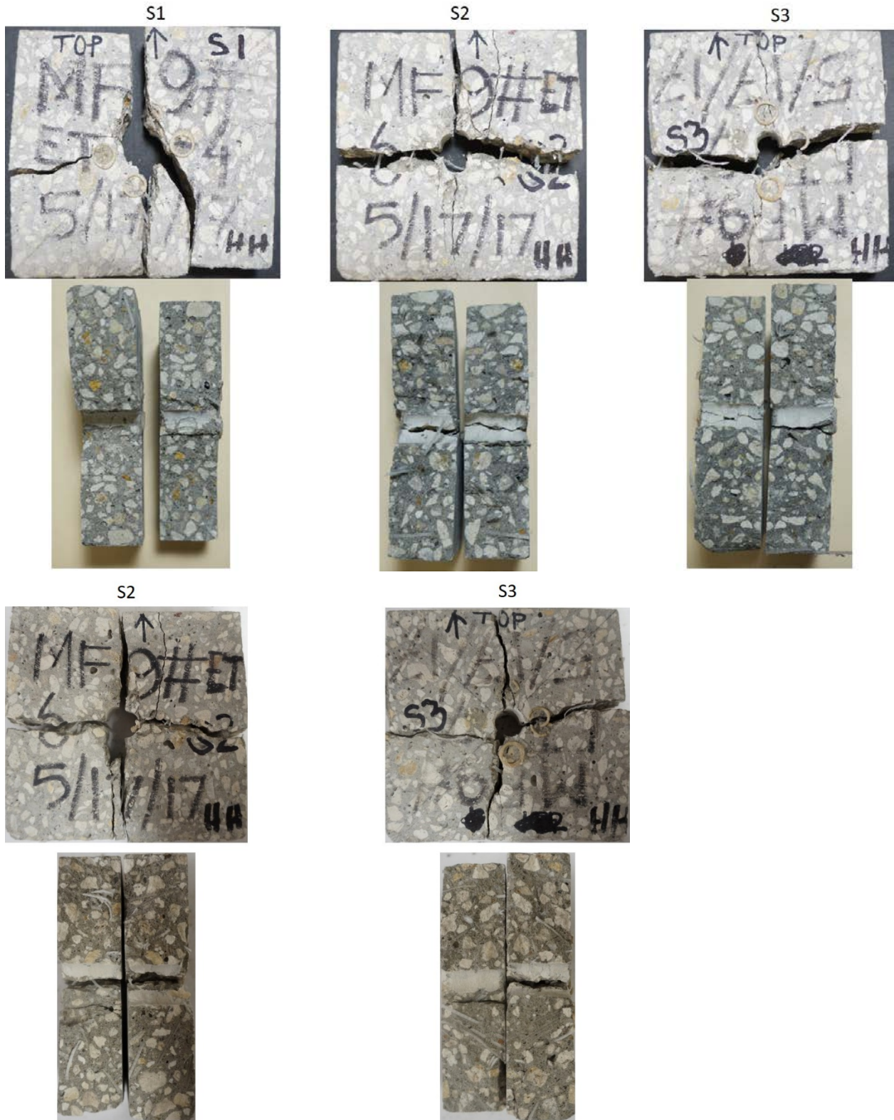
Figure 177. Visual inspection after modified IDT on mix 4 samples (HH)
