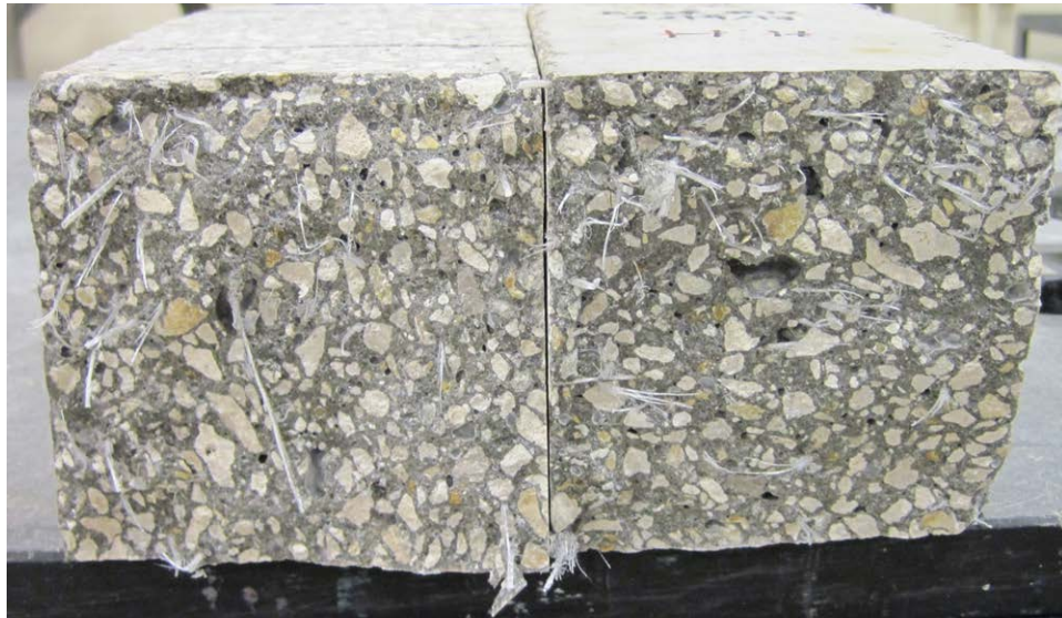
Figure 66. HH mix 1 beam after residual strength testing
