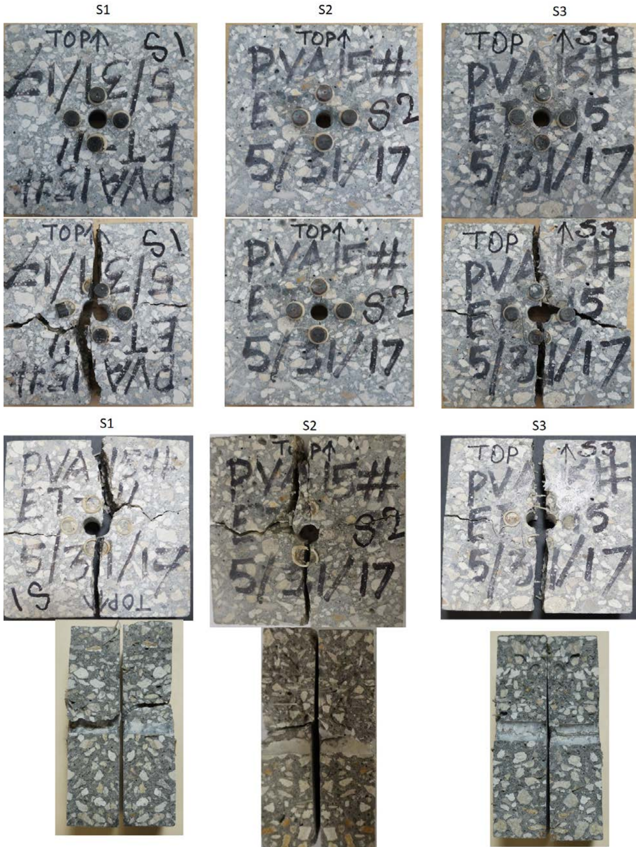
Figure 179. Visual inspection after modified IDT on mix 6 samples (HH)
