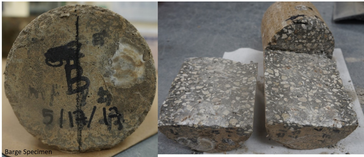
Figure 139. Visual inspection after split-tensile tests on cores of mix 4
