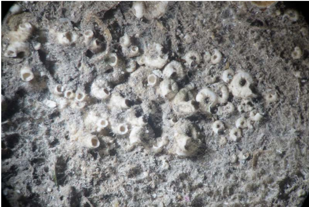
Figure 79. Marine growth observed on the surface of one of the samples.
