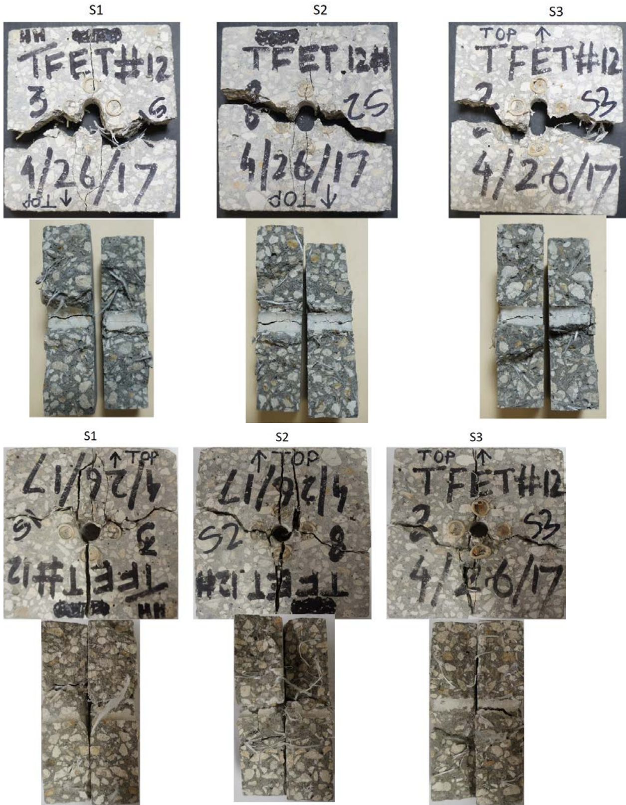
Figure 173. Visual inspection after modified IDT on mix 2 samples (HH)
