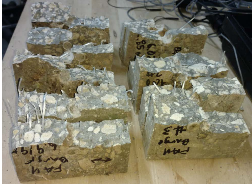
Figure 81. Barge specimens, showing fiber distribution.
