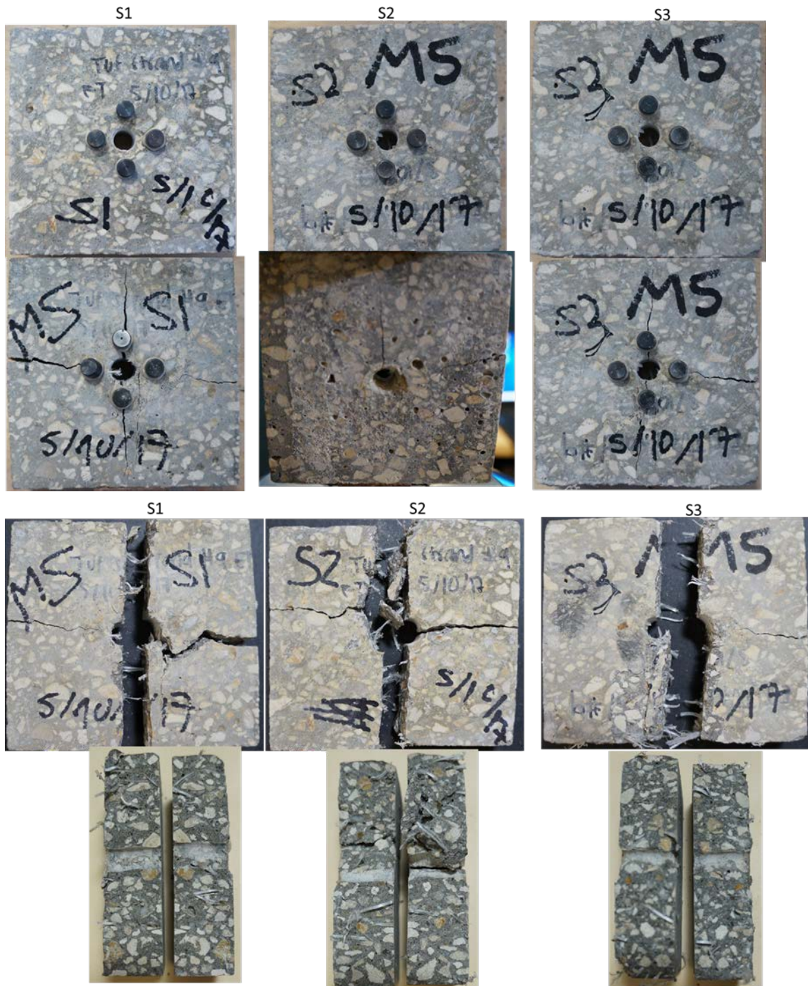
Figure 188. Visual inspection after modified IDT on mix 3 samples (SW)
