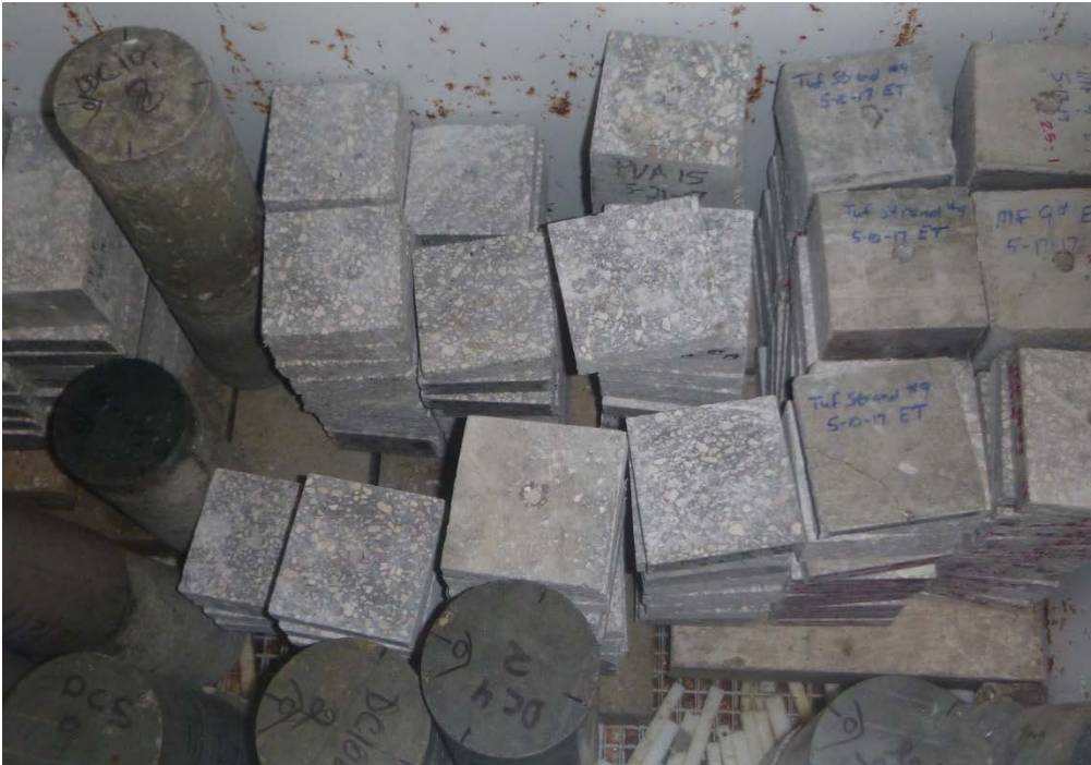
Figure 7. Square cross-section of MIDT samples, with a 10-mm hole drilled at the center.
