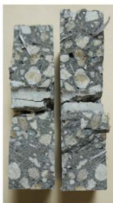
Figure 174. Visual inspection after modified IDT on mix 3 samples (HH)
