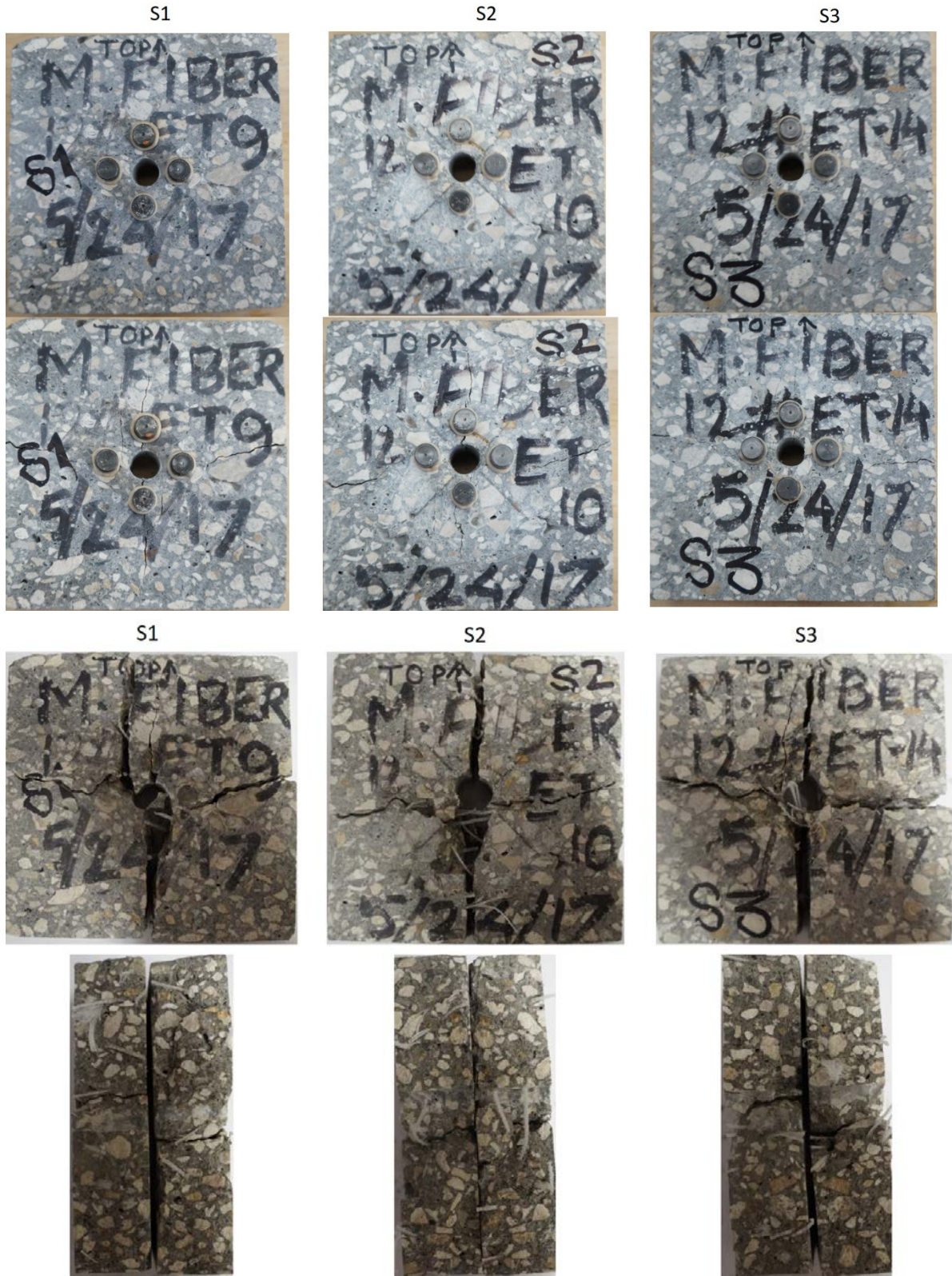
Figure 178. Visual inspection after modified IDT on mix 5 samples (HH)
