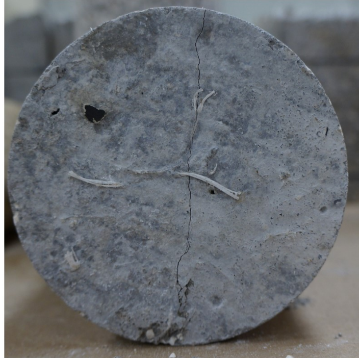
Figure 136. Visual inspection after split-tensile tests on cores of mix 2
