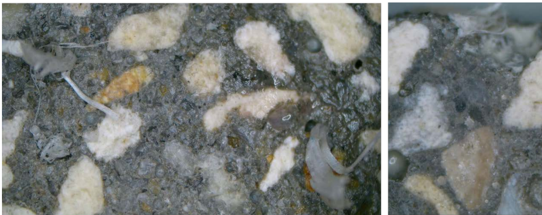
Figure 97. Mix 3 sample, showing fibers that snapped during the IDT testing.
