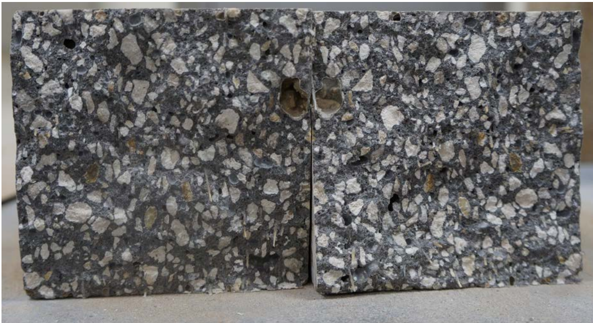
Figure 77. Mix 6 beam after residual strength (exposed immersed in low pH seawater)
