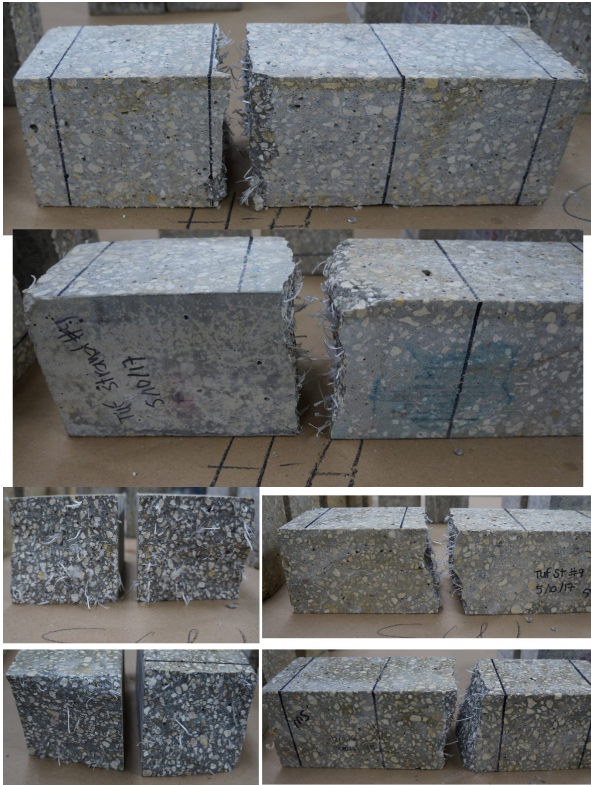
Figure 154. Fiber distribution after residual strength tests on beams of mix 3
