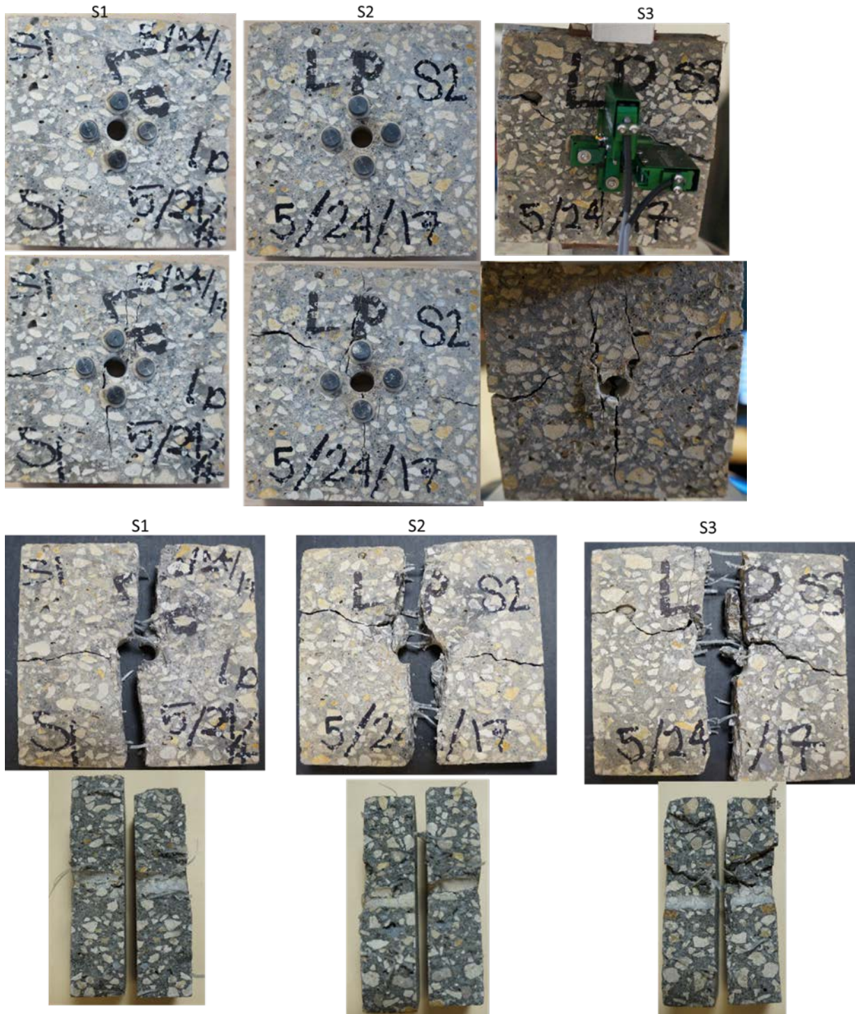
Figure 196. Visual inspection after modified IDT on mix 5 samples (SW_LpH)
