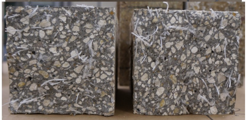
Figure 149. Fiber distribution after residual strength tests on beams of mix 2
