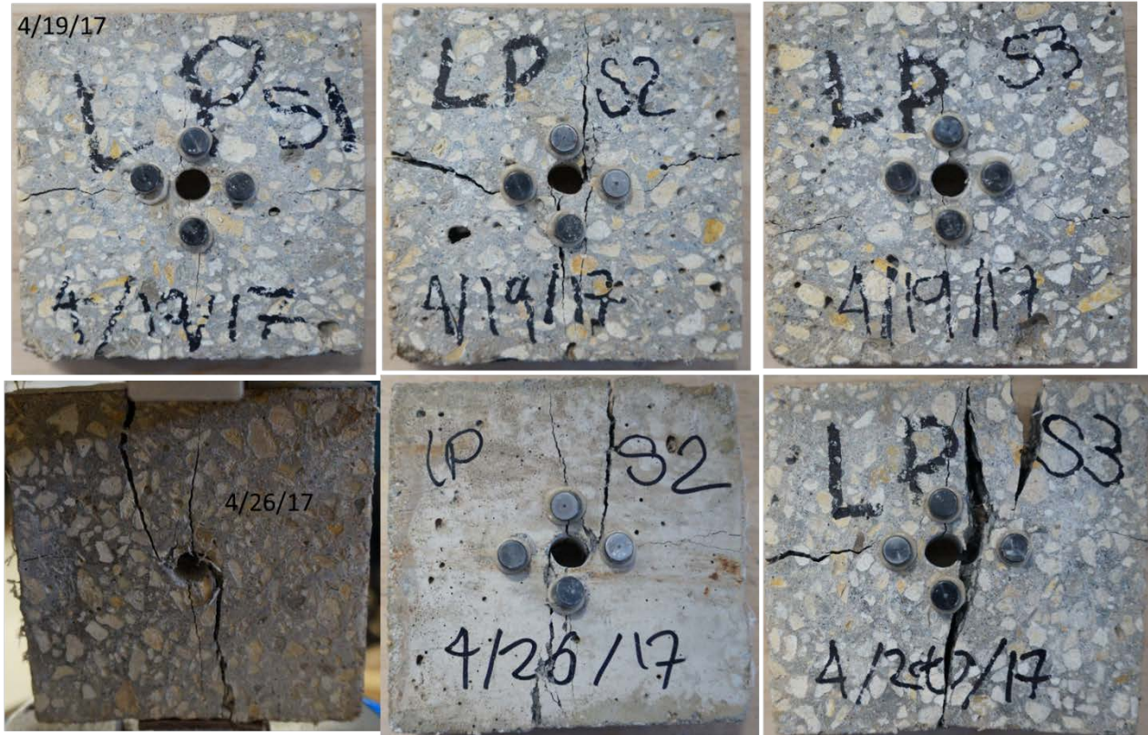
Figure 88. Mix 1 and mix 2 samples after MIDT testing (immersed in seawater low pH)
