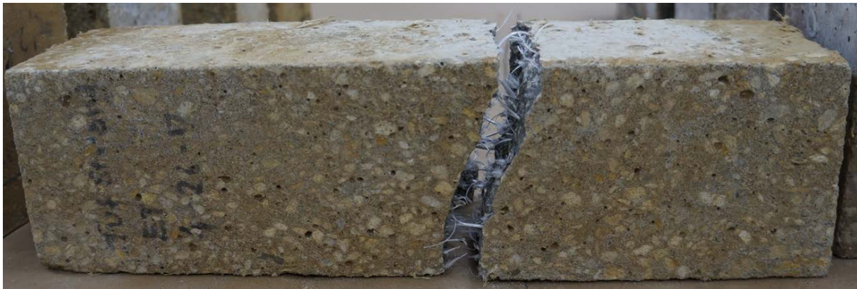
Figure 70. LpH-mix 2 beam after residual strength. Slanted break.
