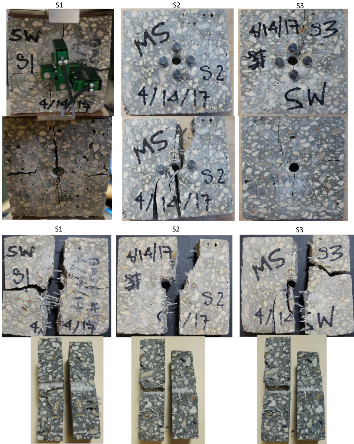
Figure 186. Visual inspection after modified IDT on mix 1 samples (SW)
