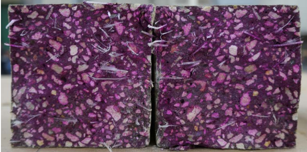
Figure 73. Carbonation depth on mix 4 sample (SW-LpH) after residual strength test.
