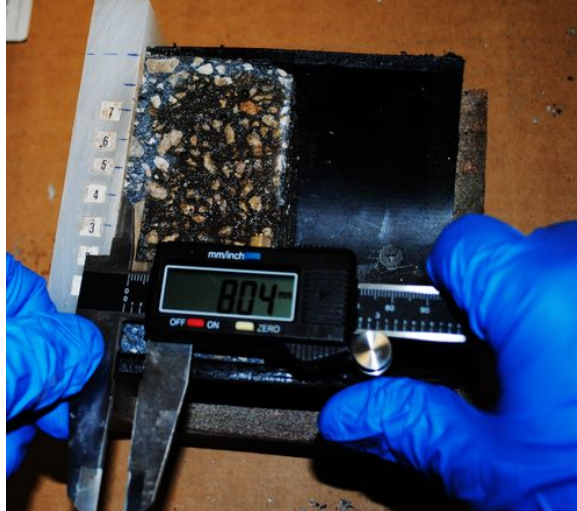
Figure 11. Measurement of chloride ion penetration depth.
