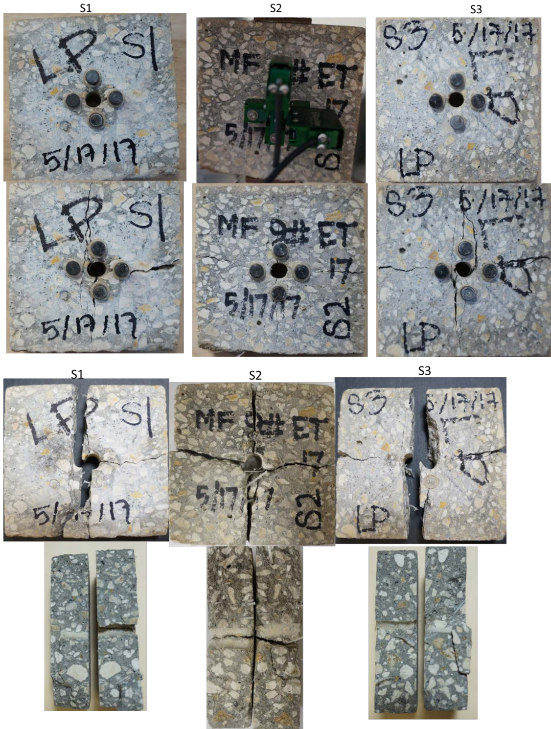
Figure 195. Visual inspection after modified IDT on mix 4 samples (SW_LpH)
