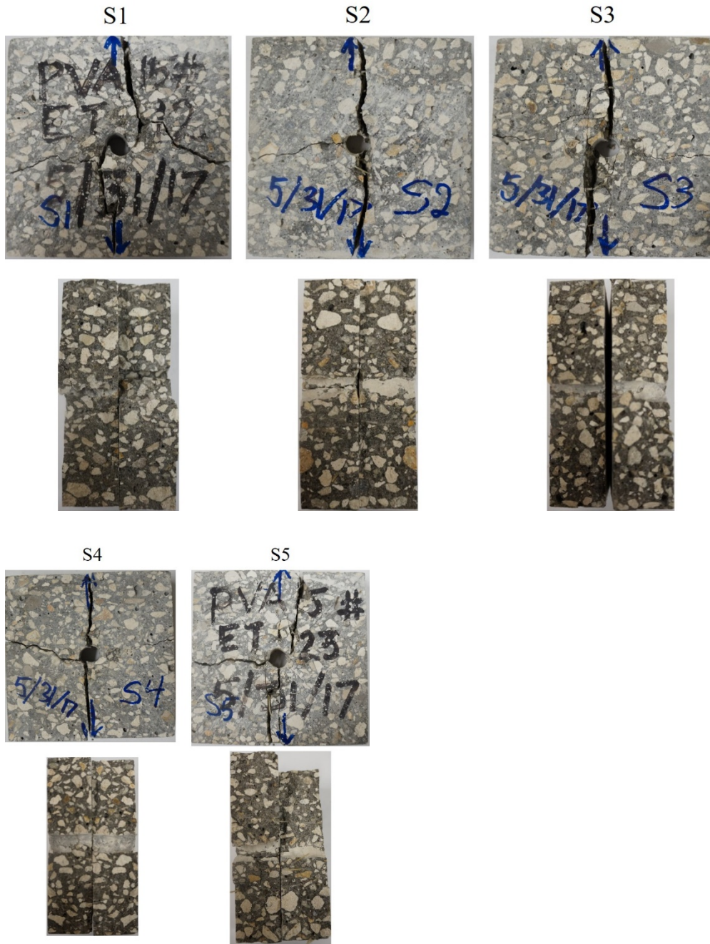
Figure 224. Visual inspection samples of mix 6 exposed in high humidity
