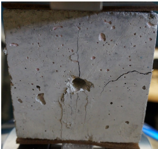
Figure 183. Visual inspection after modified IDT on mix 4 sample (CH)
