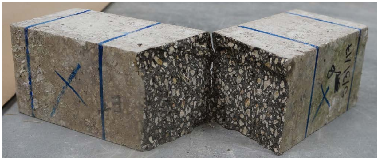
Figure 75. Mix 6 samples after residual strength (exposed immersed in intercoastal waters)
