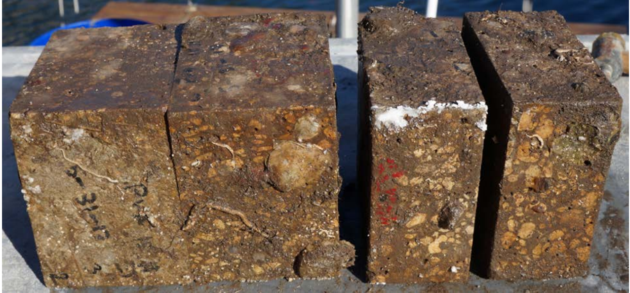
Figure 55. Two- and three-inch-thick MIDT specimens with marine growth
