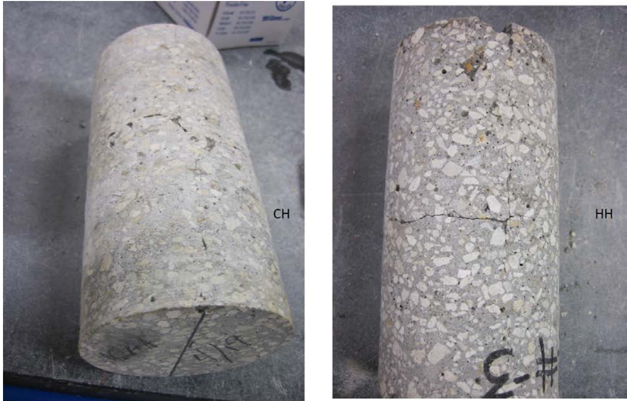
Figure 133. Visual inspection after split-tensile tests on cores of mix 1
