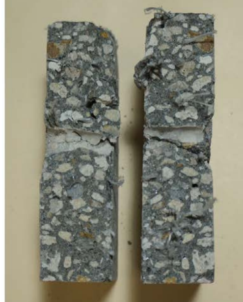
Figure 182. Visual inspection after modified IDT on mix 3 sample (CH)
