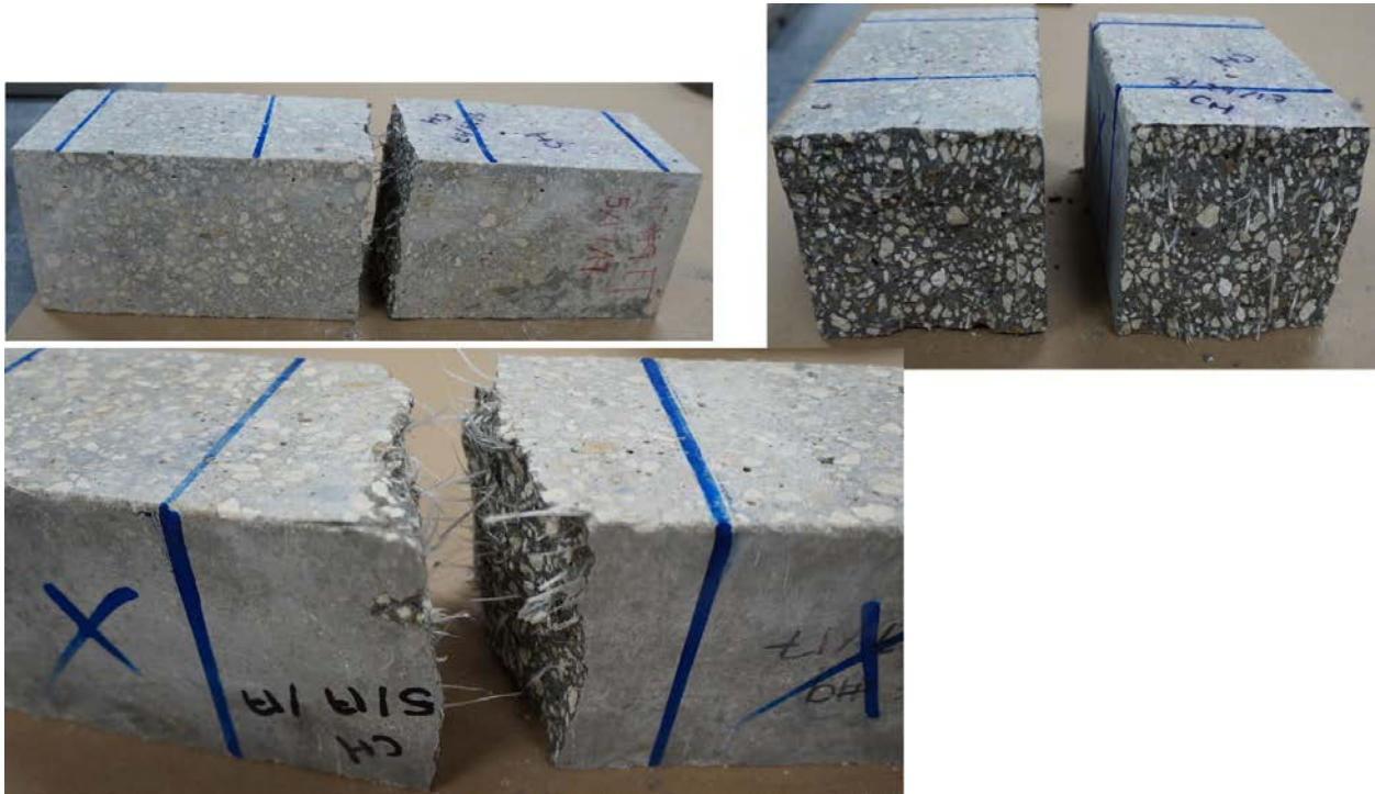
Figure 162. Fiber distribution after residual strength tests on beams of mix 4
