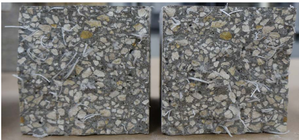
Figure 67. HH mix 2 beam after residual strength testing.
