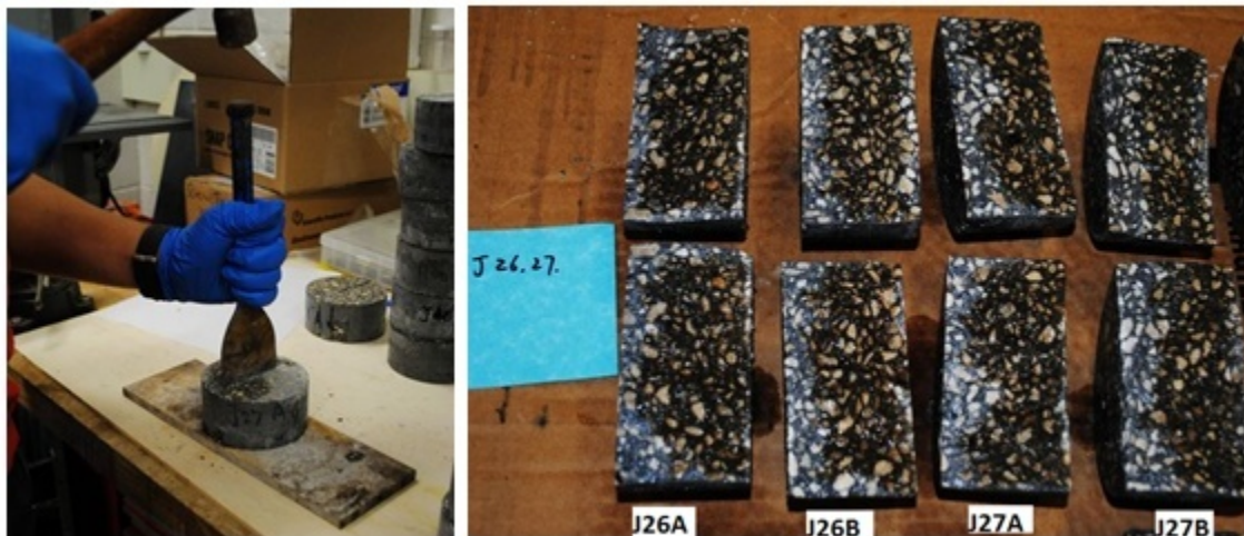
Figure 10. Illustration of splitting slices and spraying 0.1N \text{AgNO}_3 at the cross-section as an indication of chloride ion penetration depth.
