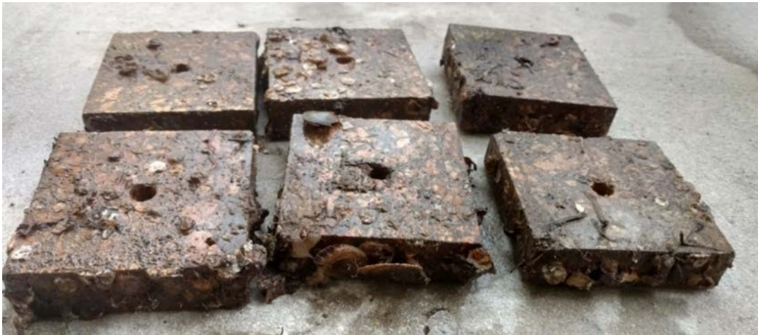
Figure 78. IDT samples exposed at the barge for 18 (check) months
