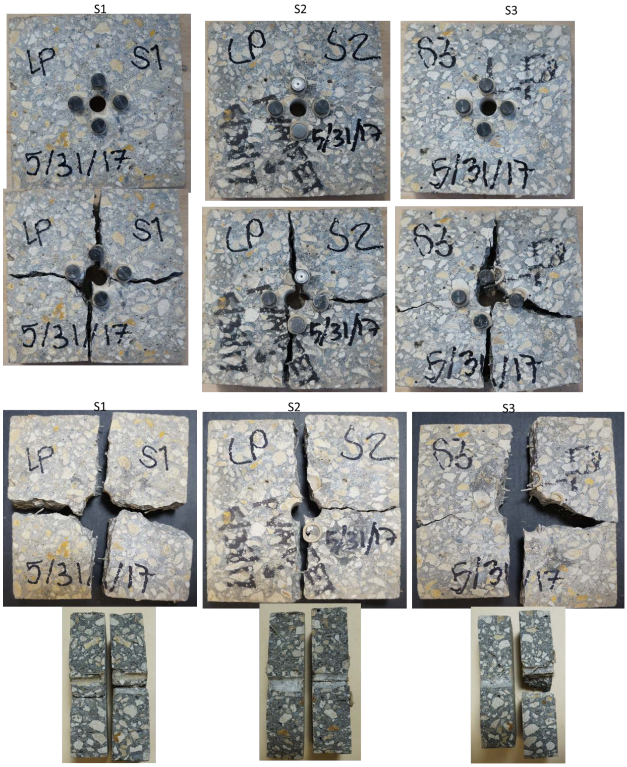
Figure 197. Visual inspection after modified IDT on mix 6 samples (SW_LpH)
