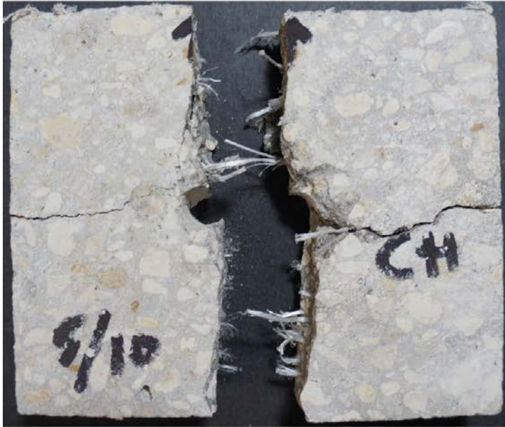
Figure 182. Visual inspection after modified IDT on mix 3 sample (CH)
