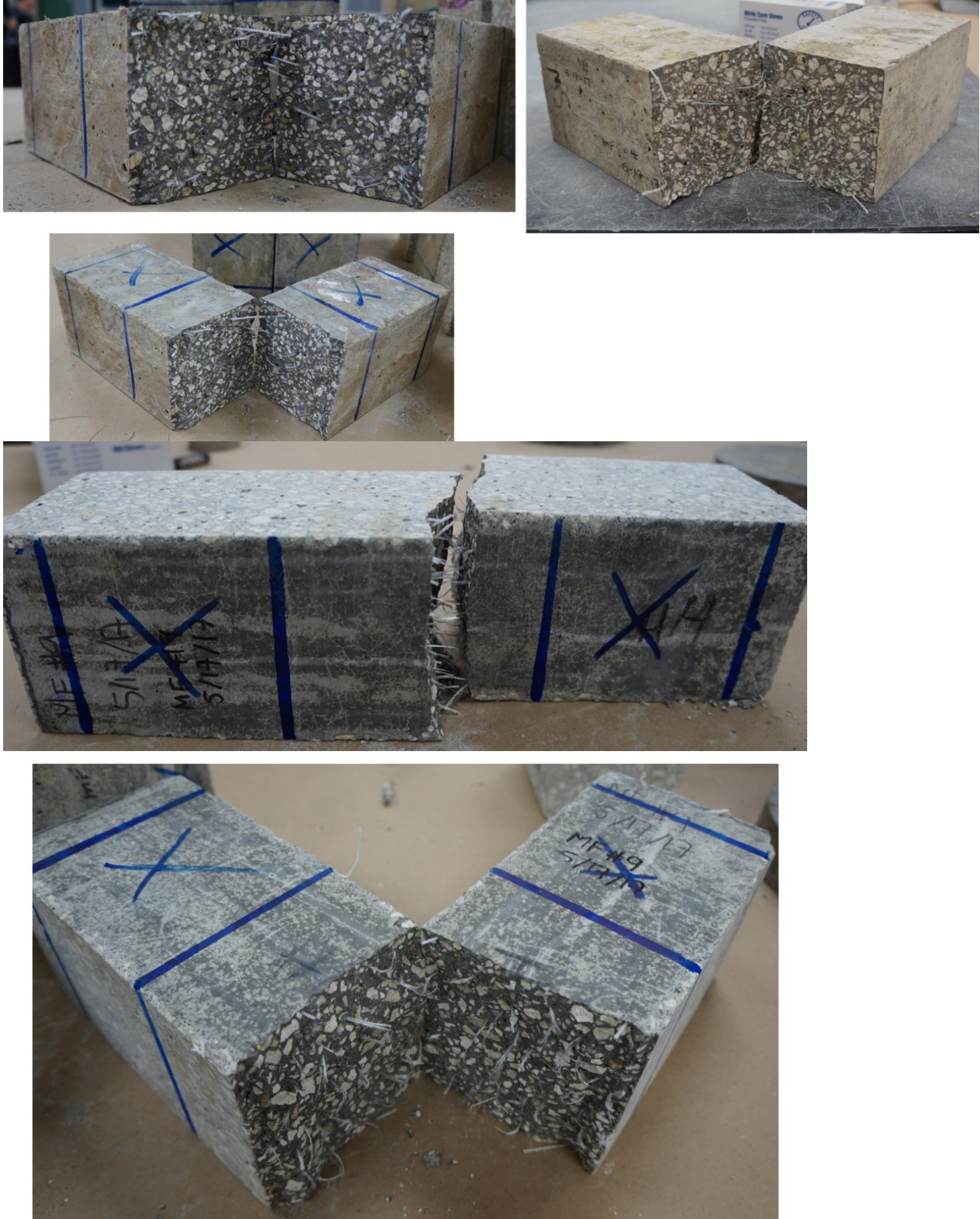
Figure 161. Fiber distribution after residual strength tests on beams of mix 4
