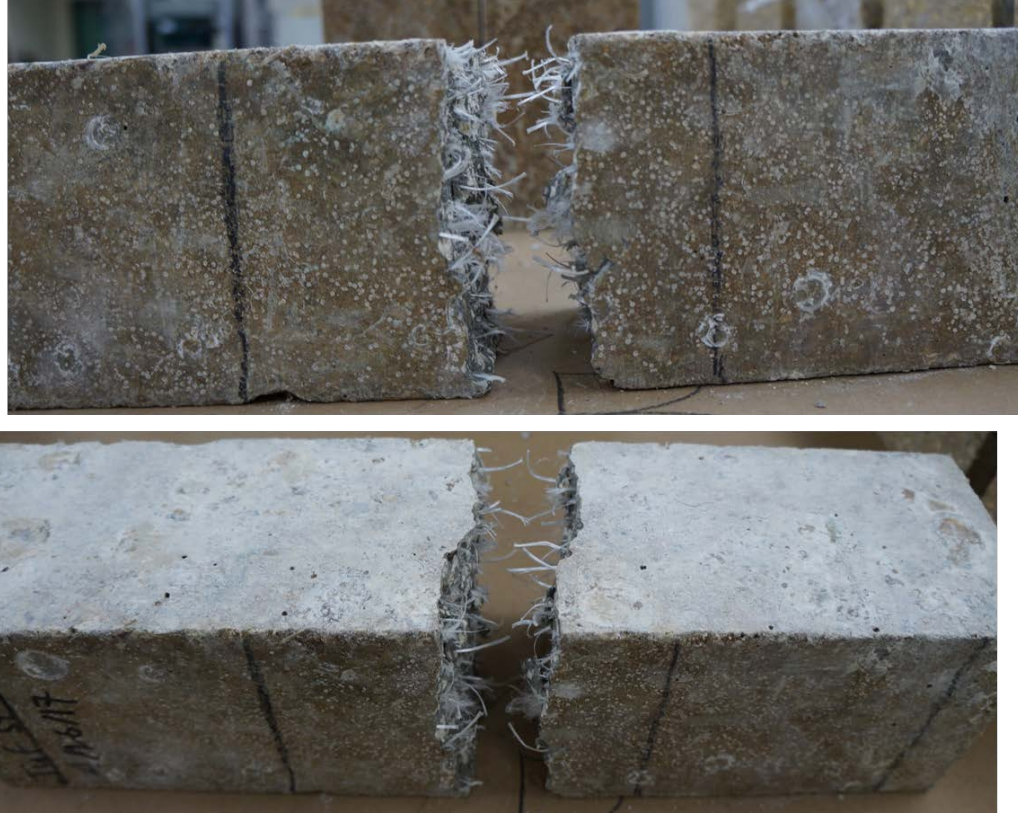
Figure 69. Mix 2 beams after residual strength testing (exposed at the barge). Longitudinal direction.
