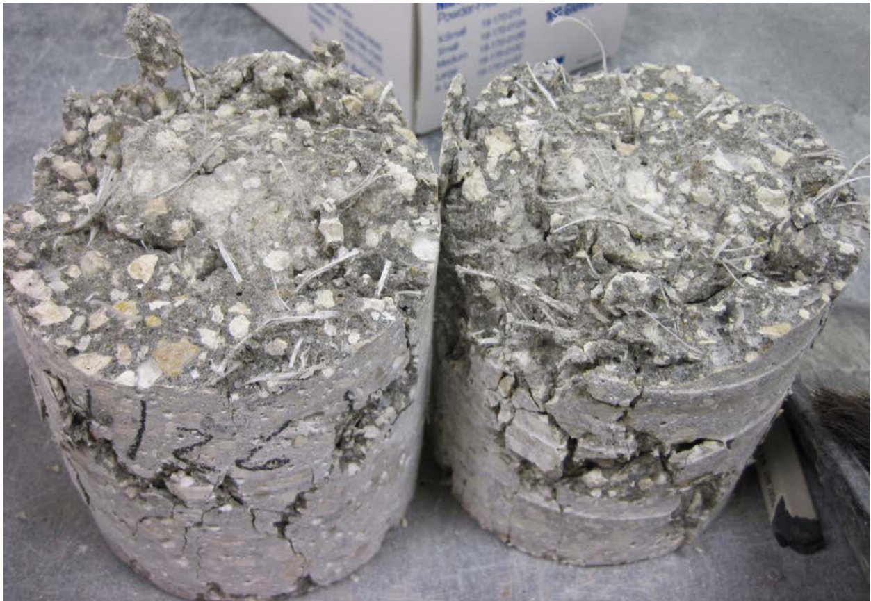
Figure 127. Visual inspection of fiber distribution after compression test on cores of mix 2
