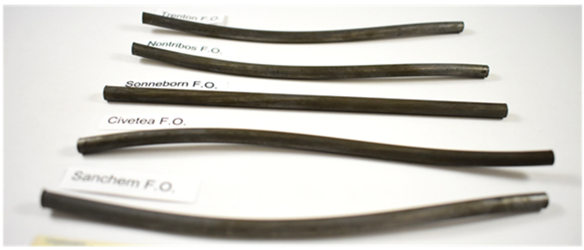
Figure 269. Coated with filler and sprayed with 0.6 milliliter of solution containing fungus FO
