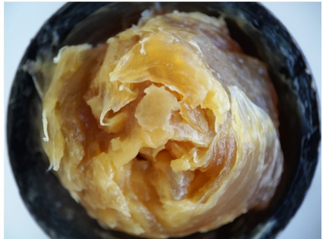
Figure 93. Sonneborn NC sample sprayed with fungi mix (one side) (June 2018).
