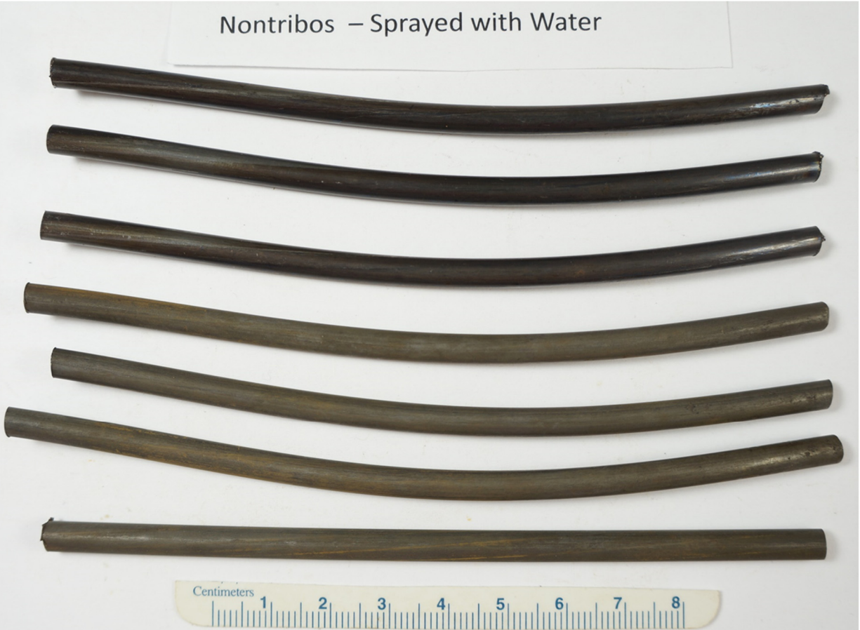
Figure 133. . Section of Nontribos coated strand, after cleaning – (water)
