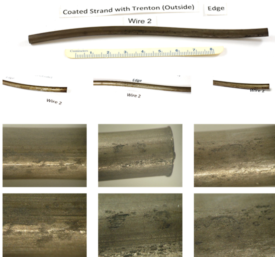
Figure 196. View of coated strand with Trenton (outside) edge, wire 2 after removing filler and cleaning (close-up 2)
