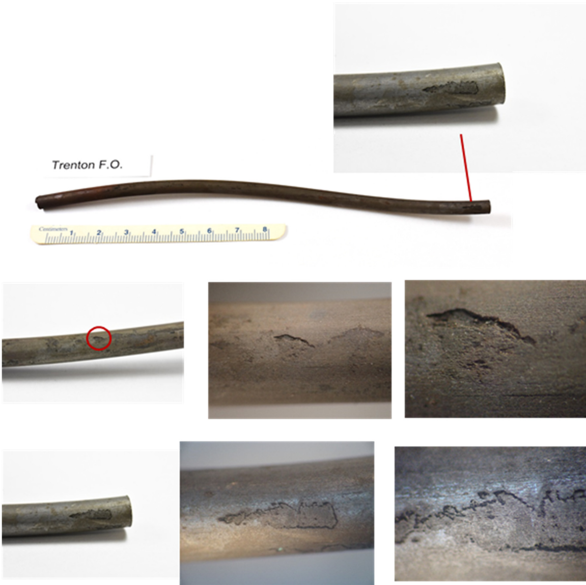
Figure 240. Coated with filler Trenton and sprayed with 1.5 milliliter of solution containing fungus FO (close-up 2)
