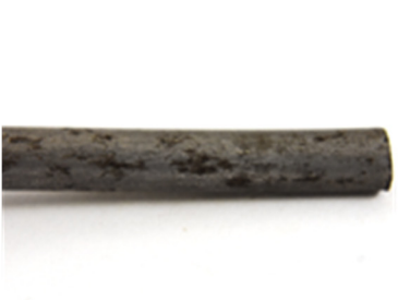
Figure 221. Single wire coated with Nontribos at 20°C at high humidity
