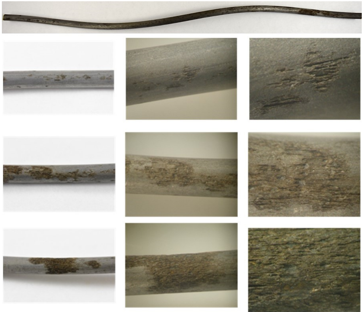
Figure 225. Single wire blank at 20°C at high humidity
