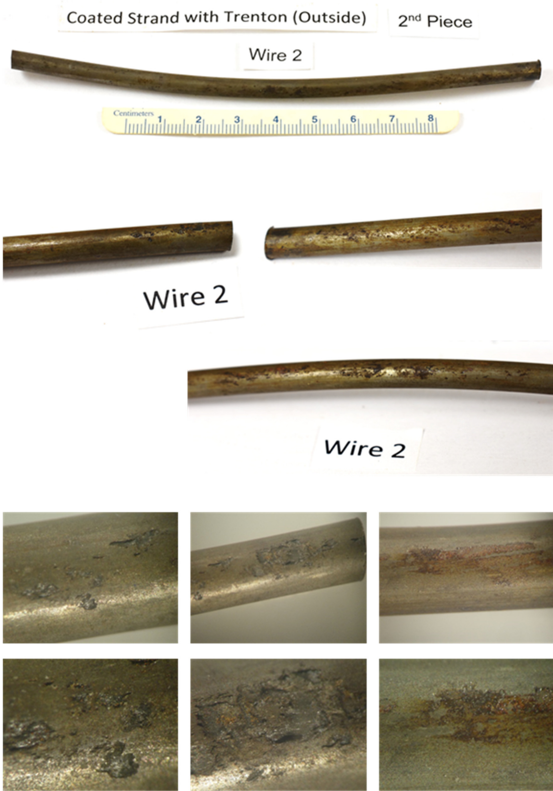
Figure 204. View of coated strand with Trenton (outside) 2 nd piece, wire 2 after cleaning
