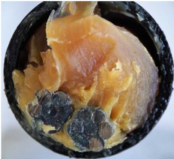
Figure 94. Sanchem NC sample sprayed with fungi mix (one side) (December 2017).
