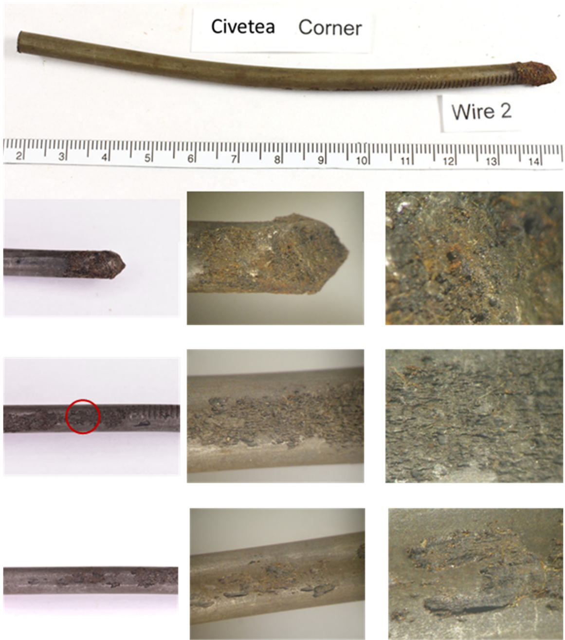
Figure 162. View of wire 2 after removing filler and cleaning (full view).
