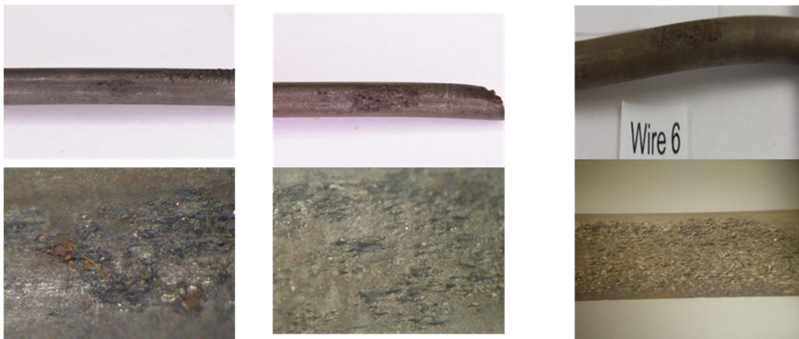
Figure 48. Wires from the strand coated with Civetea (edge): (a) Wire 3; (b) Central wire; (c) Wire 6.
