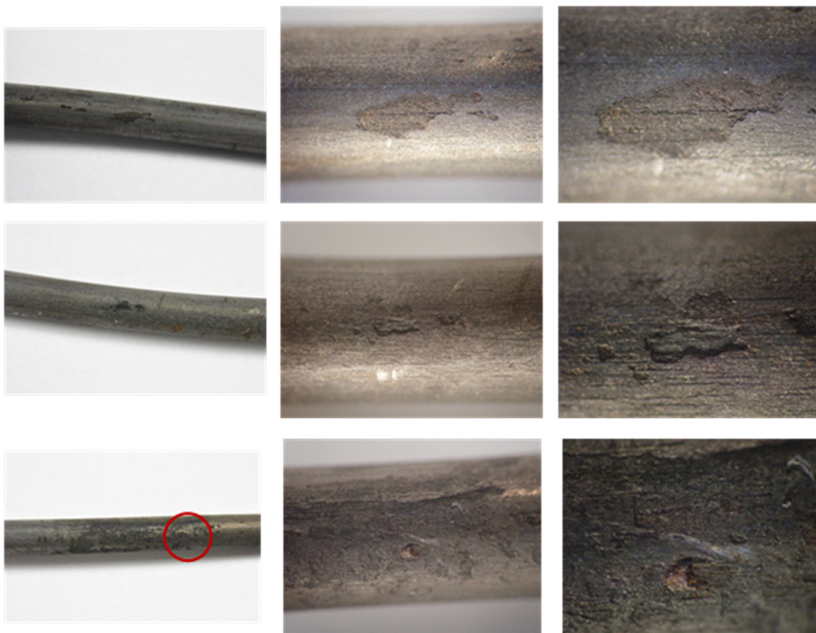
Figure 241. Coated with filler Nontribos and sprayed with 1.5 milliliter of solution containing fungus FO (close-up 3)
