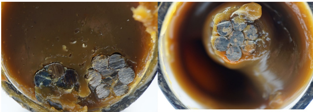
Figure 92. Sonneborn NC sample sprayed with fungi mix (one side) (December 2017).
