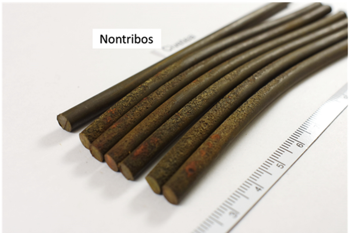
Figure 186. View of strand wires after removing Nontribos filler and cleaning
