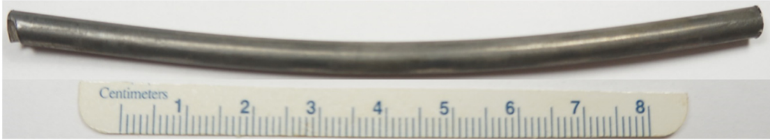
Figure 154. Wire after cleaning removed from samples injected with Sanchem – sprayed with fungi mix
