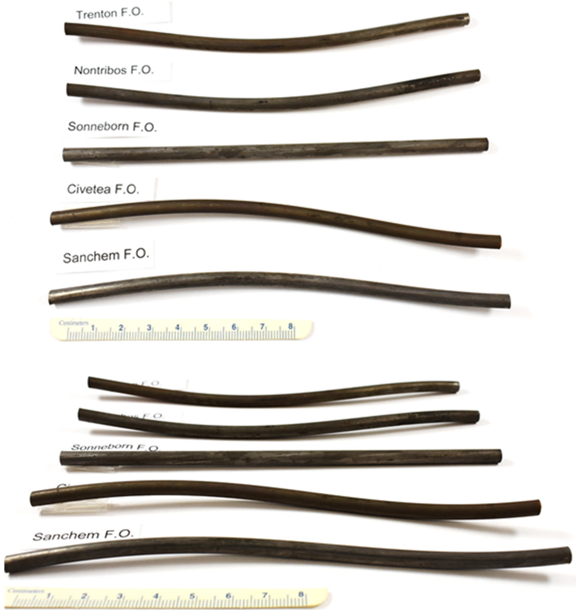
Figure 238. Coated with filler and sprayed with 1.5 milliliter of solution containing fungus FO
