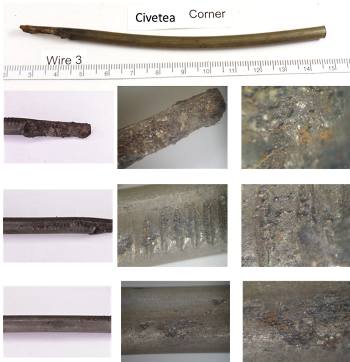
Figure 163. View of wire 3 after removing filler and cleaning (full view).
