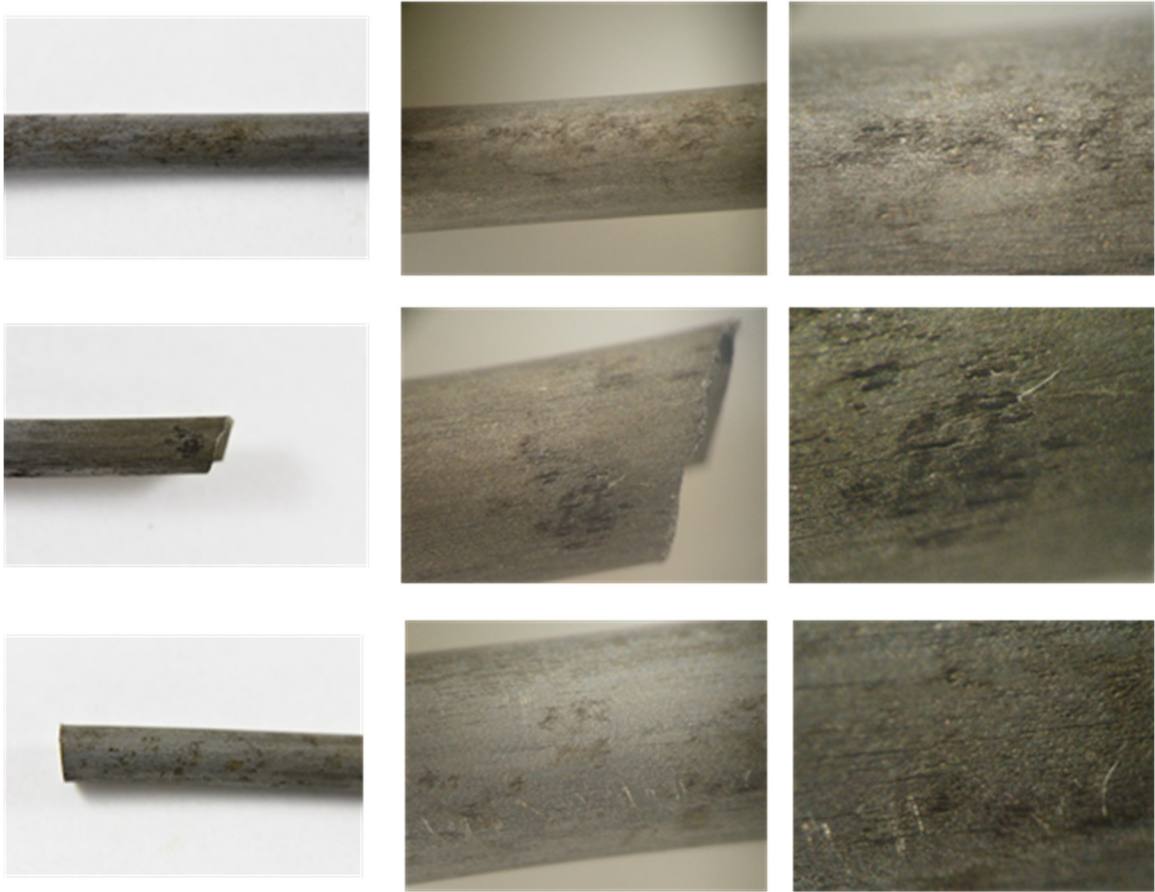
Figure 223. Single wire coated with Civetia at 20°C at high humidity
