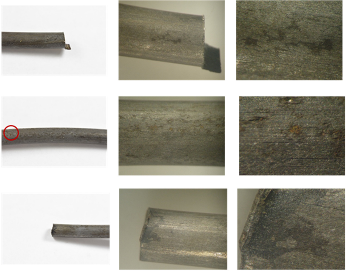
Figure 227. Single wire coated with Nontribos at 32°C at high humidity
