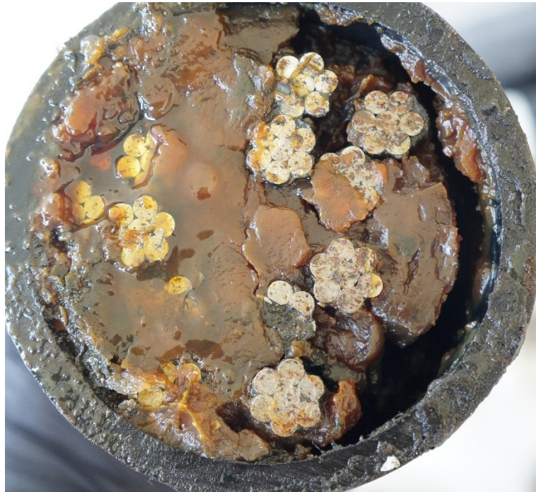
Figure 79. Four-inch diameter sample, side sprayed with Water (June 2018).
