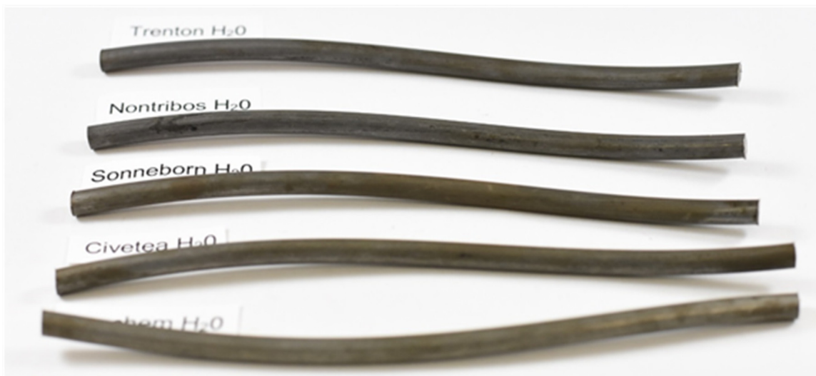
Figure 280. Coated with filler and sprayed with 0.6 milliliter of water.
