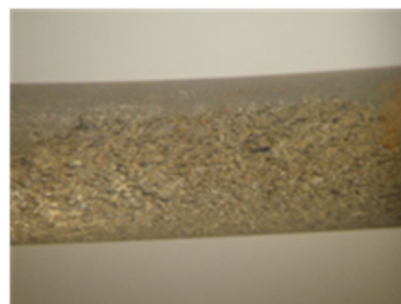
Figure 190. View of 2nd strand segment, wire 4 after removing filler and cleaning (close-up)
