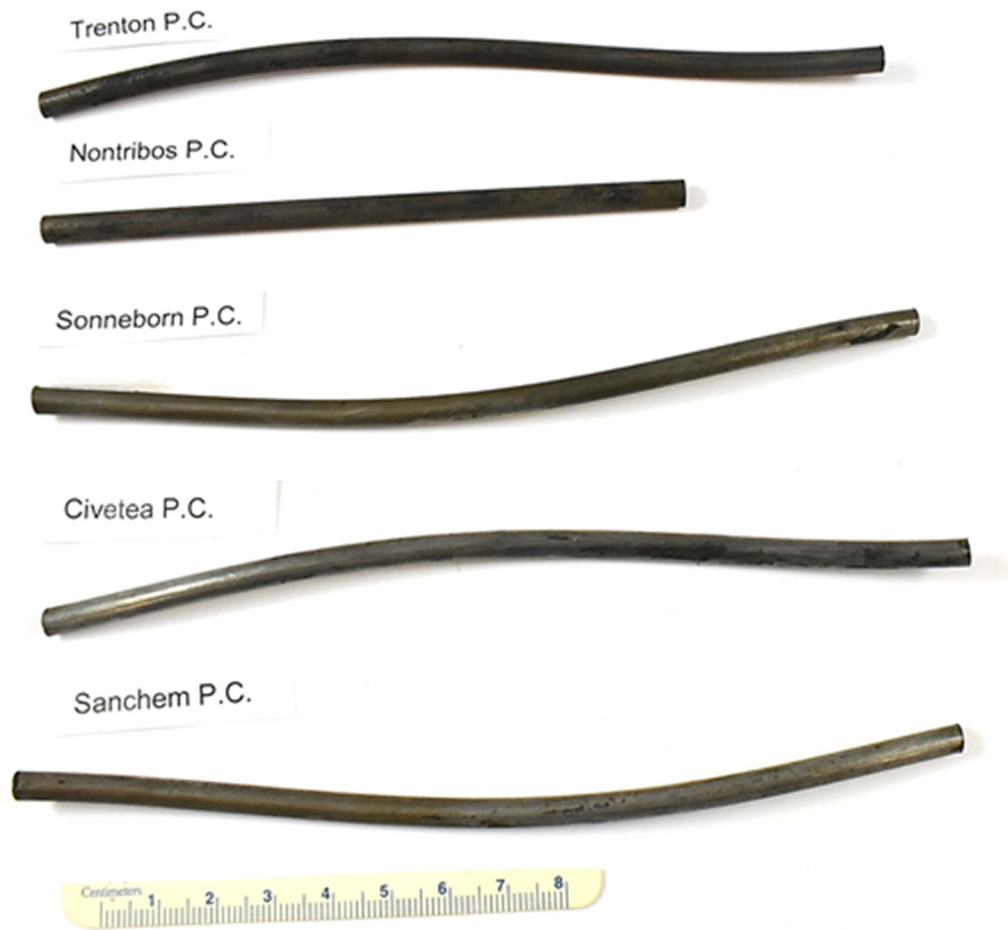
Figure 253. Coated with filler and sprayed with 1.5 milliliter of solution containing fungus PC
