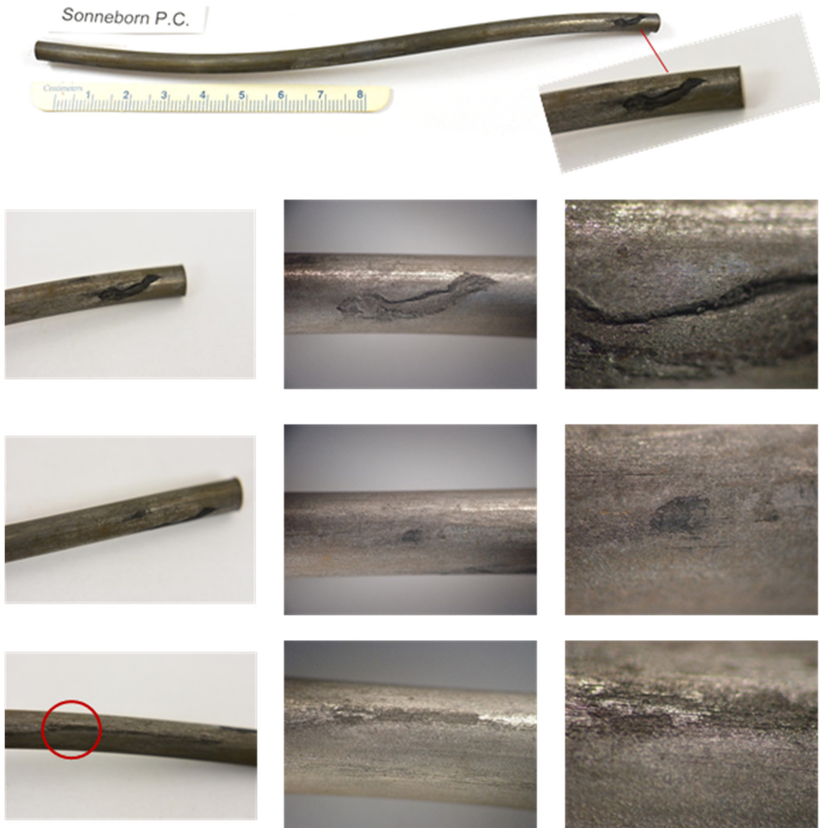
Figure 256. Coated with filler Sonneborn and sprayed with 1.5 milliliter of solution containing fungus PC (close-up).
