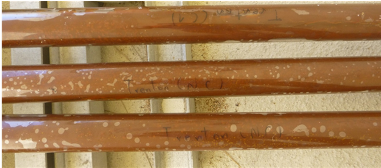
Figure 15. Two-inch diameter 4-foot long samples injected with Trenton (two NC and one C1 conditions)
