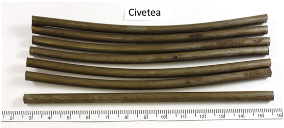
Figure 168. View of second strand segment: wires after removing filler and cleaning
