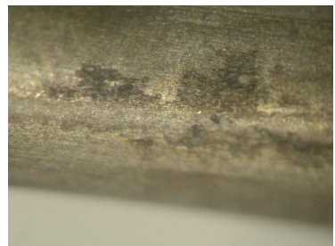
Figure 195. View of coated strand with Trenton (outside) edge, wire 1 after removing filler and cleaning (close-up)
