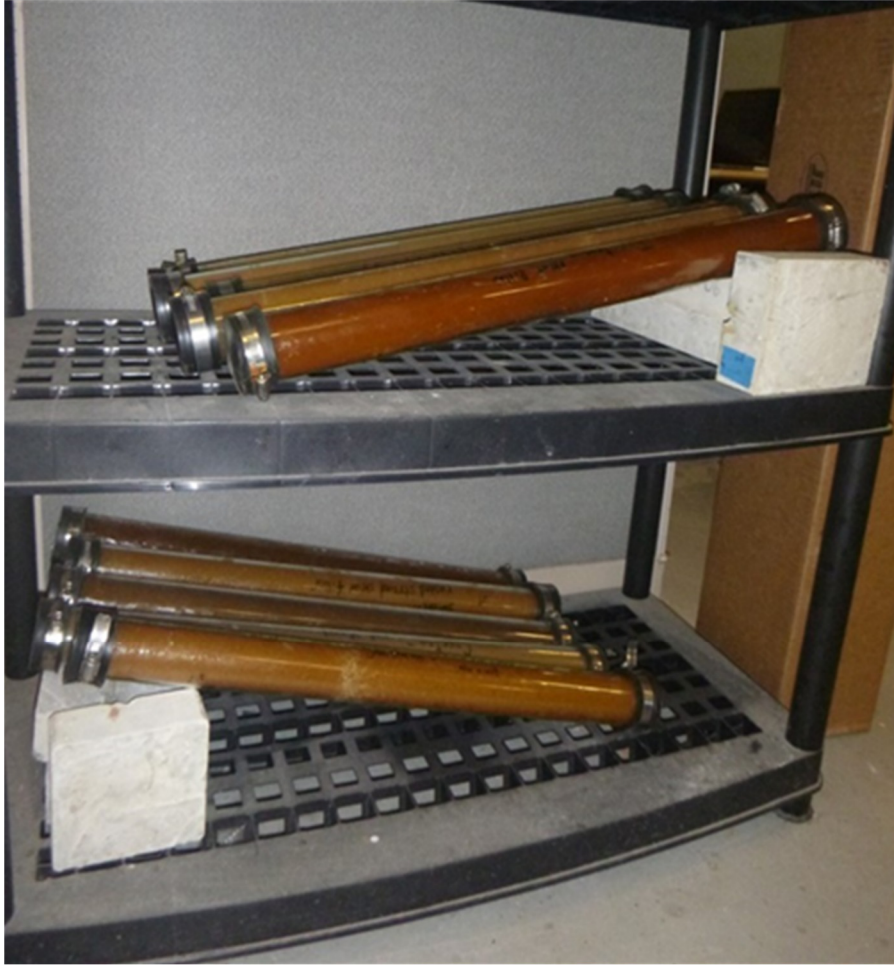
Figure 17. Two-inch diameter, 2 foot long samples stored in the laboratory at a shelf
