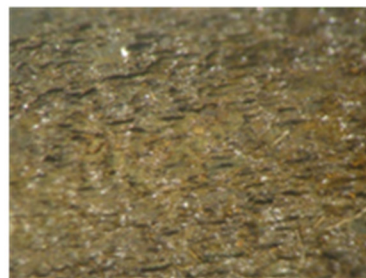
Figure 193. View of 2nd strand segment, wire 7 after removing filler and cleaning (close-up 1)
