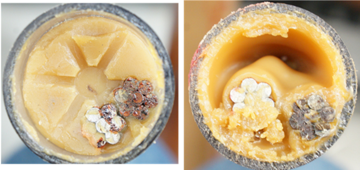
Figure 111. Two-foot long samples injected with Civetea filler (polycarbonate tubing) sprayed with fungi mix (June 2018).
