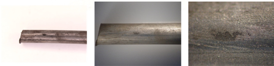
Figure 289. Coated with filler Sanchem and sprayed with 0.6 milliliter of water (close-up 2).
