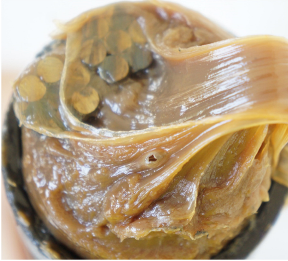
Figure 93. Sonneborn NC sample sprayed with fungi mix (one side) (June 2018).
