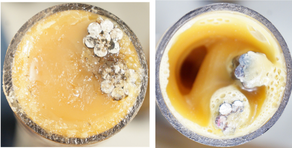
Figure 117. Two-foot long samples injected with Sanchem filler (polycarbonate tubing) sprayed with fungi mix (June 2018).
