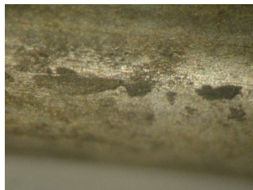
Figure 195. View of coated strand with Trenton (outside) edge, wire 1 after removing filler and cleaning (close-up)
