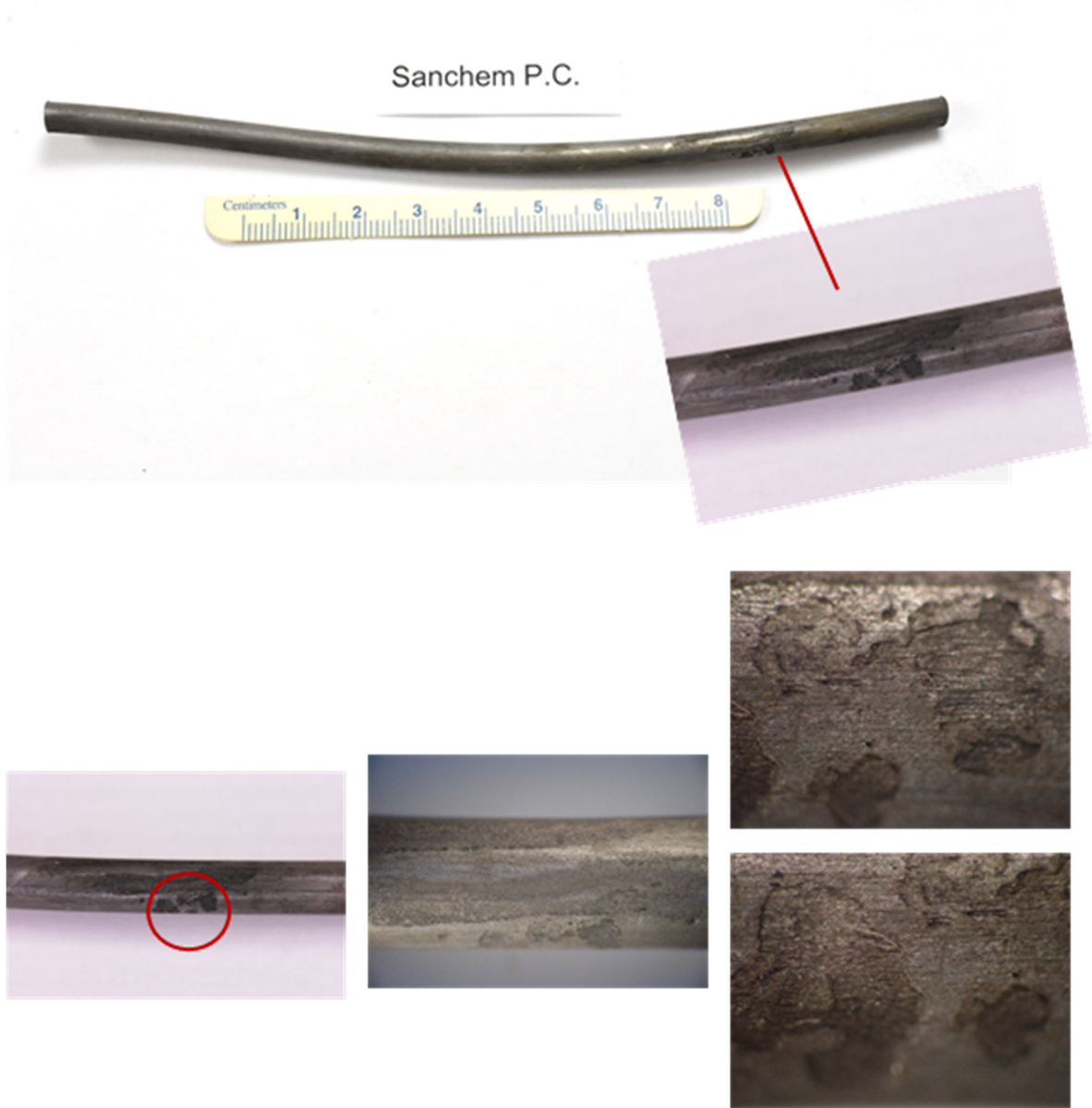
Figure 308. Coated with filler Sanchem and sprayed with 0.6 milliliter of solution containing fungus PC (close-up 1).
