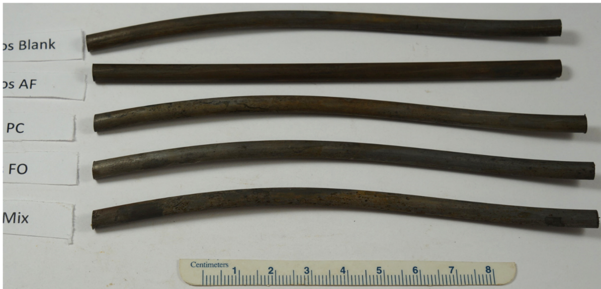
Figure 149. Wires after cleaning removed from samples injected with Nontribos.
