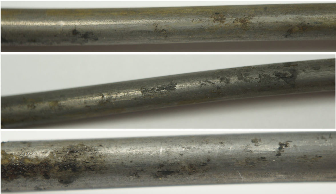
Figure 127. Close-up selected wires, after cleaning (Nontribos fungi mix)
