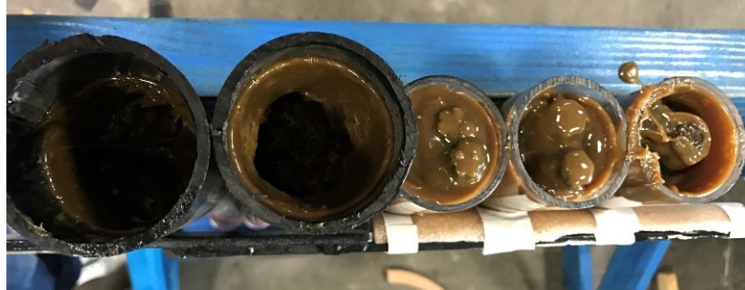
Figure 10. Top view of flexible filler cooling down prior to capping.
