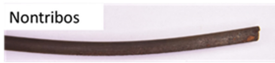
Figure 182. View of 1st strand segment, wire 5 after removing filler and cleaning
