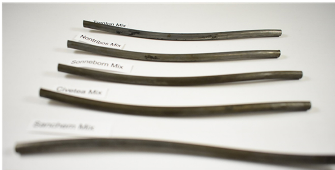
Figure 290. Coated wires sprayed with 0.6 milliliter of solution containing fungi mix
