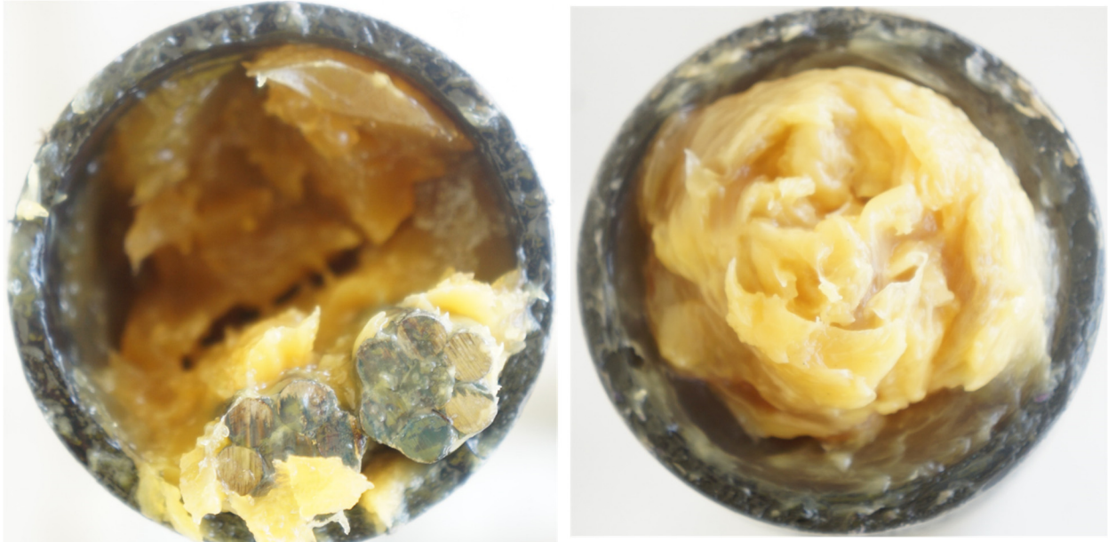
Figure 95. Sanchem NC sample sprayed with fungi mix (one side) (June 2018).
