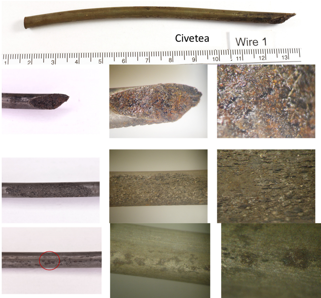
Figure 161. View of wire 1 after removing filler and cleaning
