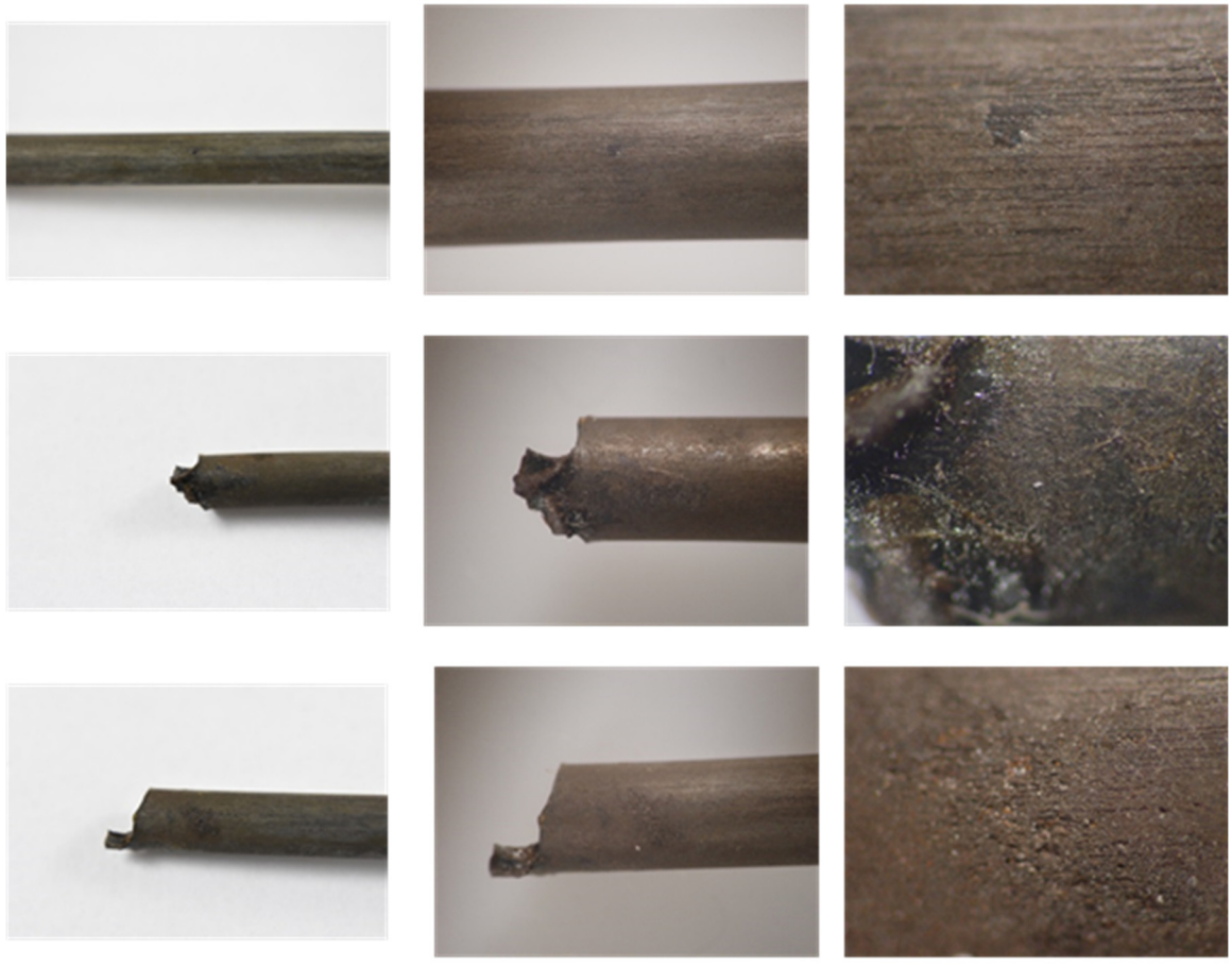
Figure 216. Single wire coated with Nontribos exposed outdoors inside partially closed container
