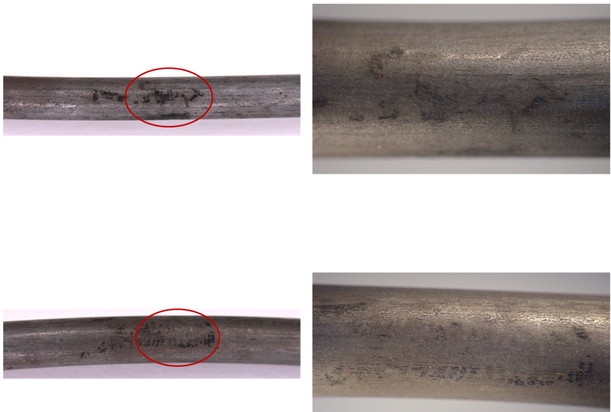
Figure 69. Close-ups – wire coated with Trenton and sprayed with Penicillium chrysogenum .
