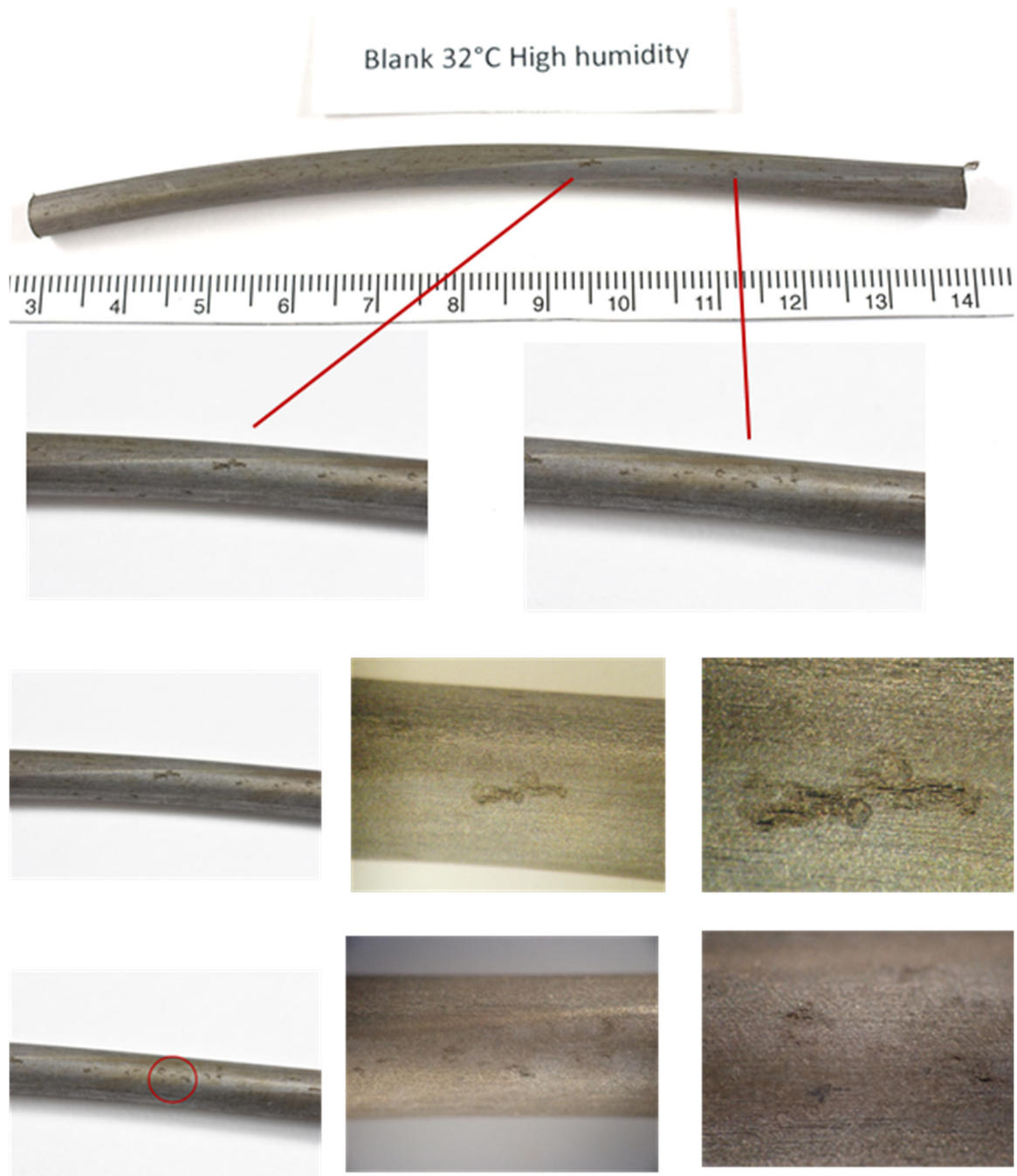
Figure 231. Single wire blank at 32°C at high humidity
