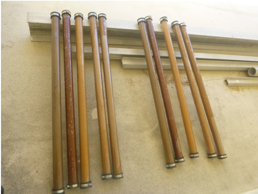
Figure 14. Two-inch diameter samples injected with various flexible fillers.
