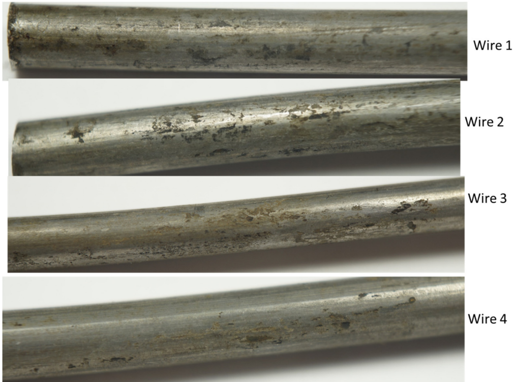
Figure 121. Close-up selected wires, after cleaning. (Trenton – fungi mix)
