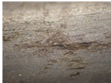
Figure 221. Single wire coated with Nontribos at 20°C at high humidity
