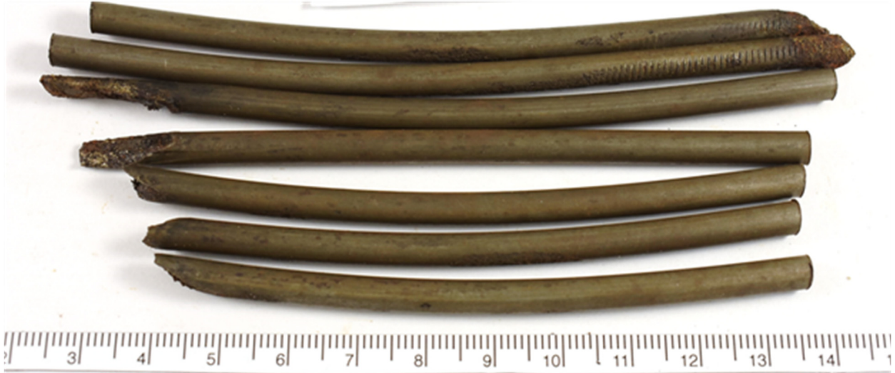
Figure 160. View of strand wires coated with Civetea after removing filler and cleaning
