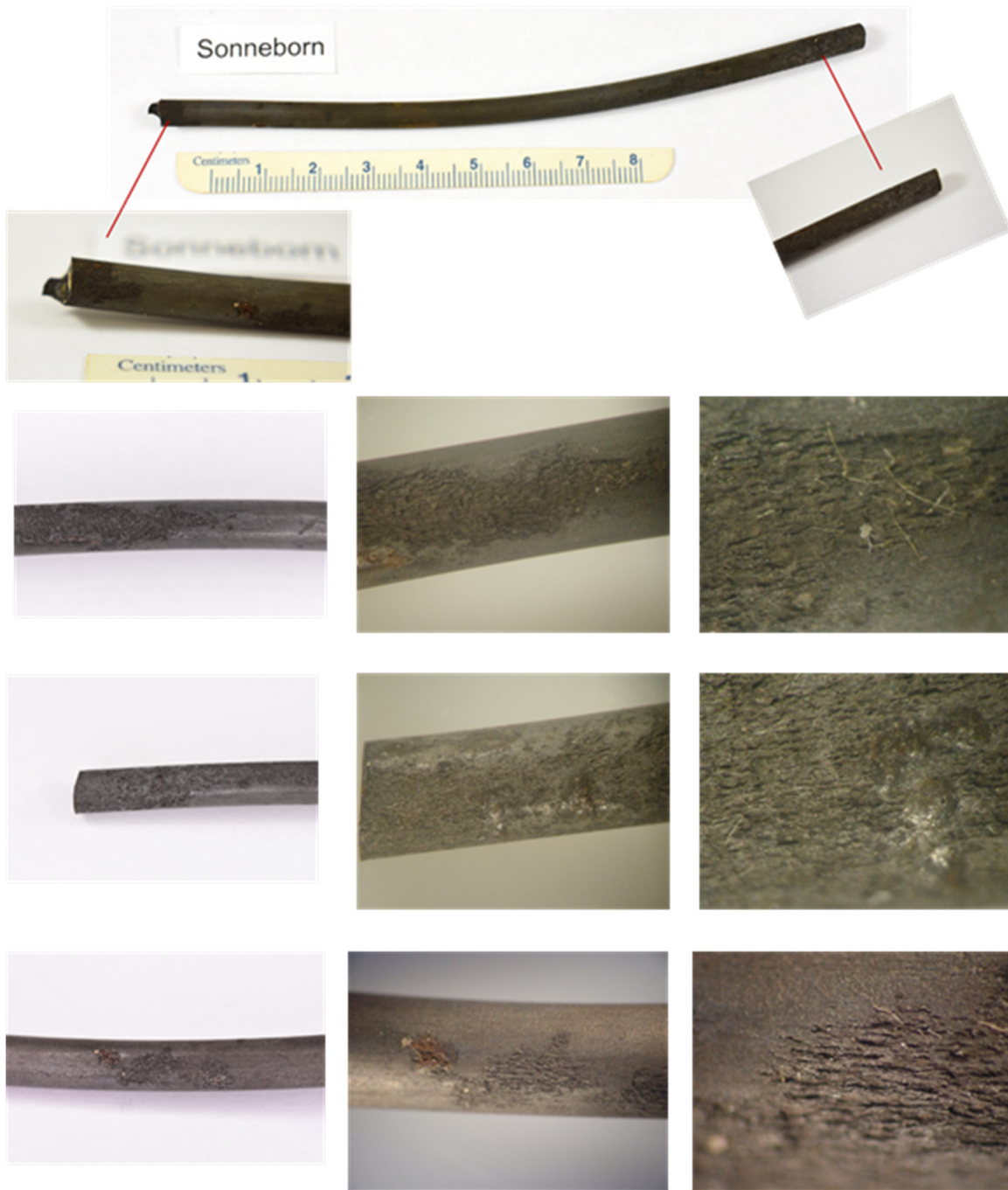
Figure 213. Single wire coated with Sonneborn exposed outside semi-sheltered area
