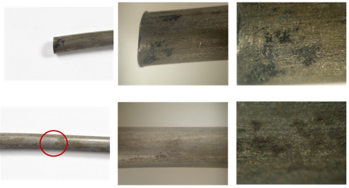
Figure 229. Single wire coated with Civetea at 32°C at high humidity.
