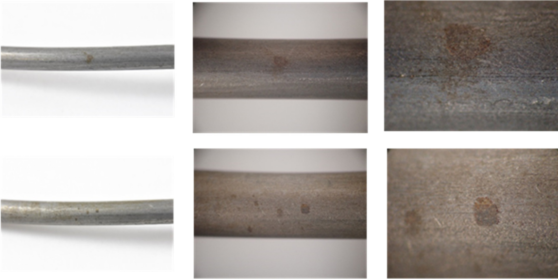
Figure 220. Single wire coated with Trenton at 20°C at high humidity.
