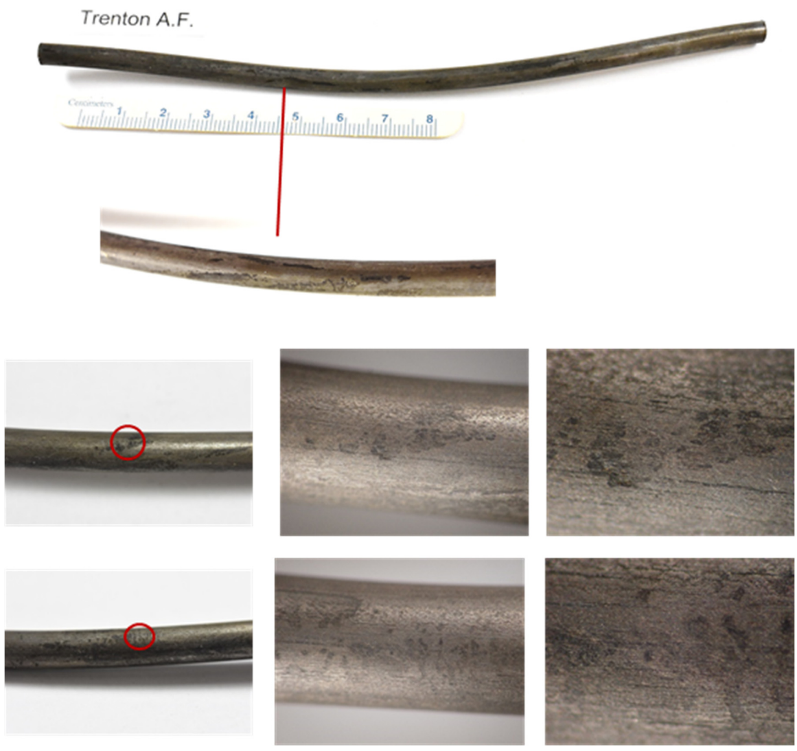
Figure 234. Coated with filler Trenton and sprayed with 1.5 milliliter of solution containing fungus AF
