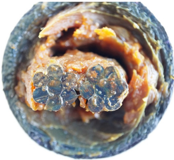
Figure 90. Trenton NC sample sprayed with fungi mix (one side) (December 2017).
