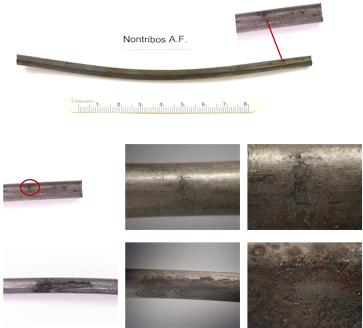
Figure 262. Coated with filler Nontribos and sprayed with 0.6 milliliter of solution containing fungus AF (close-up 1).
