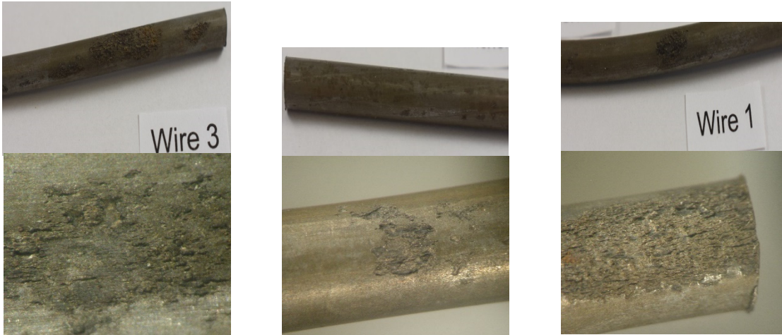
Figure 49. Wires from the strand coated with Civetea: (a) Wire 3; (b) Central wire; (c) Wire 1.
