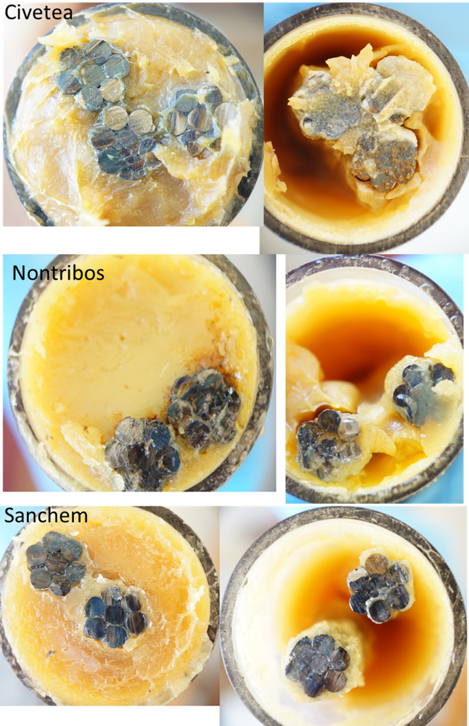
Figure 106. Samples injected with flexible fillers (polycarbonate tubing) and sprayed with water. (December 2017)
