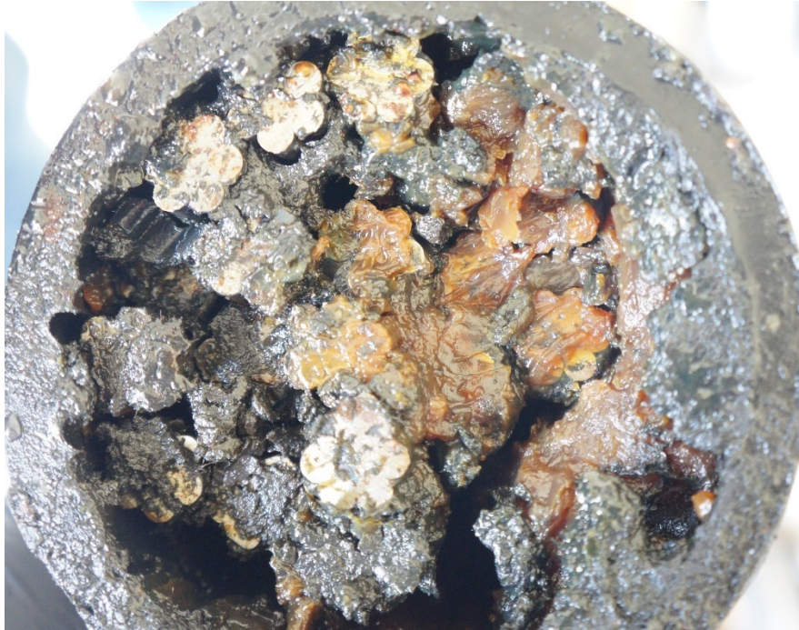
Figure 81. Four-inch diameter sample, side sprayed with fungi mix. June 2018.
