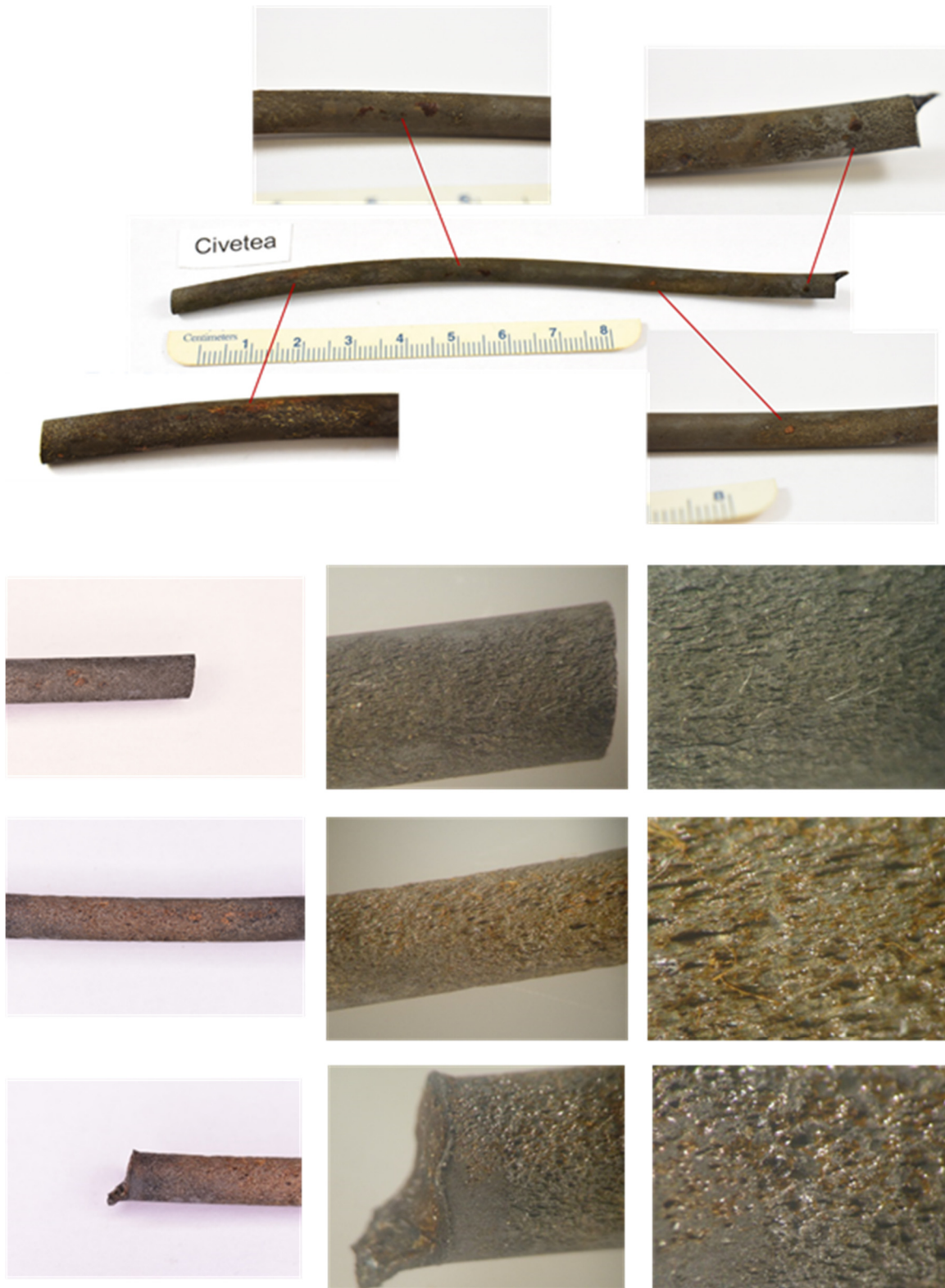
Figure 214. Single wire coated with Civetea exposed outside semi-sheltered area
