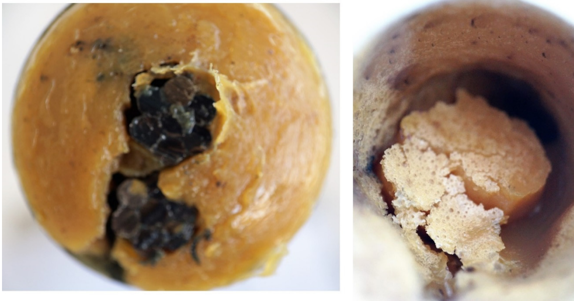
Figure 96. Nontribos NC sample sprayed with fungi mix (December 2017).
