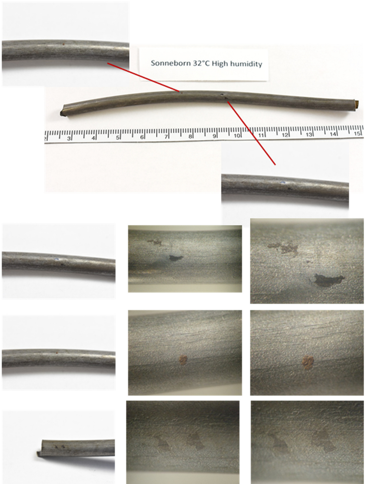
Figure 228. Single wire coated with Sonneborn at 32°C at high humidity
