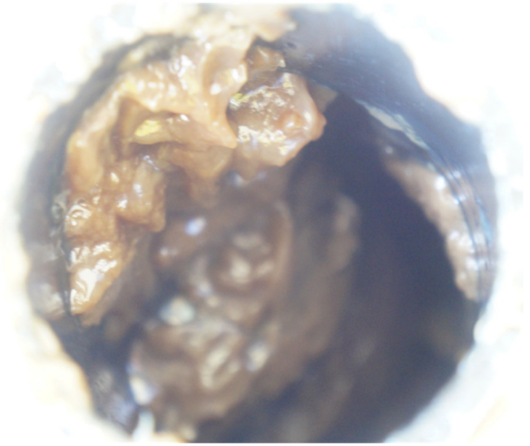
Figure 93. Sonneborn NC sample sprayed with fungi mix (one side) (June 2018).
