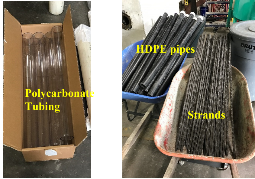
Figure 6. Polycarbonate tubing, HDPE tubing, and steel strands used
