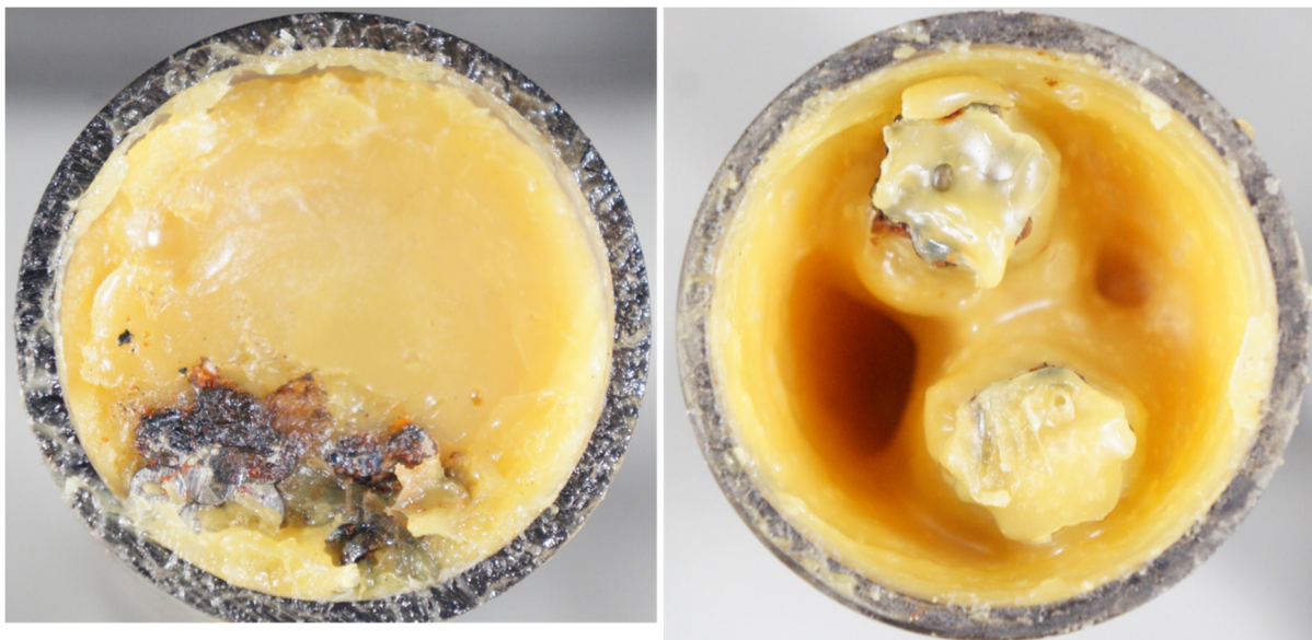
Figure 119. Two-foot long samples injected with Nontribos filler (polycarbonate tubing) sprayed with fungi mix (June 2018)
