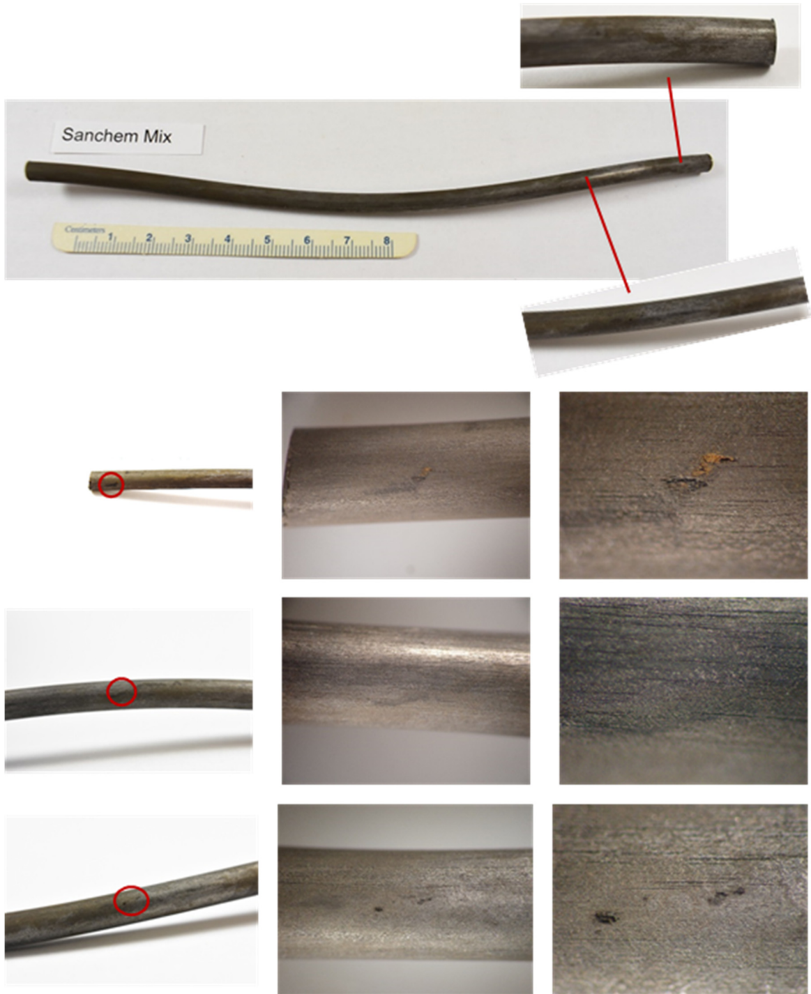
Figure 252. Coated with filler Sanchem and sprayed with 1.5 milliliter of solution containing fungi mix (close-up).
