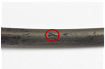
Figure 254. Coated with filler Trenton and sprayed with 1.5 milliliter of solution containing fungus PC (close-up).
