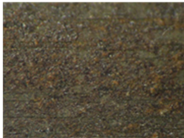
Figure 217. Single wire coated with Sonneborn exposed outdoors inside partially closed container (close-up 2)
