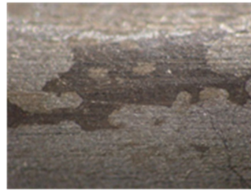
Figure 219. Single wire coated with Sanchem exposed outdoors inside partially closed container.
