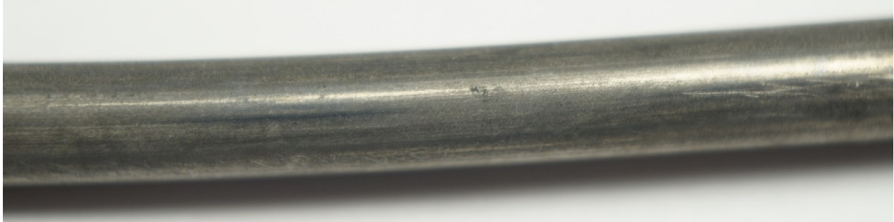
Figure 158. Wire section after cleaning for wire removed from samples injected with Trenton – sprayed with fungi mix.
