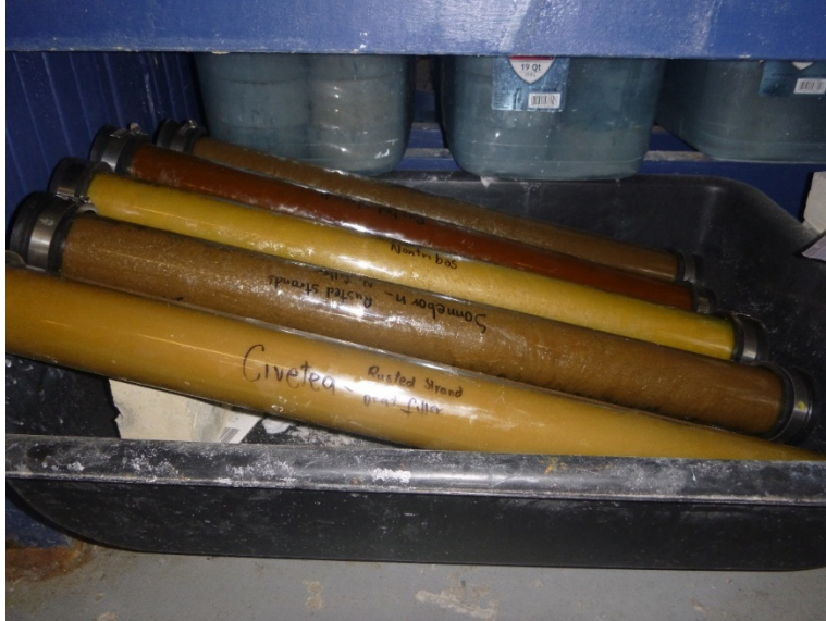
Figure 16. Two-inch diameter, 2-foot long samples stored in the laboratory
