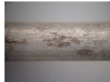
Figure 221. Single wire coated with Nontribos at 20°C at high humidity
