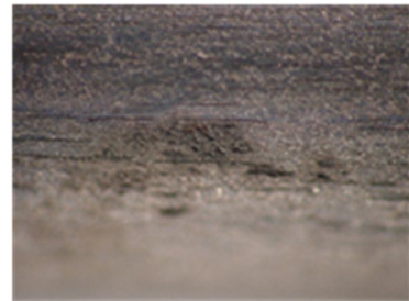
Figure 279. Coated with filler Sanchem and sprayed with 0.6 milliliter of solution containing fungus FO (close-up 2).
