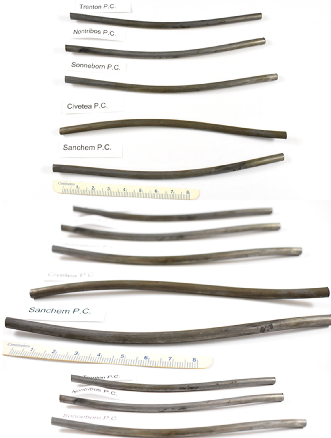
Figure 300. Coated with filler and sprayed with 0.6 milliliter of solution containing fungus PC (full view)
