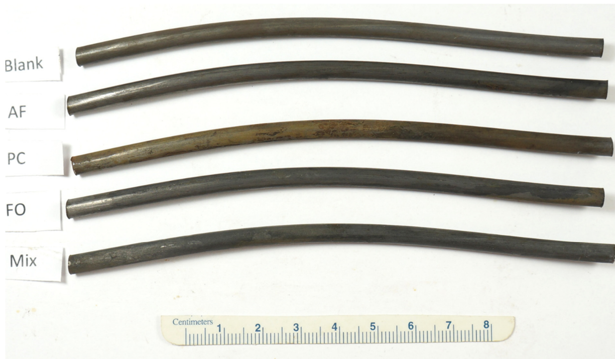
Figure 145. Wires after cleaning removed from samples injected with Civetea.
