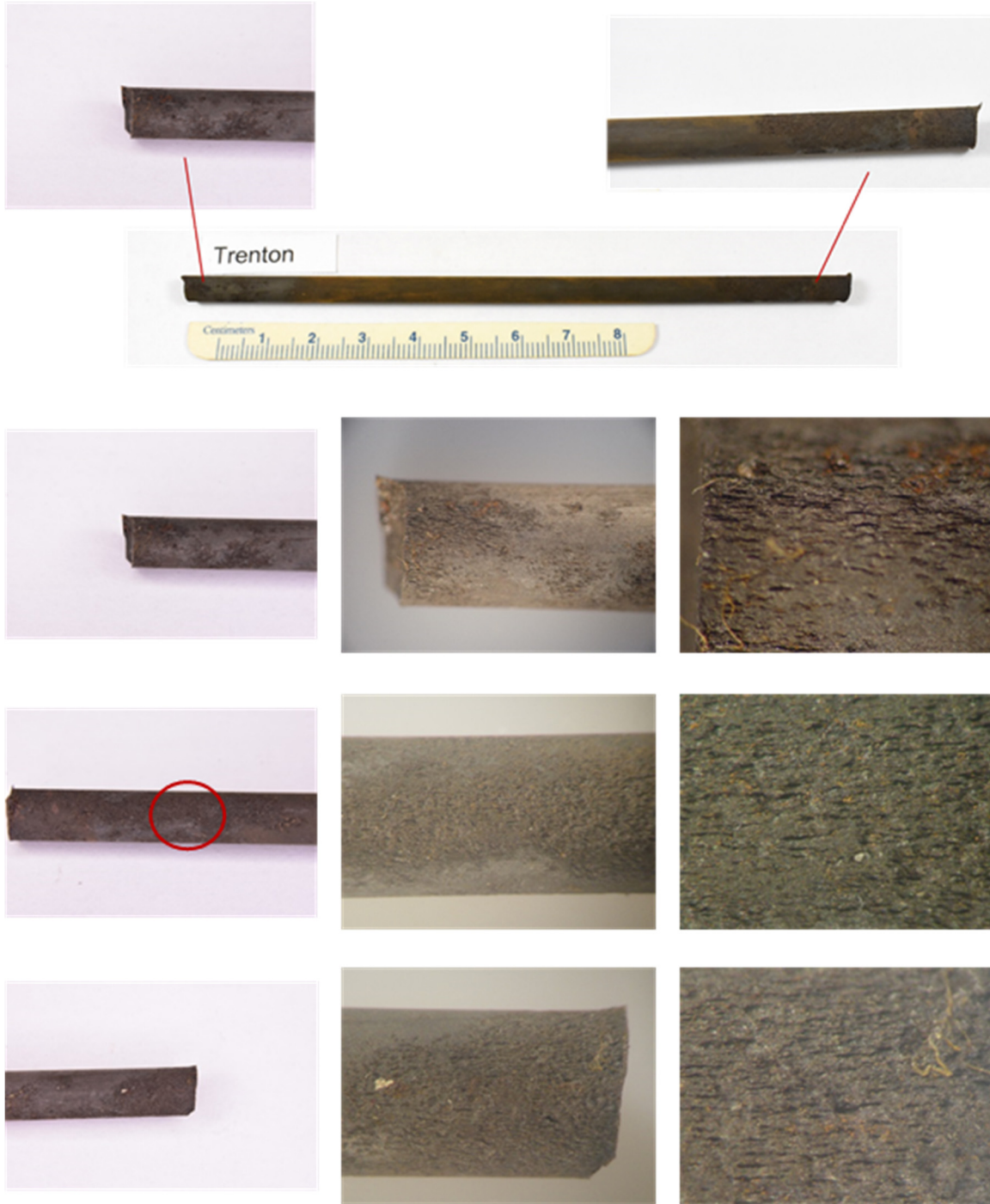
Figure 211. Single wire coated with Trenton exposed outside semi-sheltered area.
