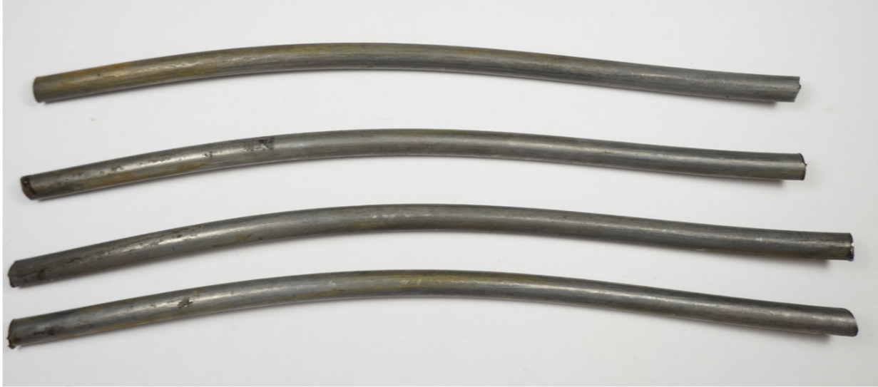
Figure 126. Section of Nontribos coated strand, after cleaning (Nontribos - fungi mix)
