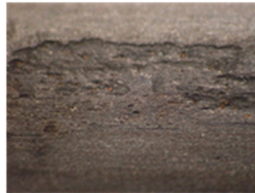
Figure 268. Coated with filler Sanchem and sprayed with 0.6 milliliter of solution containing fungus AF (close-up).
