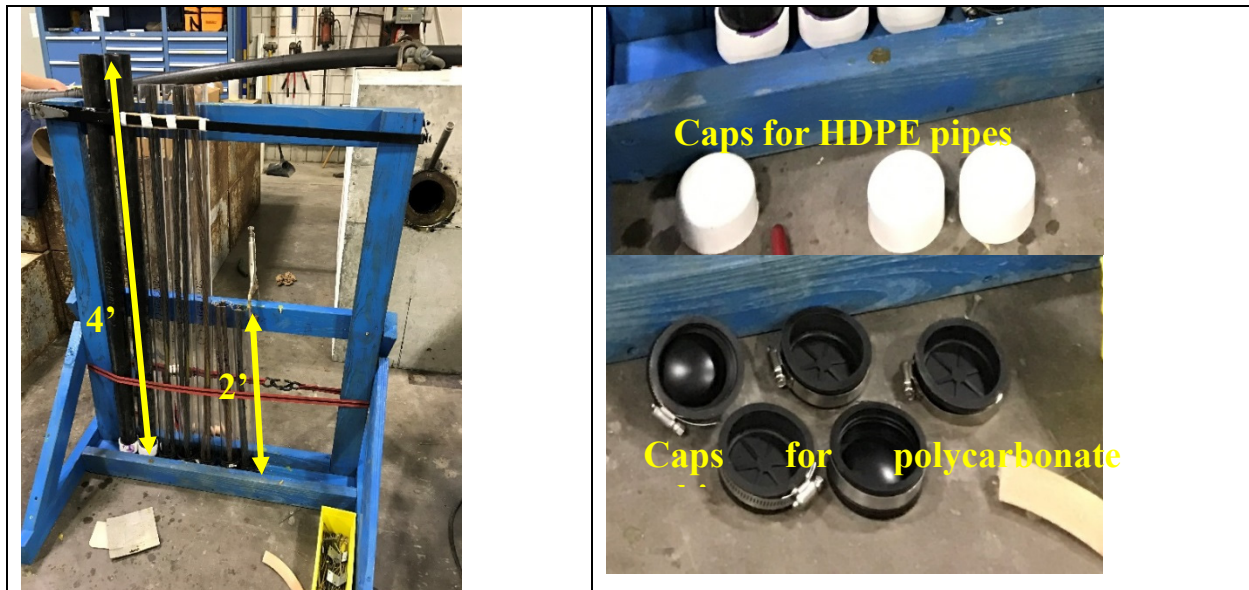
Figure 5. Left: Stand used with tubing ready to be injected; Right: Caps used.
