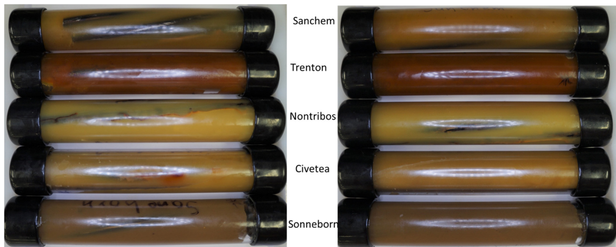
Figure 140. Two views of the five samples sprayed with Aspergillus flavus .
