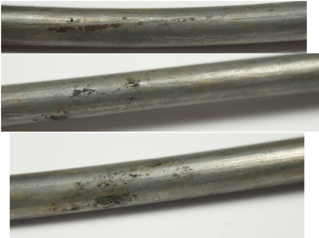
Figure 124. Close-up selected wires, after cleaning (Civetea – fungi mix)
