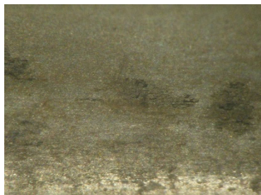
Figure 195. View of coated strand with Trenton (outside) edge, wire 1 after removing filler and cleaning (close-up)
