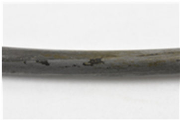
Figure 219. Single wire coated with Sanchem exposed outdoors inside partially closed container.
