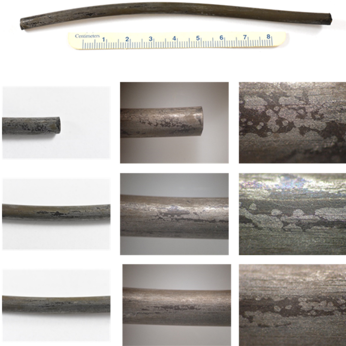
Figure 215. Single wire coated with Trenton exposed outdoors inside partially closed container
