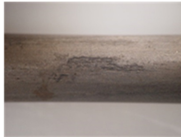
Figure 268. Coated with filler Sanchem and sprayed with 0.6 milliliter of solution containing fungus AF (close-up).
