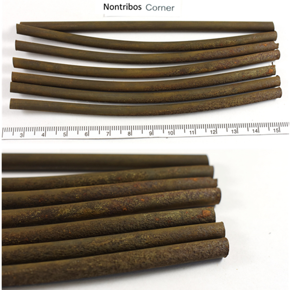
Figure 176. View of strand wires after removing Nontribos filler and cleaning (edge piece)
