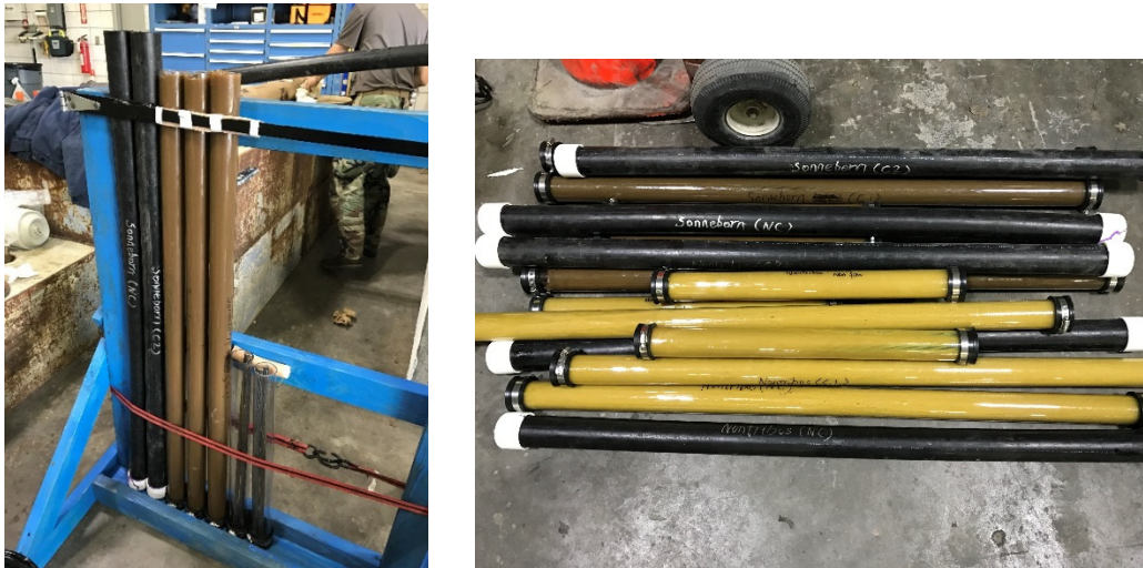
Figure 9. Left: Cooling down of 4-foot samples; Right: After top cap had been placed.
