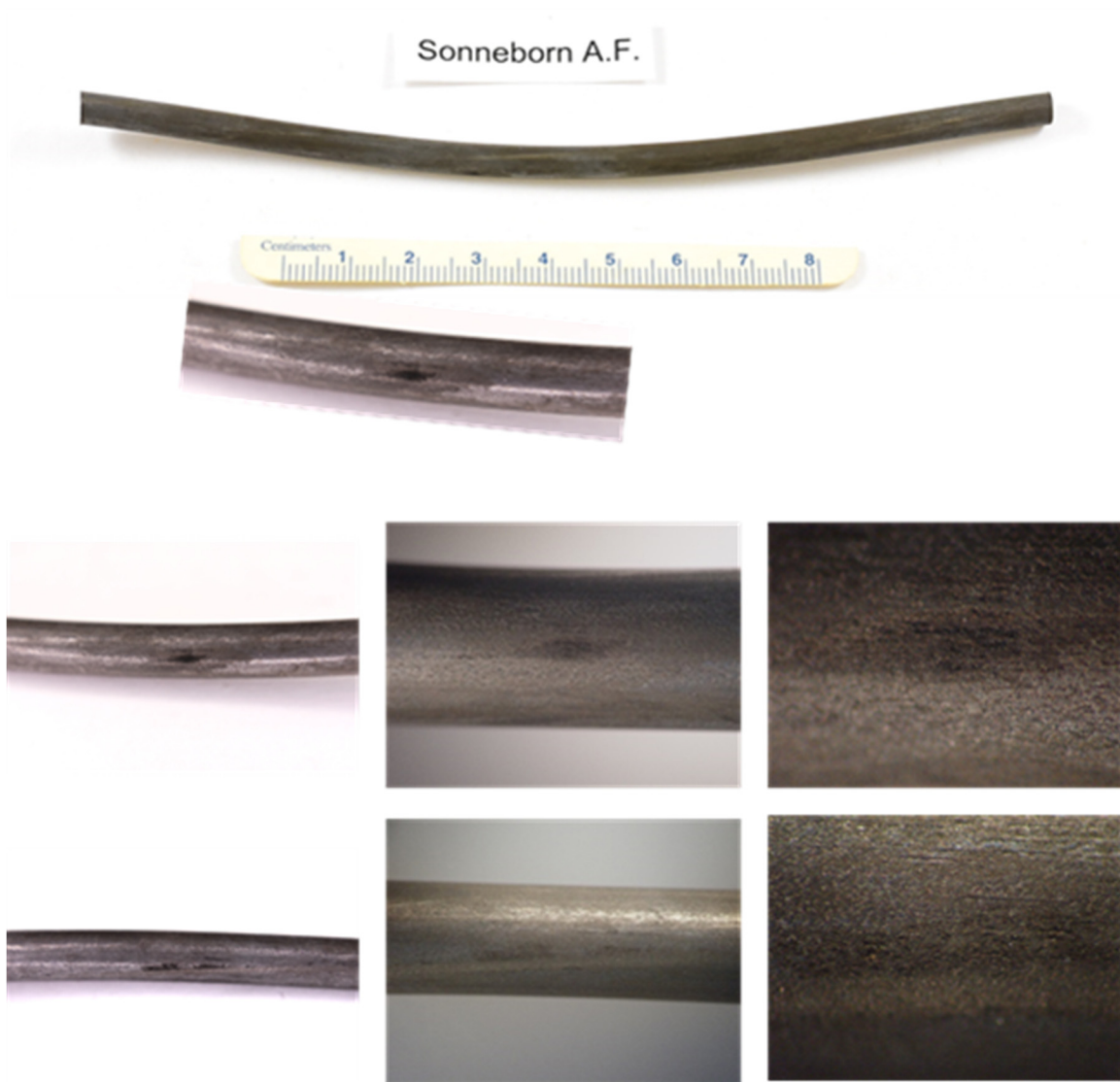
Figure 264. Coated with filler Sonneborn and sprayed with 0.6 milliliter of solution containing fungus AF (close-p view 1).
