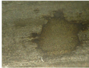
Figure 197. View of coated strand with Trenton (outside) edge, wire 3 after removing filler and cleaning (close-up 2)
