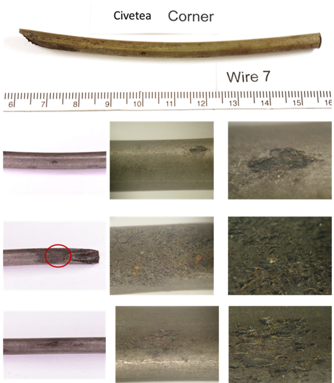
Figure 167. Close-up of wire 7 after removing filler and cleaning
