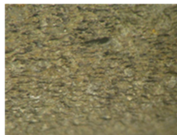
Figure 190. View of 2nd strand segment, wire 4 after removing filler and cleaning (close-up)
