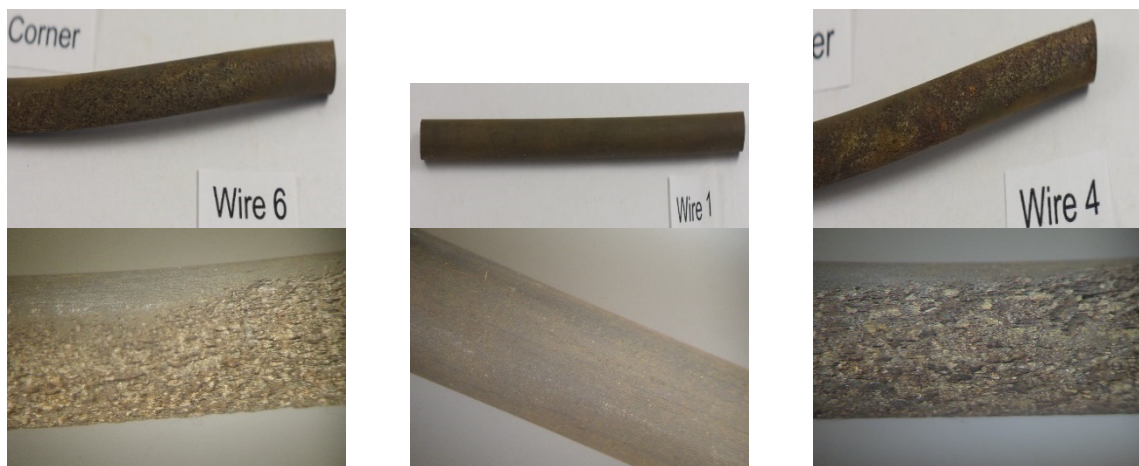
Figure 44. Wires from the strand coated with Nontribos, (a) Wire 6; (b) Central wire; (c) Wire 4.
