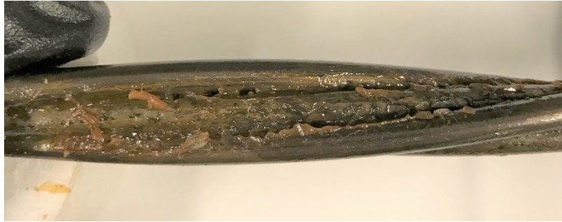
Figure 43. Strand coated with Trenton (182 days after Exposure).
