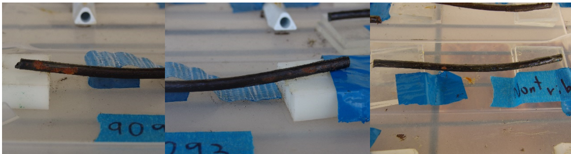
Figure 50. Wires coated and presence of rust. Left and Middle: Sanchem; Right: Nontribos, June 14, 2016.
