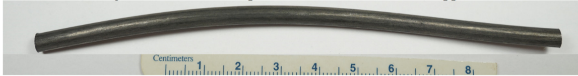
Figure 156. Wire after cleaning removed from samples injected with Sonneborn – sprayed with fungi mix.
