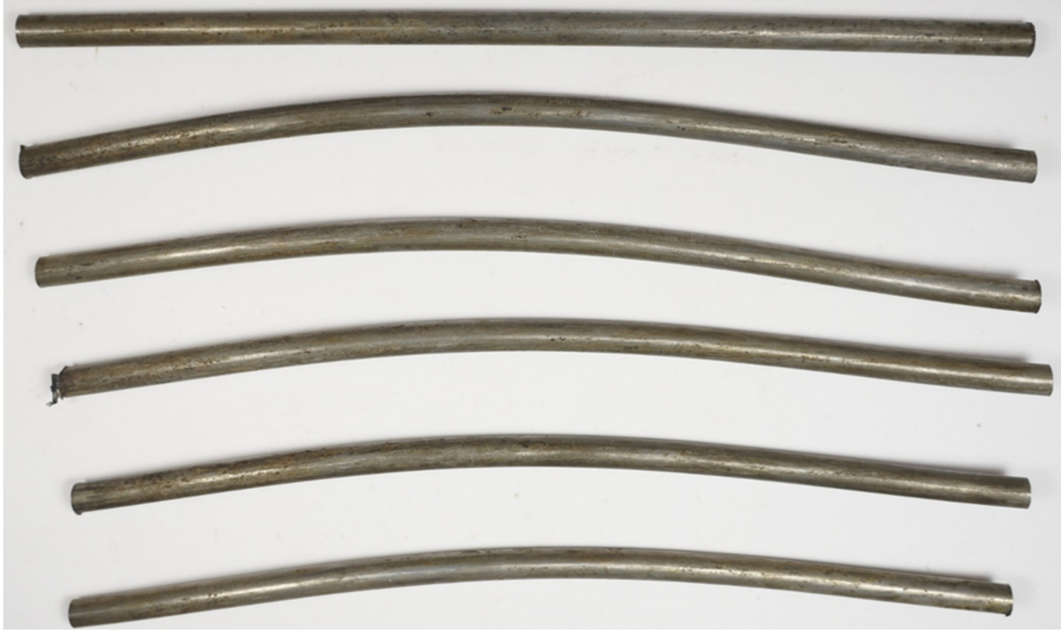
Figure 120. Section of Trenton coated strand (fungi mix), after cleaning
