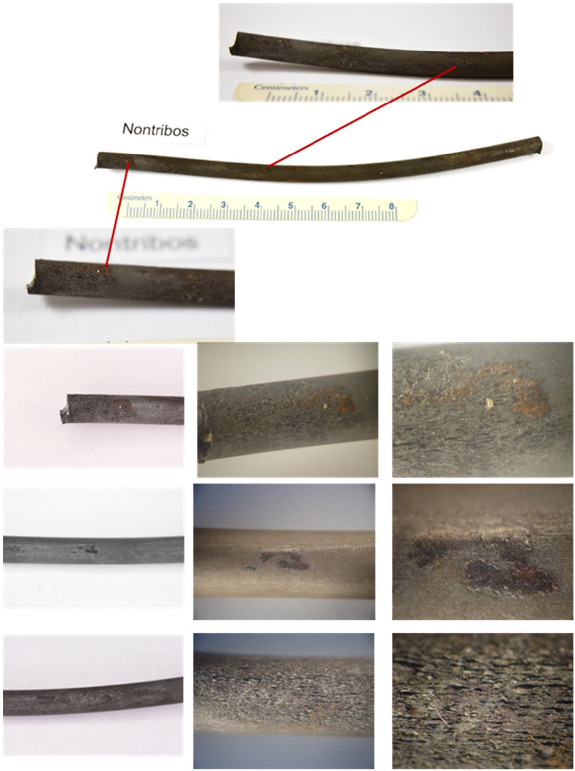
Figure 212. Single wire coated with Nontribos exposed outside semi-sheltered area
