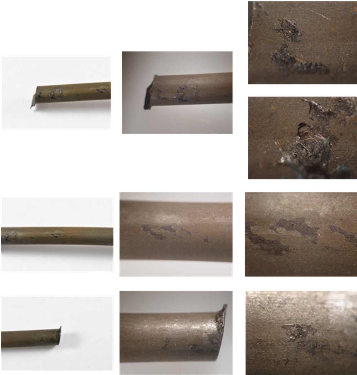
Figure 218. Single wire coated with Civetex exposed outdoors inside partially closed container.
