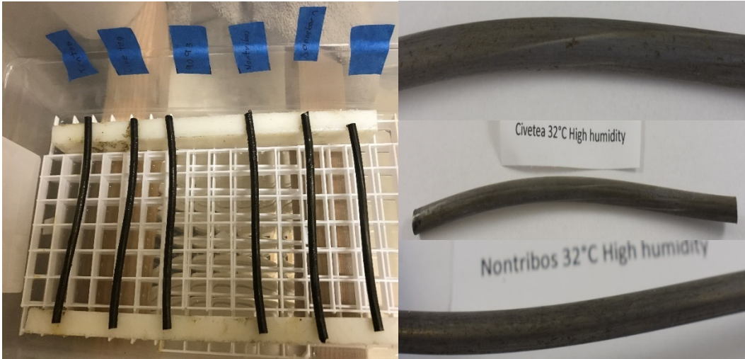
Figure 57. Wires coated at elevated temperature room.
