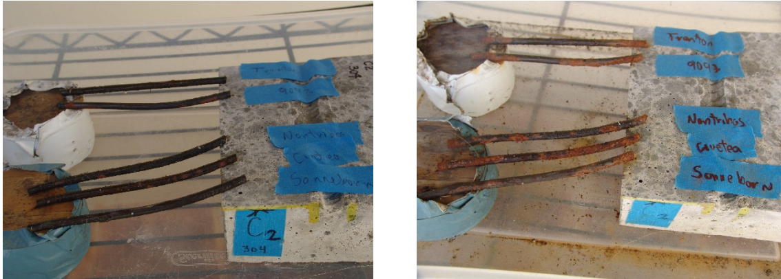
Figure 51. Wires coated with presence of rust. Left: July 28, 2016; Right: March 14, 2017.
