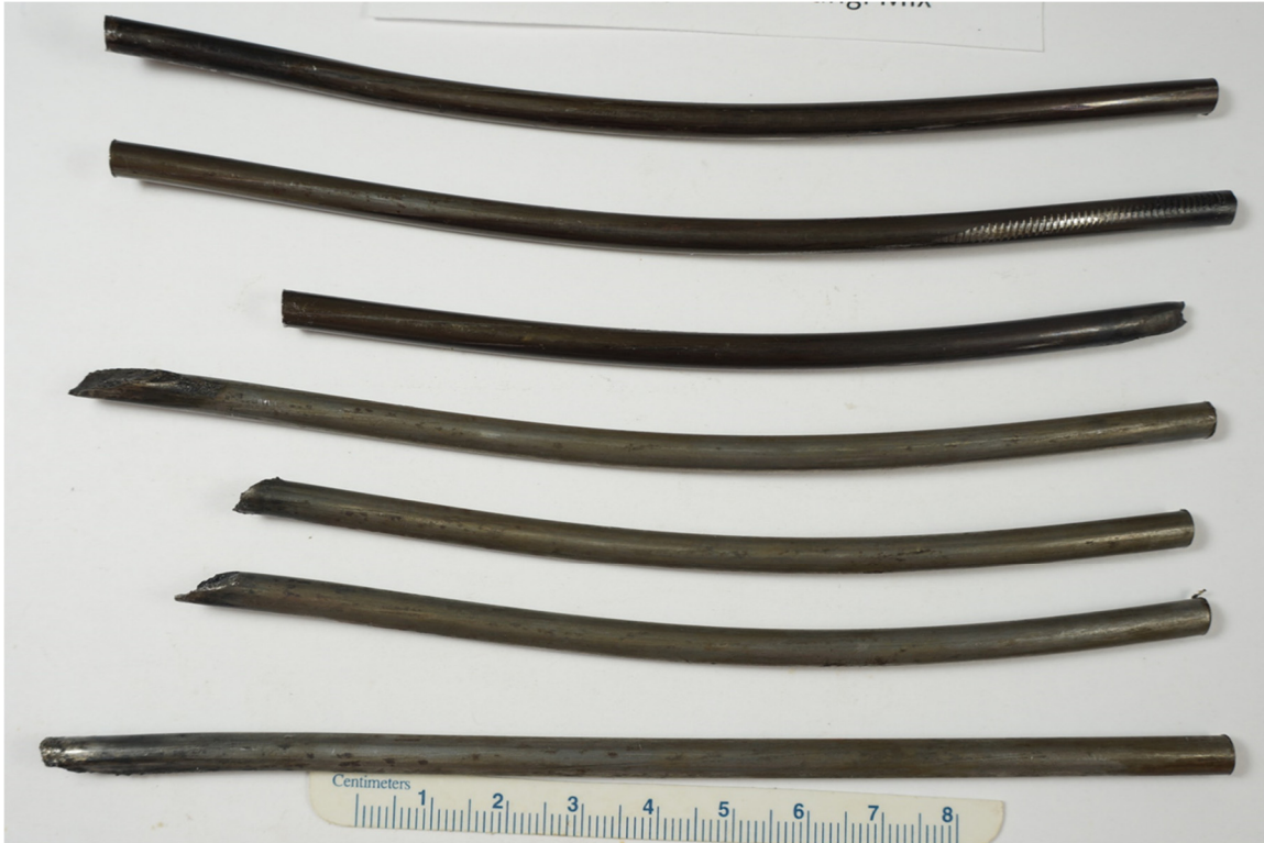
Figure 123. Section of Civetea coated strand, after cleaning (fungi mix).
