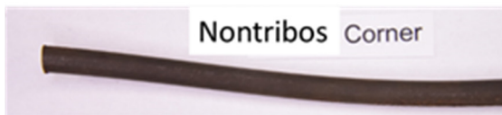
Figure 182. View of 1st strand segment, wire 5 after removing filler and cleaning
