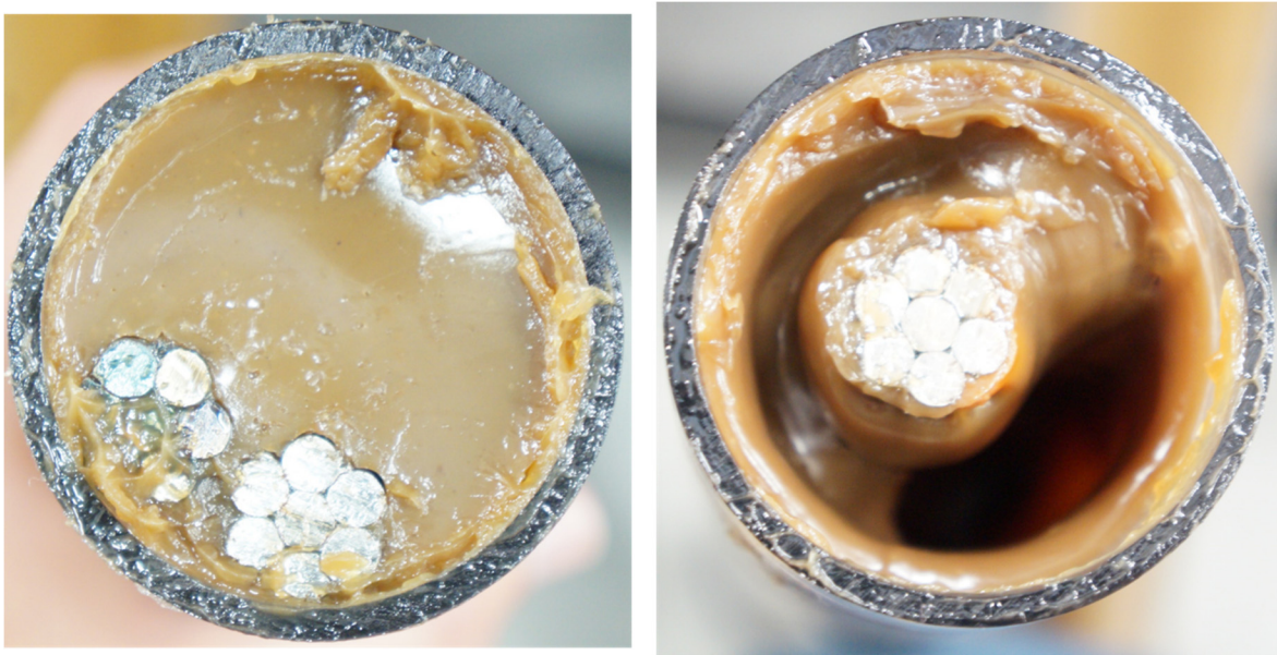
Figure 115. Two-foot long samples injected with Sonneborn filler (polycarbonate tubing) sprayed with fungi mix (June 2018).
