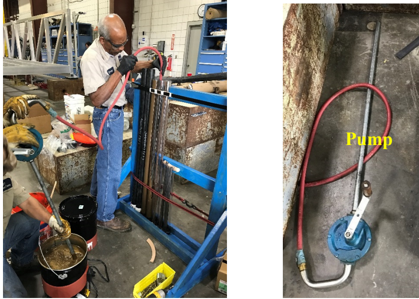
Figure 8. Flexible filler injection and a picture of the pump used.
