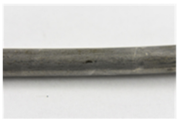
Figure 222. Single wire coated with Sonneborn at 20°C at high humidity
