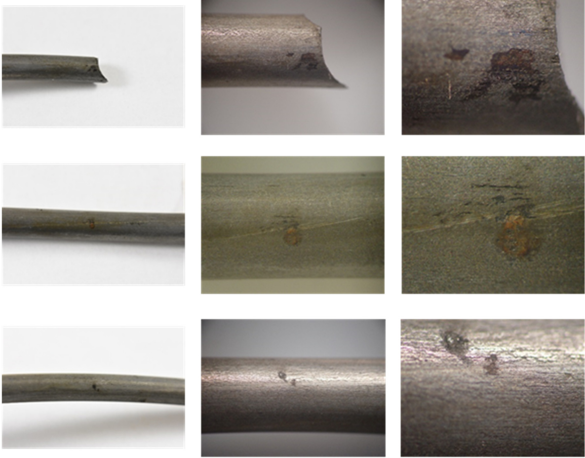
Figure 224. Single wire coated with Sanchem at 20°C at high humidity
