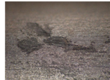
Figure 254. Coated with filler Trenton and sprayed with 1.5 milliliter of solution containing fungus PC (close-up).
