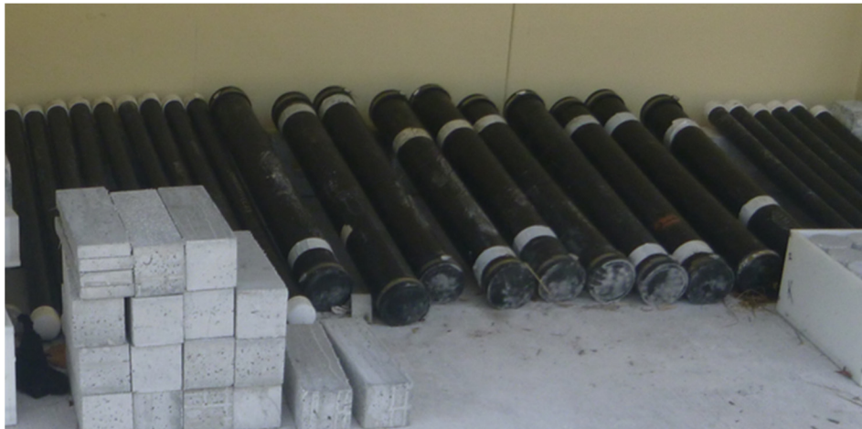
Figure 11. Four-inch and 2-inch diameter samples injected with flexible filler.
