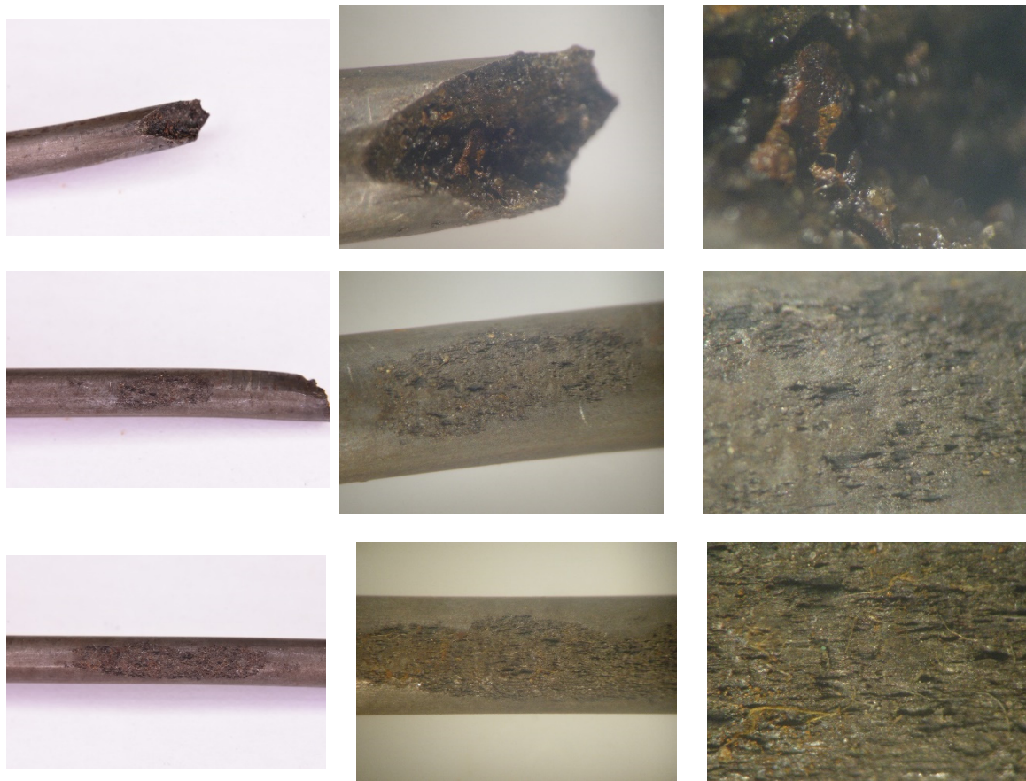
Figure 166. Close-up of wire 6 after removing filler and cleaning (view 2)
