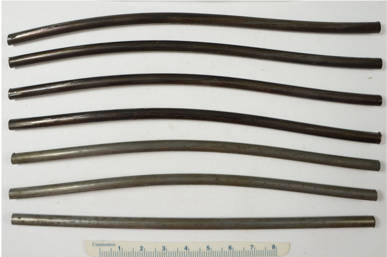
Figure 135. Section of Civetea coated strand, after cleaning (water)
