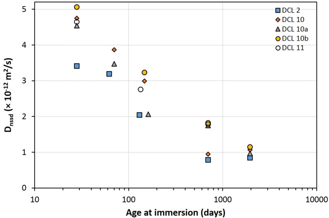
Figure 59. D_{nssd} vs. age at immersion measured on DC2, DC10, DC10a, DCL10b, and DC11 specimens
