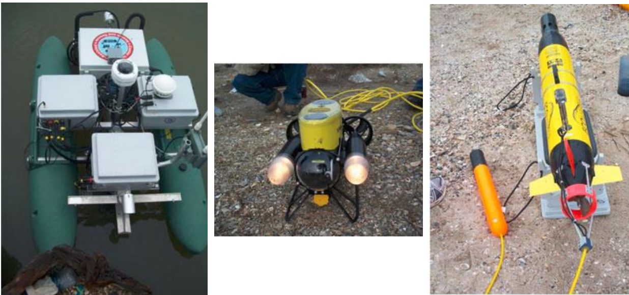
Figure 2: The USV (left), ROV (center) and AUV (right) tested by Murphy et al. [5].
