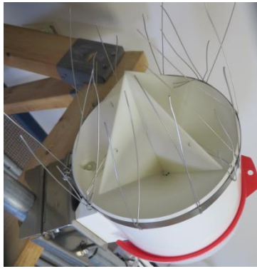
Figure 12: Rain gauge – top view of particle baffle and bird deterrence.
