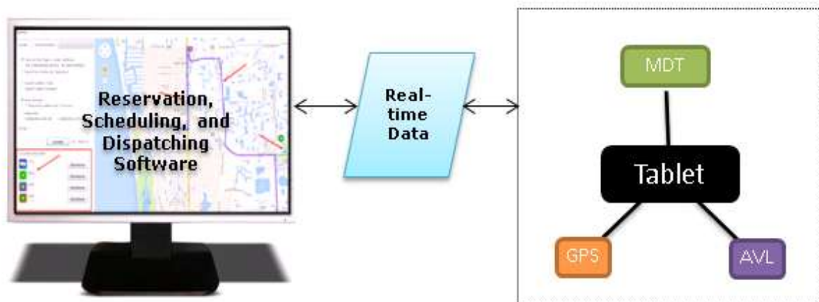
Figure 2-1: Tablet Serving as an MDT/AVL/GPS Unit Exchanges Real-Time Data with Dispatcher using the Reservation, Scheduling, and Dispatching Software
