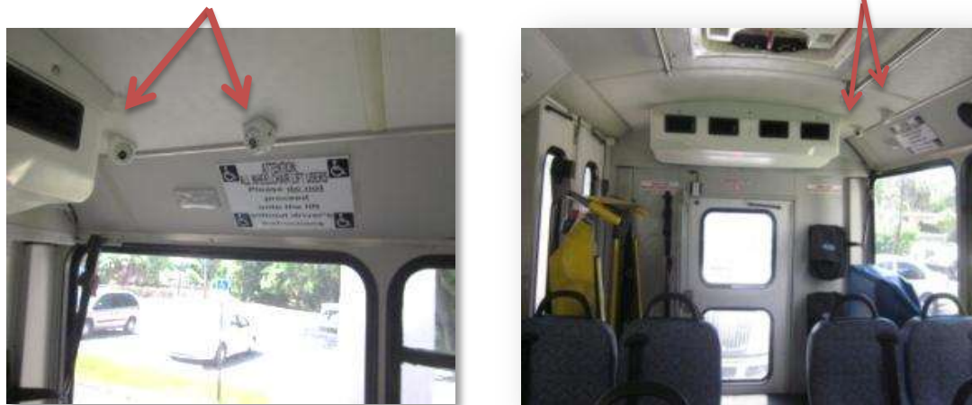
Figure 4-13: Vehicle Security Cameras Mounted Facing Wheelchair Lift
