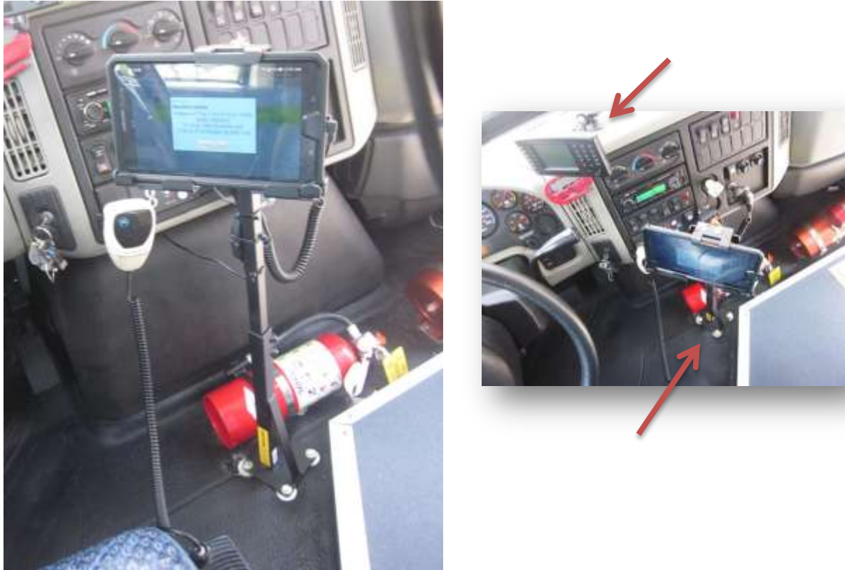
Figure 4-10: New MDT Tablet Mounted on Stand Secured to Floor of Vehicle and Old MDT Ranger Unit Mounted on the Dashboard
