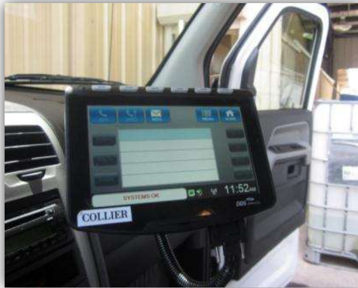
Figure 4-4: New M-Slate MDT from AVAIL on a Collier Area Transit Fleet Vehicle
