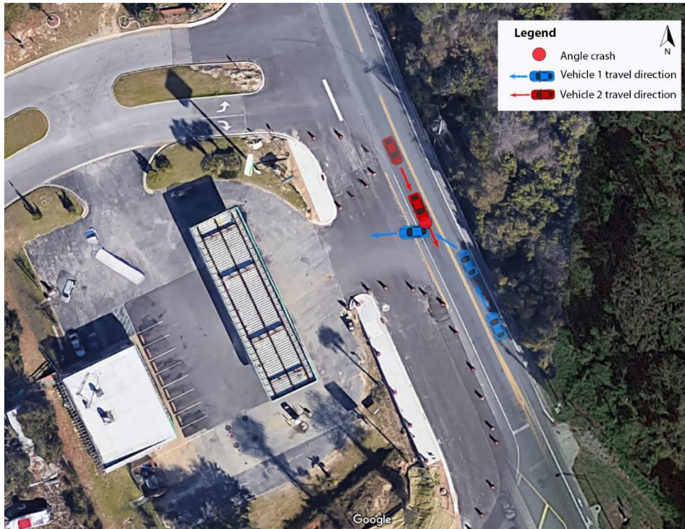
Figure 78. Left-turn crash at gas station north of interchange near ramps.
