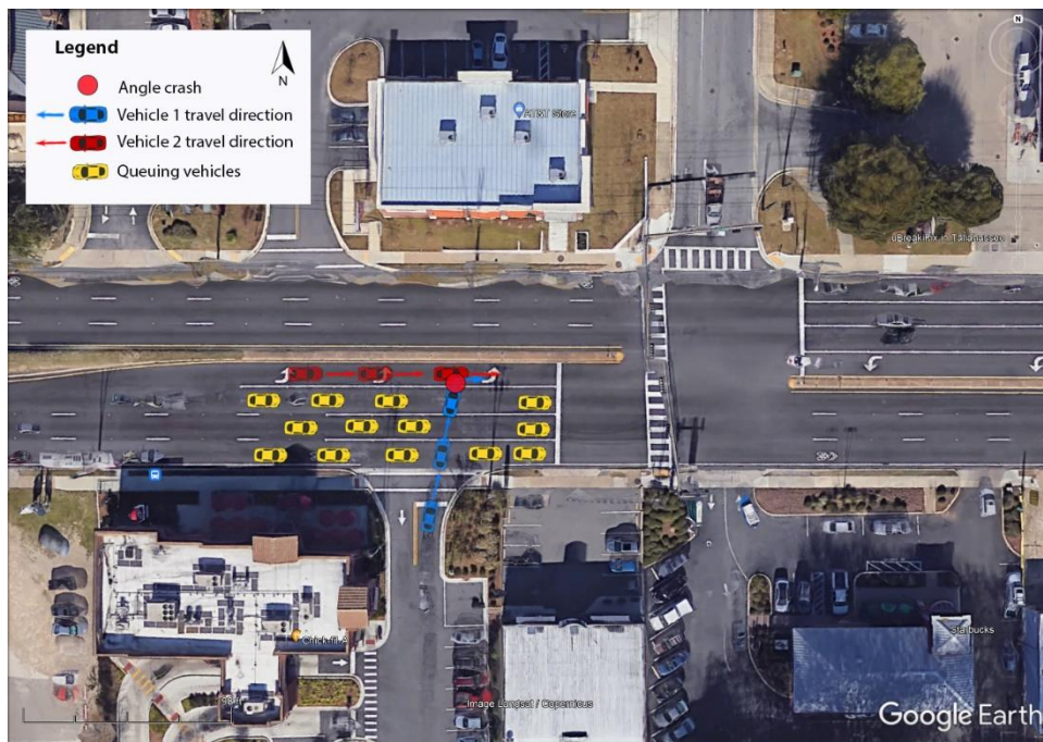
Figure 47. Angle crash on W. Tennessee Street.
