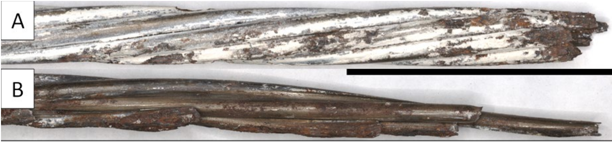
Figure 3-4. Example of (A) a strand with brittle fractures on all wires and (B) a strand with a combination of ductile and brittle fractured wires.
