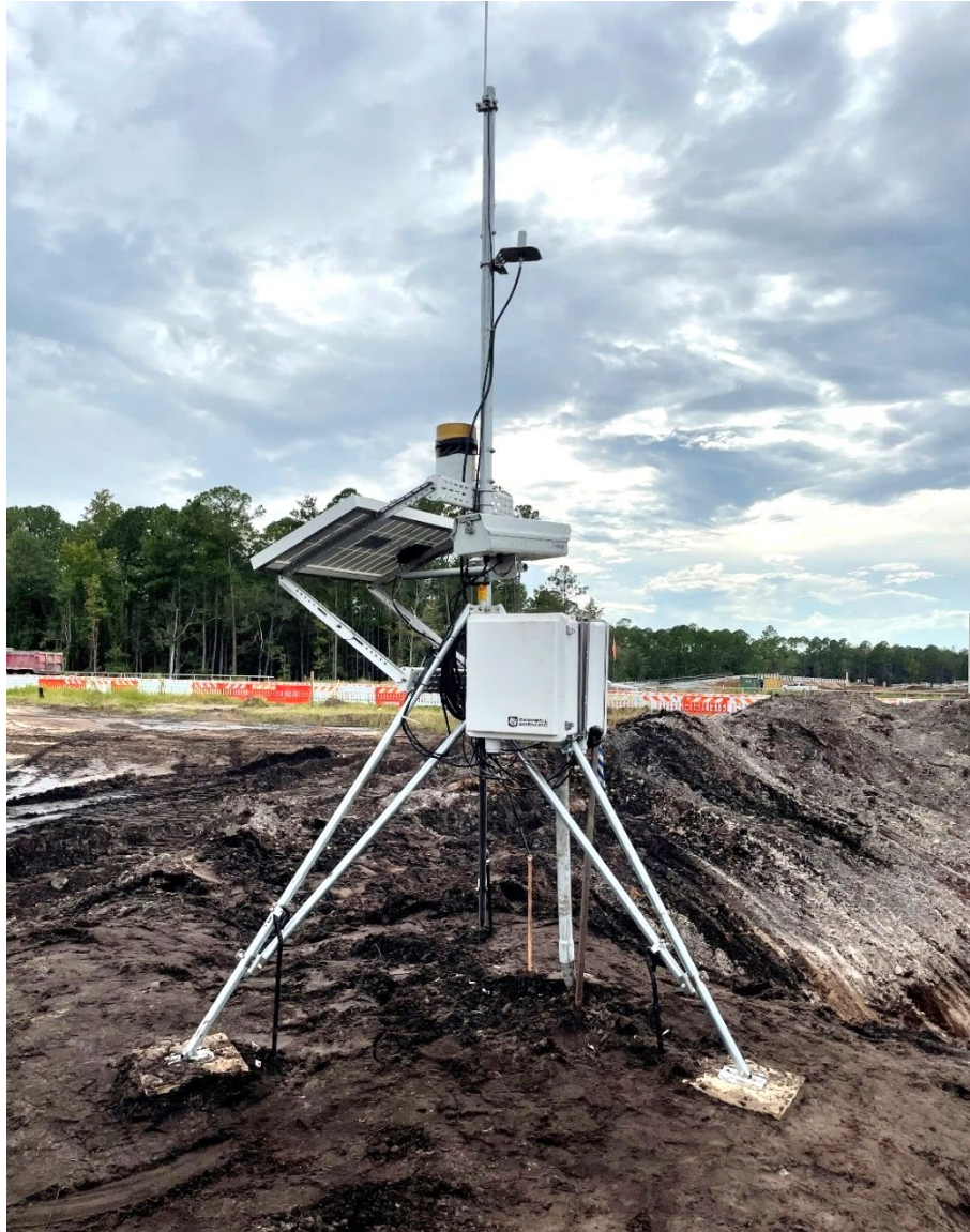
Figure 3.23 Solar-powered data collector complete with rain gauge, camera, cellular communications, and lightning rod.
