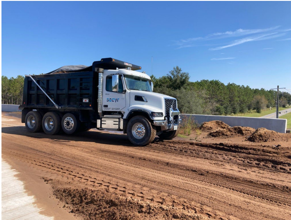
Figure 4.31 Seventy-kip loaded truck parked over test pile in end bent (Sandridge Rd).
