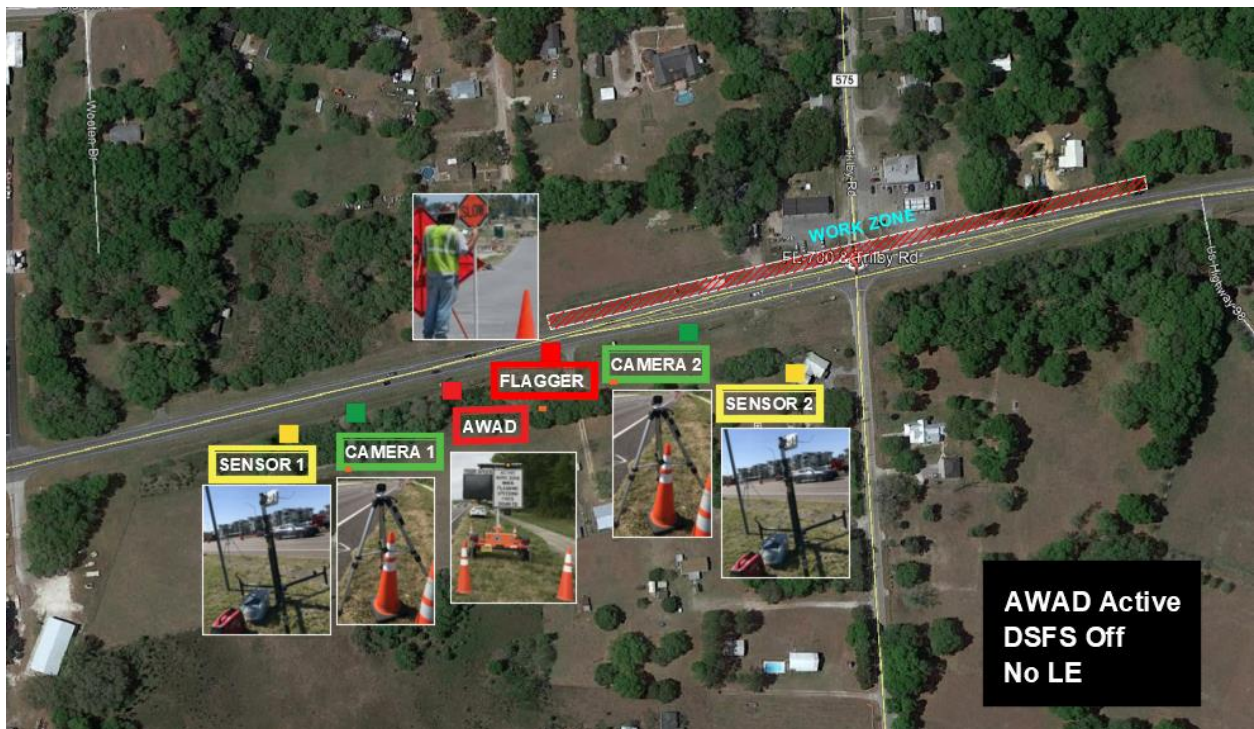
Figure 43. Deployment Stage of “After 1/AWAD” for Phase 4B1 at US-98 and Trilby Rd
