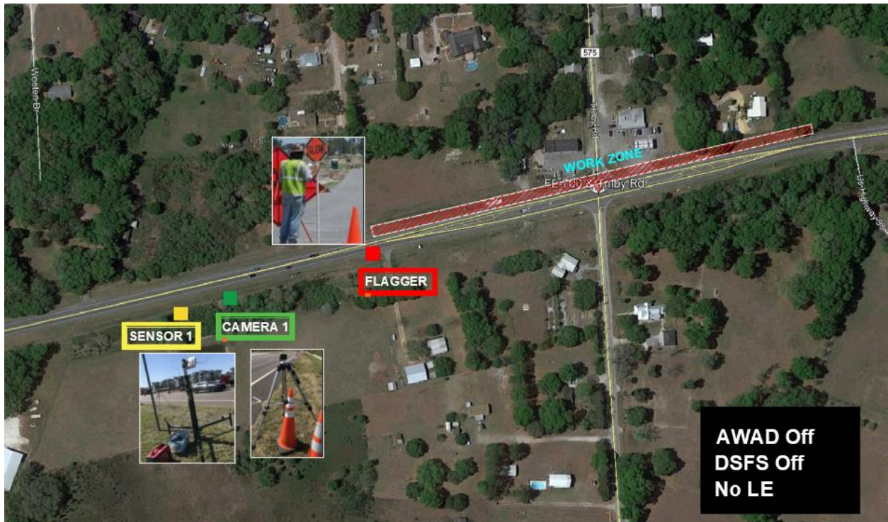
Figure 42. Deployment Stage of “Before/OFF” for Phase 4B1 at US-98 and Trilby Rd
