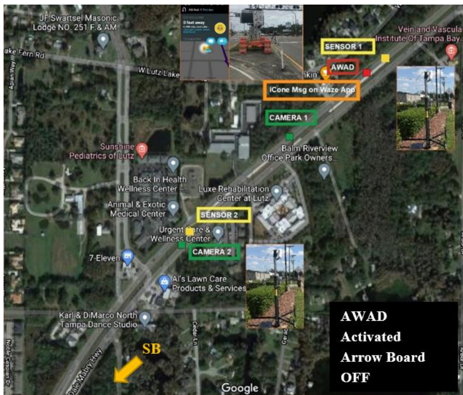
Figure 75. Layout of Data Collection for AWAD + iCone on N Dale Mabry Hwy
