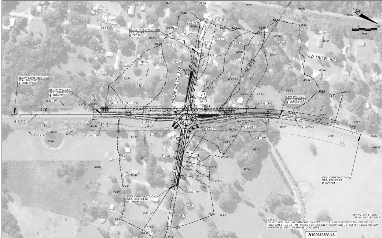
Figure 30. Construction Plan at US-98 and Trilby Rd
