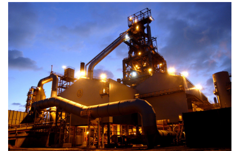
The enormous furnaces that convert iron ore into iron produce tons of slag as a byproduct.
