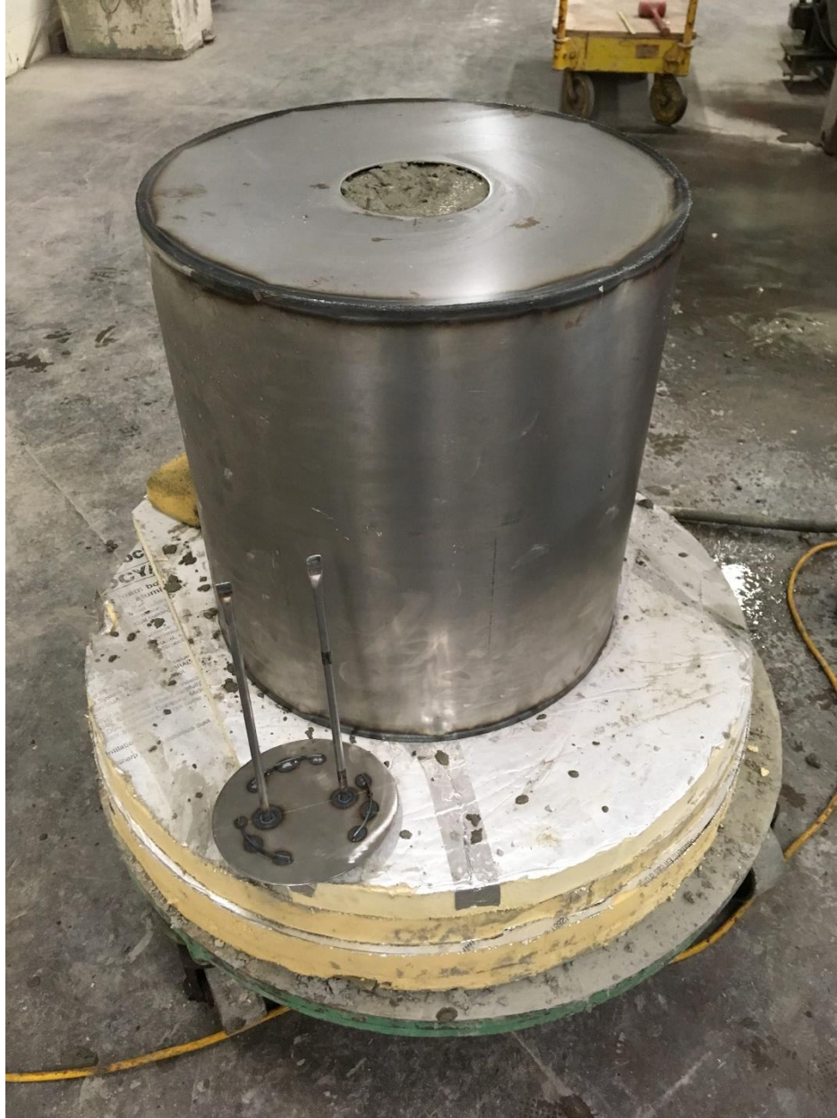
Figure 4-1: Concrete sample placed in steel canister set on insulated foam blocks and dolly
