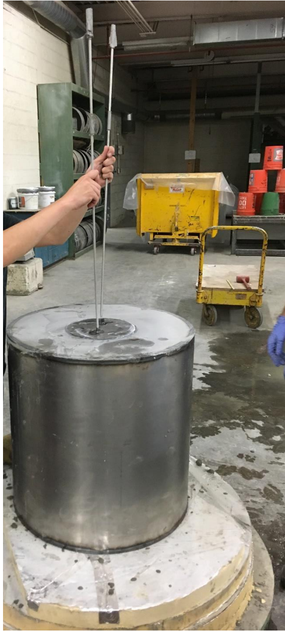
Figure 4-3: Thermocouple insertion into tubes on sample top
