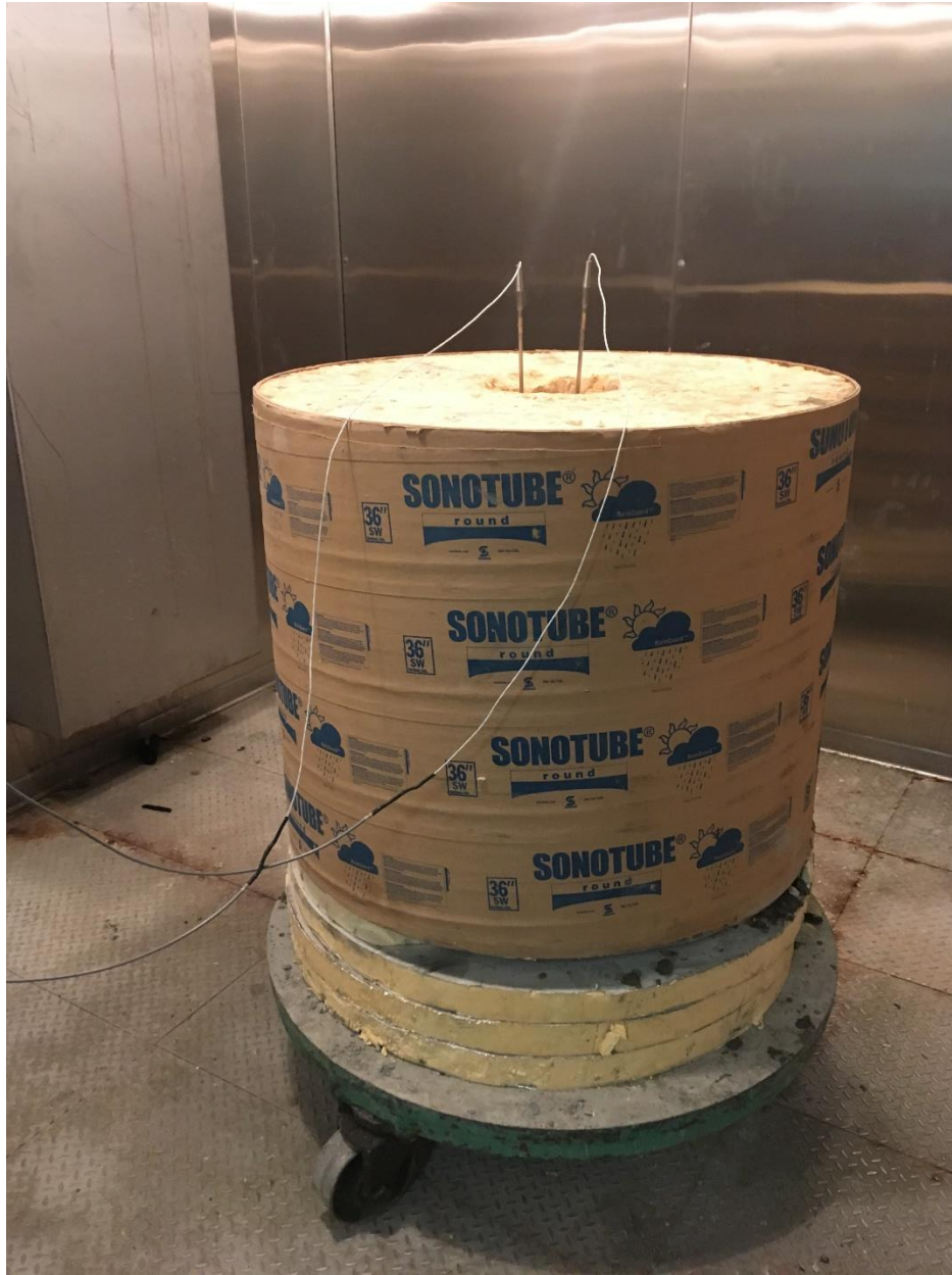
Figure 4-4: Concrete sample in adiabatic calorimeter
