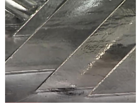
Sheet steel glistens as it is withdrawn from an 840°F bath of liquid zinc metal.
