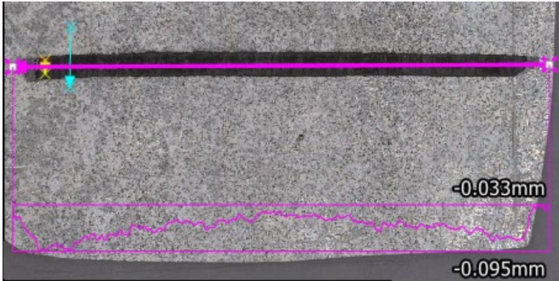
Figure 4.8. Aluminized steel etched crevice sample with a line scan using profilometric device with variations in depths in the etched defect before immersion, where the lowest depth is 33 \mu\text{m} and the maximum is 95 \mu\text{m} . The sample is called Sample (A) and immersed under the mild solution.
