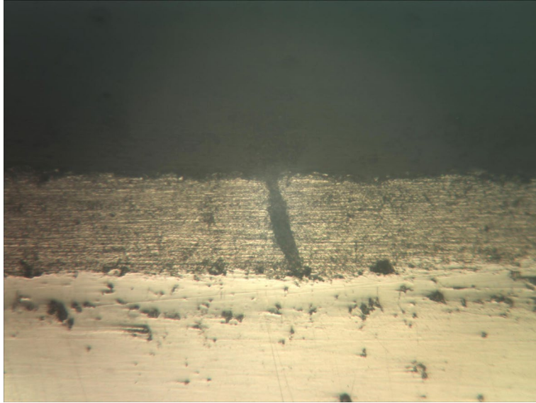
Figure 3.21. Metallographic image of coating break and shards in galvanized steel pipe from the Plant B.
